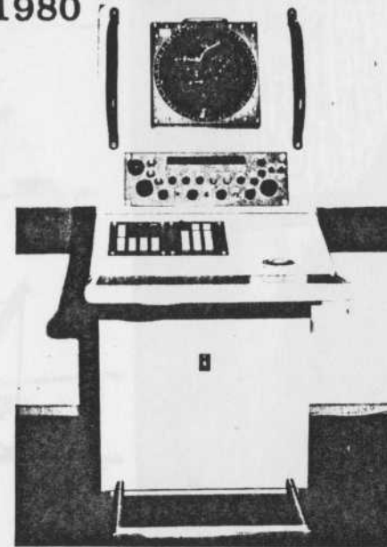
The Decca CANE console for HMS Speedy . The console features a Decca ED1200 viewing unit (top) and integral track management controls.
