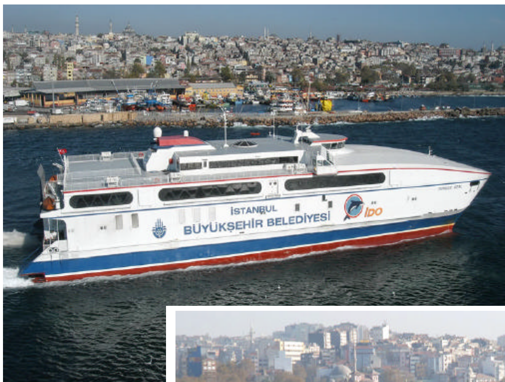
LEFT: Four vehicle/passenger catamarans built in Australia by Austal Ships are operated on longer routes across the Sea of Marmara. Auto Express 86 Turgut Özal was delivered in 1998 / IDO photo
