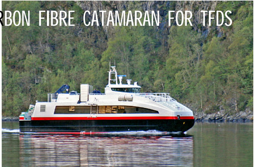
The 23m carbon fibre catamaran built by Brødrene Aa for TFDS, Kvænangen, on pre-delivery trials in the Hyefjord / BRØDRENE AA photo
