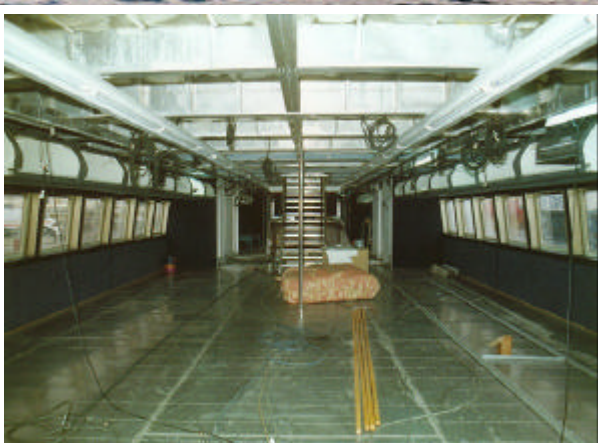
There is one big undivided downstairs saloon on the MEC 1 rather than two smaller ones – one advantage of the main engines being located aft on the MEC 1 rather than amidships as on all other Rodriquez hydrofoil designs
