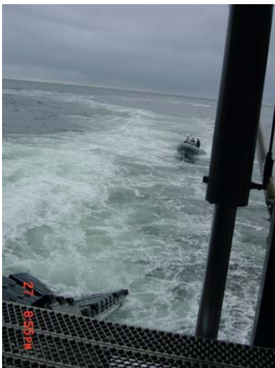
Figure 3. USV making an autonomous approach and alignment to Sea Fighter's stern ramp (foreground), April 2006.
