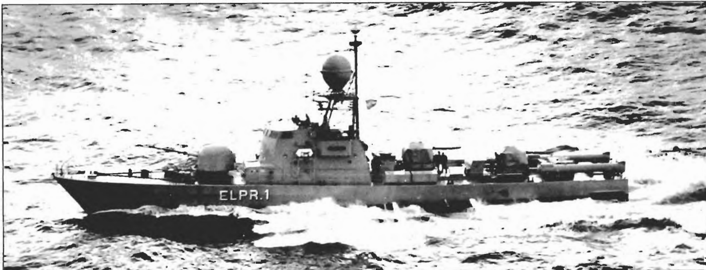
Above: The Argentinian Intrepida is armed with wire-guided torpedoes aft, a 40mm gun amidships and a 76mm gun forward.
