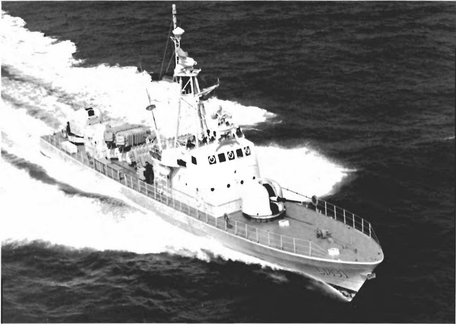
Above: The Ecuadorean FPB Quito , built by Lürssen, is armed with French Exocet missiles.
