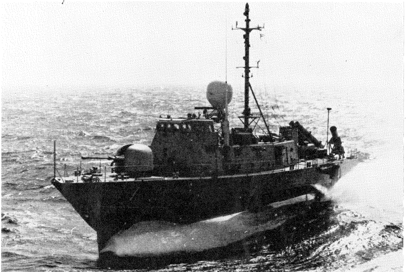
PEGASUS demonstrates her stable platform capability during a rough water test off Southern California. During testing, the PEGASUS successfully launched Harpoon missiles while foil-borne at over 40 knots.
