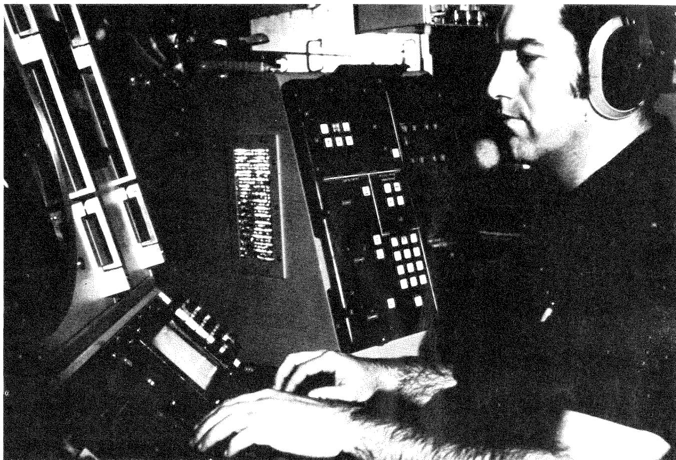
A PO1 operates the Mark 94 fire control system on board the PEGASUS. The system embodies a combined fire control and search antenna system mounted on a single stabilized platform and enclosed in a fiberglass radome.
