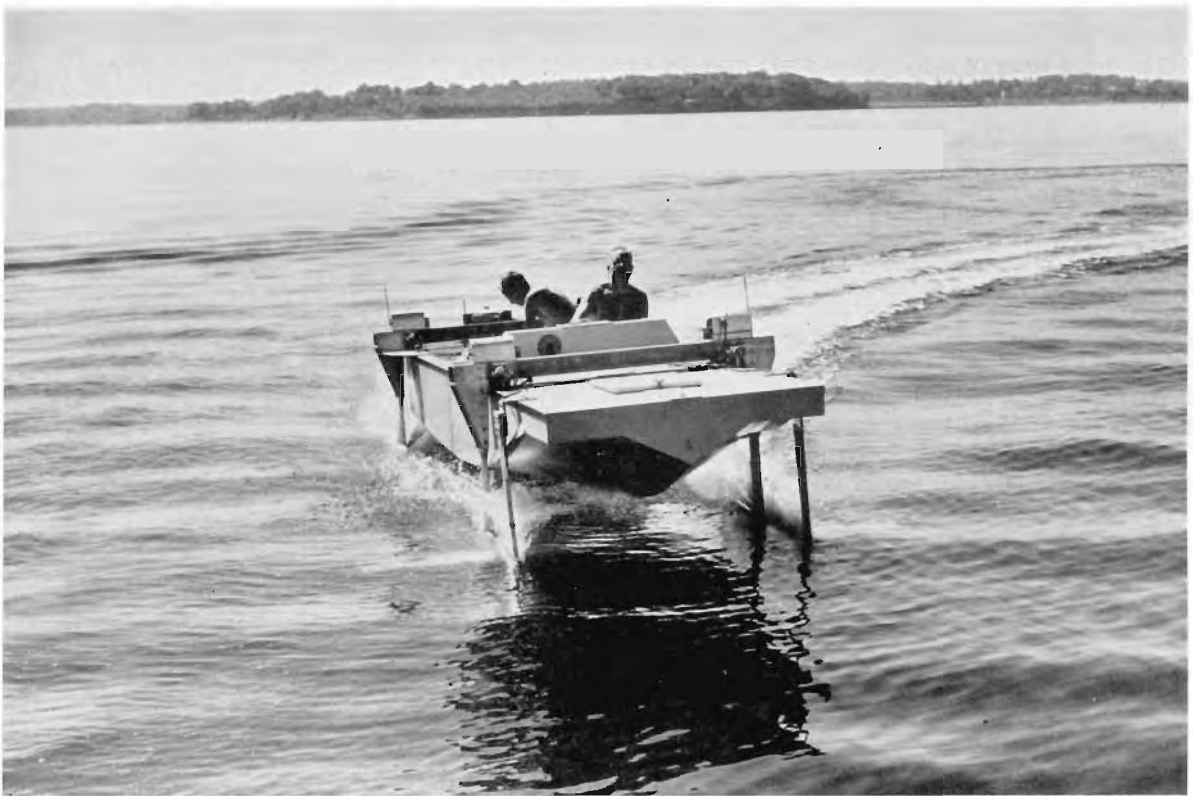
FIG. 10.—AUTOMATIC INCIDENCE CONTROL STABILIZATION ON A 20-FOOT UNITED STATES NAVY TEST CRAFT
