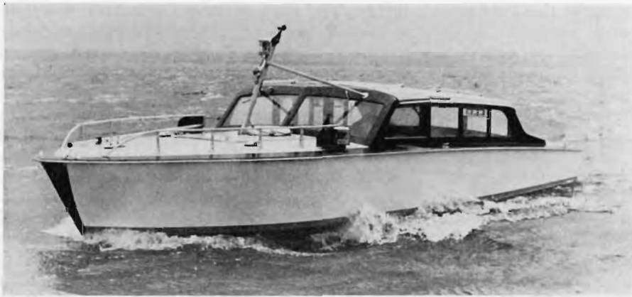
FIG. 20.—HYDROFOIL-EQUIPPED CRUISER IN CONVENTIONAL OPERATION
