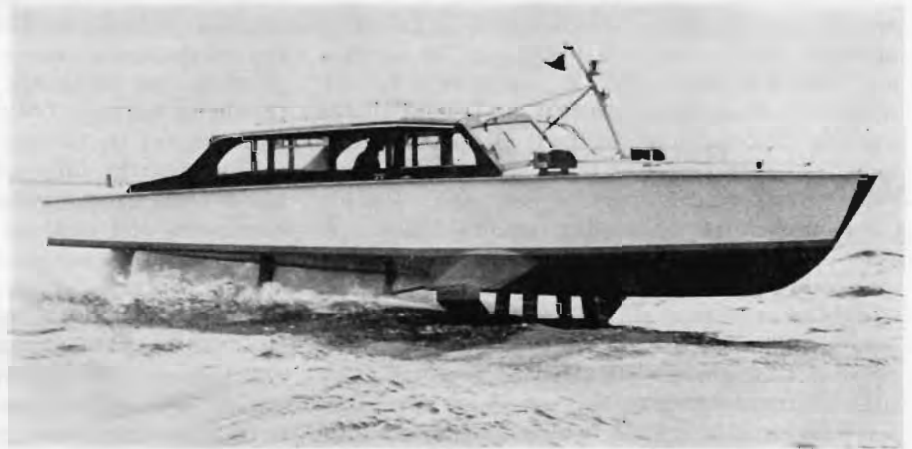
FIG. 21.—CRUISER RUNNING AT SPEED, SHOWING HYDROFOILS IN ACTION
