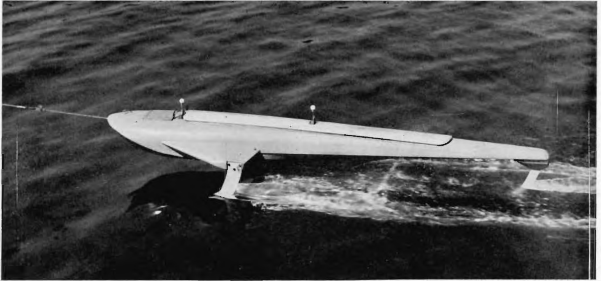
FIG. 8.—TWELVE-FOOT OPEN WATER MODEL FITTED WITH BIPLANE V-FOILS
