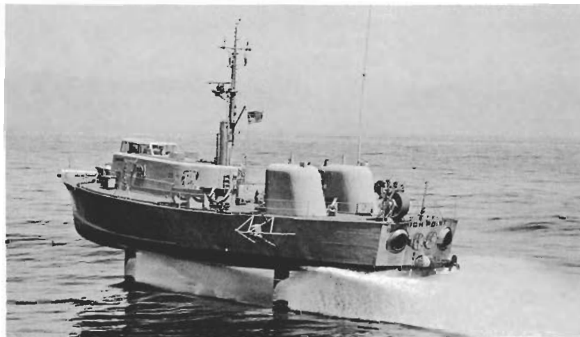
Hydrofoils, as well as air cushion vehicles, hold promise for naval applications. Above the HIGH POINT, the Navy's first operational hydrofoil, is shown during tests off the Washington State coast. The 110-ton craft was built for the Bureau of Ships by the Boeing Company. It is designed to exceed 50 miles an hour.
