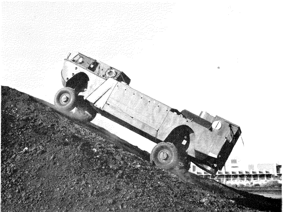
Land power for the LVHX2 is transmitted from the Solar T 1,000-S27 gas turbine to the wheels through an Allison TX 365-2 six speed transmission. The craft is able to negotiate 60% slopes in forward or reverse and can operate on 30% side slopes
