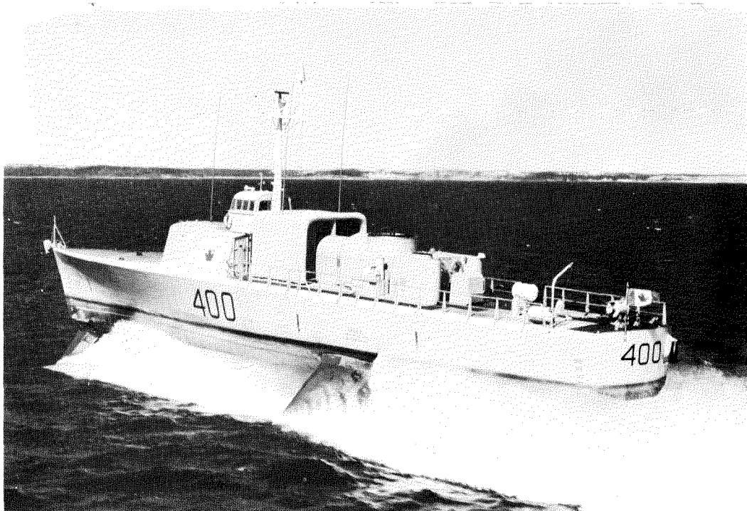
The De Havilland FHE-400 HMCS Bras D'Or—photographed during her first foilborne run off the Halifax coast on April 9th 1969
