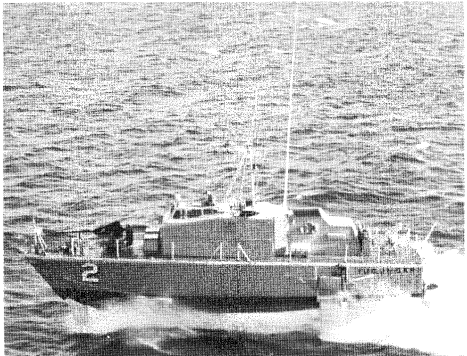
Boeing PGH-2 Tucumcari waterjet-propelled hydrofoil gunboat, designed for high-speed, heavy weather, offensive and defensive operations. Main armament comprises a 40 mm rapid-fire cannon forward of the bridge and an 81 mm mortar aft. Manually-operated twin .50 machine guns on ring mountings are sited aft of the pilothouse on each side of the bridge superstructure. Foilborne cruising speed is in excess of 40 knots
