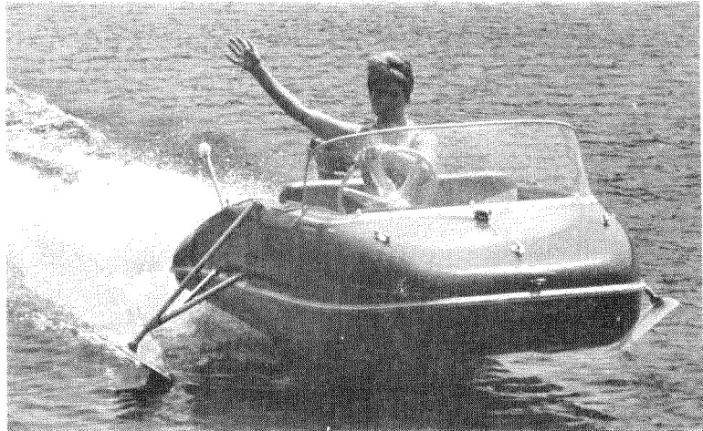
Water Spyder 2-B, a two seat, fibreglass-hulled hydrofoil pleasure craft powered by a 20-30 hp long-shaft outboard motor. The retractable VV main foil system carries 98% of the total load
