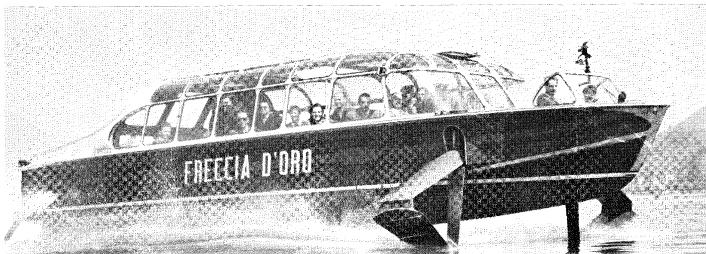
The Supramar PT10 (one 1,100 hp MB 820 Db diesel), a 32 passenger hydrofoil for sightseeing or commuter services on inland waters and protected bays
