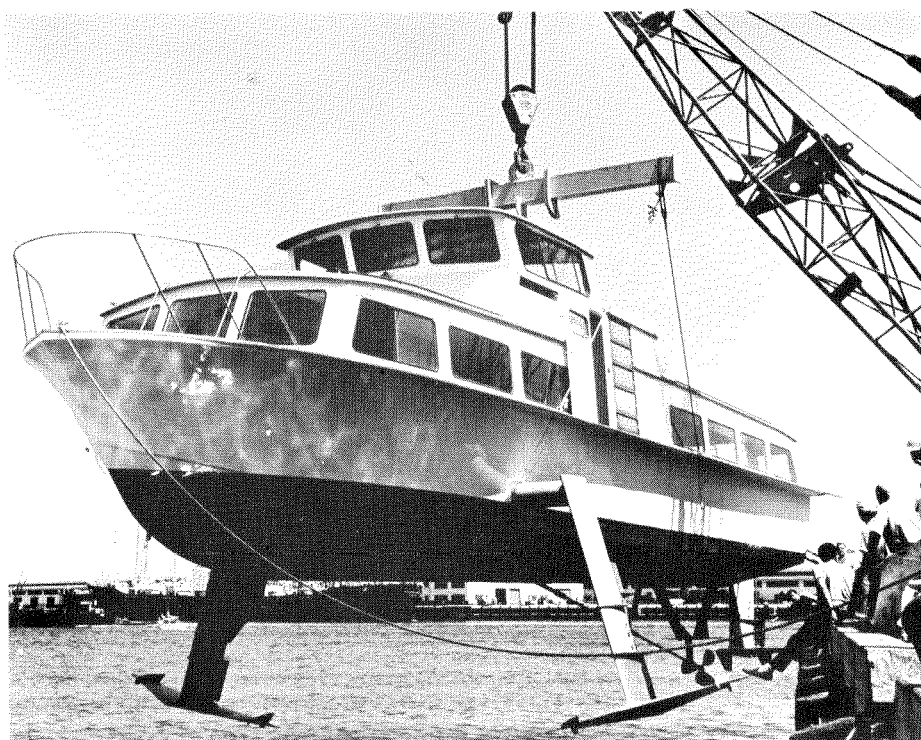
Flying Cloud, showing the mechanically-operated foil system. Hinged vertical control flaps on the trailing edges of the forward struts automatically deflect the foil flaps to maintain the craft at a stable inflight attitude in all sea states
