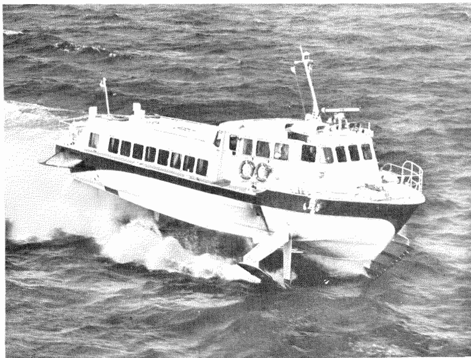
A feature of the PT 20B is the location of the bridge in the foreship to provide improved vision. The standard version seats sixteen passengers in the forward cabin above the engine room and fifty-four in the main compartment. Powered by an MB 820 Db diesel rated at 1,100 hp continuous, the craft cruises at 34 knots (63 km/h)
