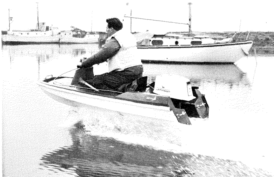
Hi-Foil 2, a two-seat, fibreglass-hulled sports hydrofoil. The bow foil is mounted at the base of a handle-bar equipped steering head. Top speed is 25-35 mph according to the outboard motor installed
