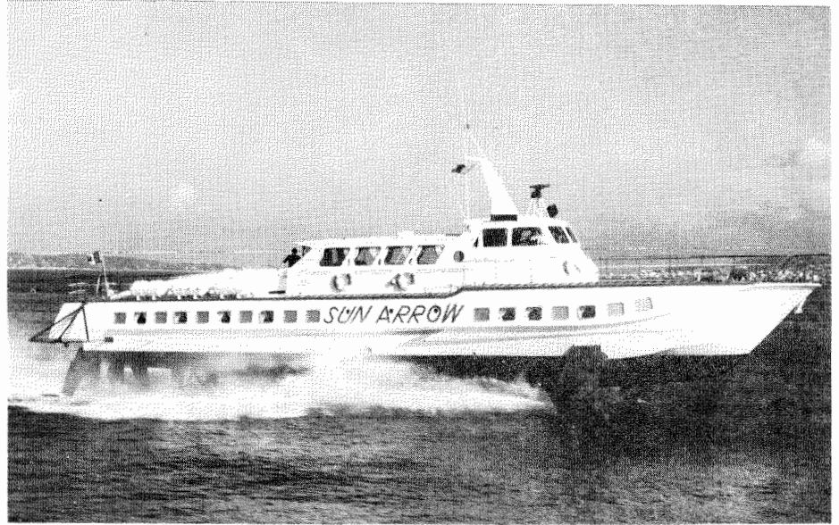
A Rodriguez-built PT 50, a 63-ton hydrofoil with a cruising speed of 34 knots and seating up to 140 passengers
