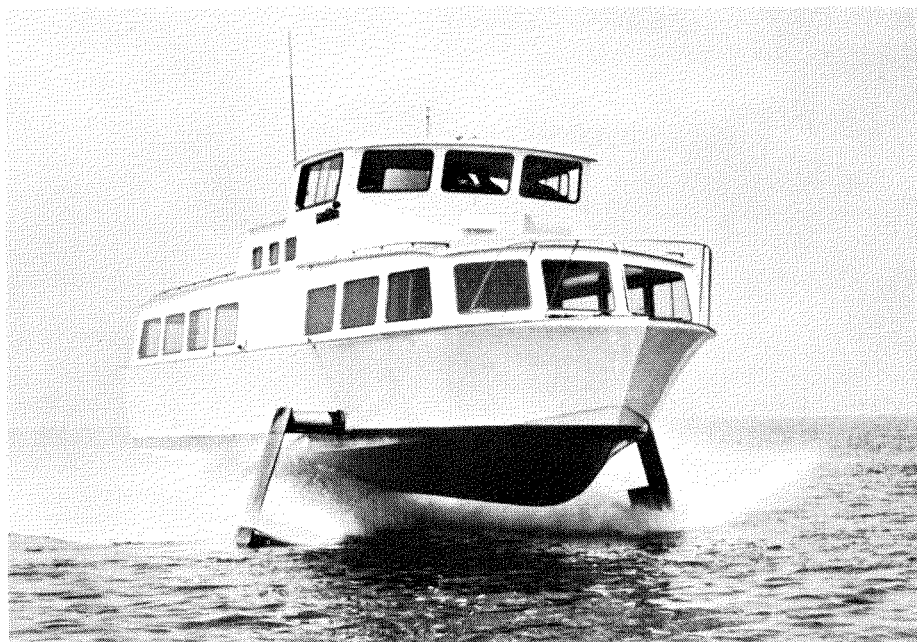
Flying Cloud, designed by Atlantic Hydrofoils Inc, and built by Teledyne Inc of Gardena, California, is powered by a 1,100 hp Solar Saturn gas turbine and has a service speed of 32 knots
