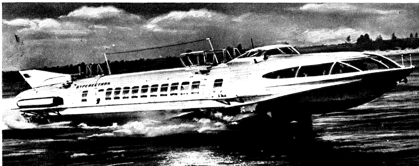
The gas-turbine powered Burevestnik, latest in the family of Soviet hydrofoils inspired by the Meteor. The craft cruises at 60 knots and opened a service between Gorky and Kuibyshev in April 1968
