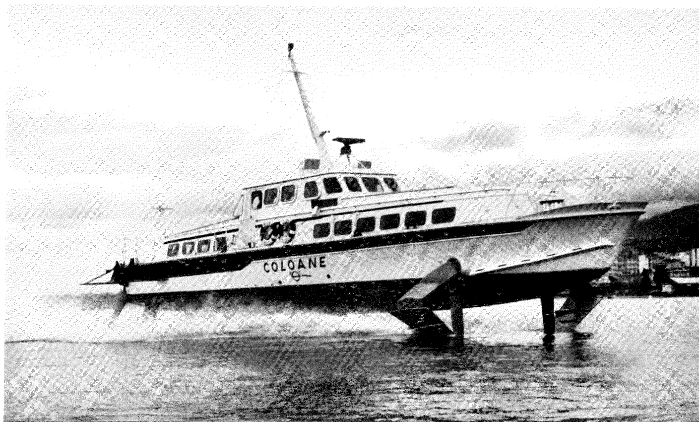
The PT 20, a 72-seat hydrofoil for coastal services, has been in continuous production since 1955. Nearly 70 are in service in 21 countries
