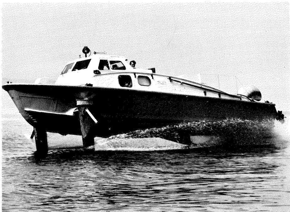
A modified ST 3 is being employed by Supramar as a research craft for the Schertel-Supramar fully-submerged, air-stabilised foil system. Powered by a 1,000 hp GE LM100 gas-turbine, the craft has reached speeds in excess of 54 knots during tests in the Mediterranean
