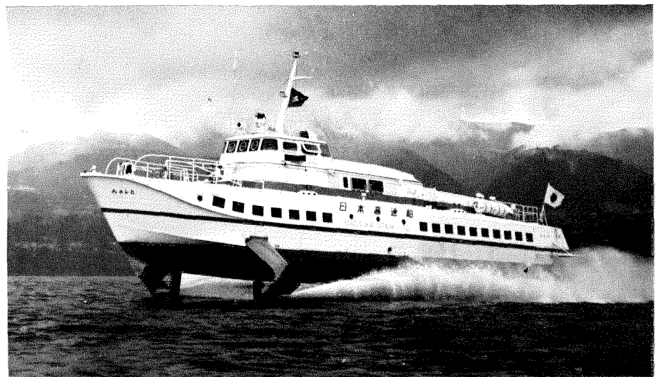
Wakashio, a Hitachi PT 50 (two 1,350 hp MB 820 Db diesels) which has been operated between Enosima and Atami by Nihon Kosokusen since 1963.
