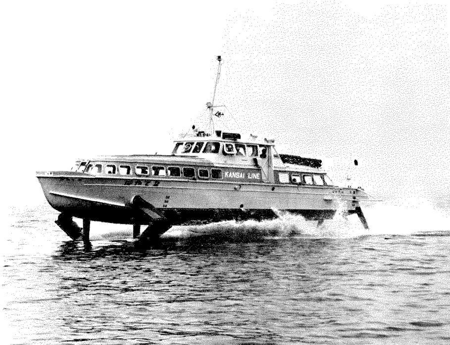
Figure 1. The PT 20, first passenger carrying hydrofoil to be approved by classification societies for coastal services
