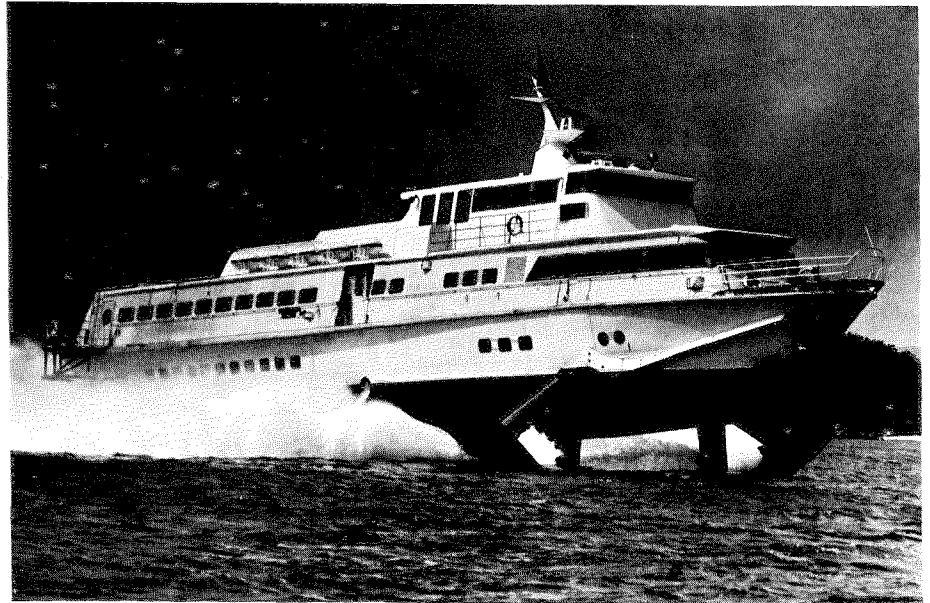
The first Supramar PT 150, a 150-ton 37-knot passenger/car ferry built by Westermoen Hydrofoil A/S, Mandal, Norway, for Gothenburg-Fredrikshavn-Line. The craft was delivered in June 1968 and is now operating between Sweden and Denmark, calling at Gothenburg, Aalborg and Fredrikshavn
