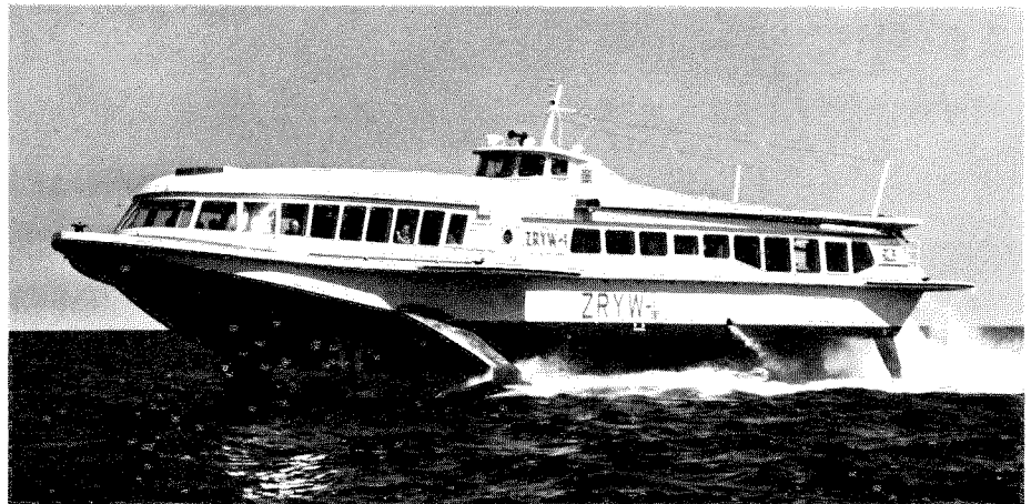
The ZRYW-1 (one Soviet-built M-50F 4 diesel) averages more than 39 knots on scheduled services between Szczecin and Swinoujscie, a distance of 36 nautical miles (67 km)
