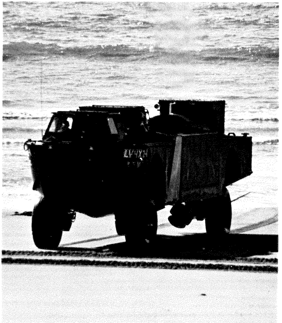
Land power for the LVHX2 is transmitted from the 1,100 hp Solar T 1,000-S27 gas turbine to the wheels through an Allison TX 365-2 six speed transmission and non-slip differentials
