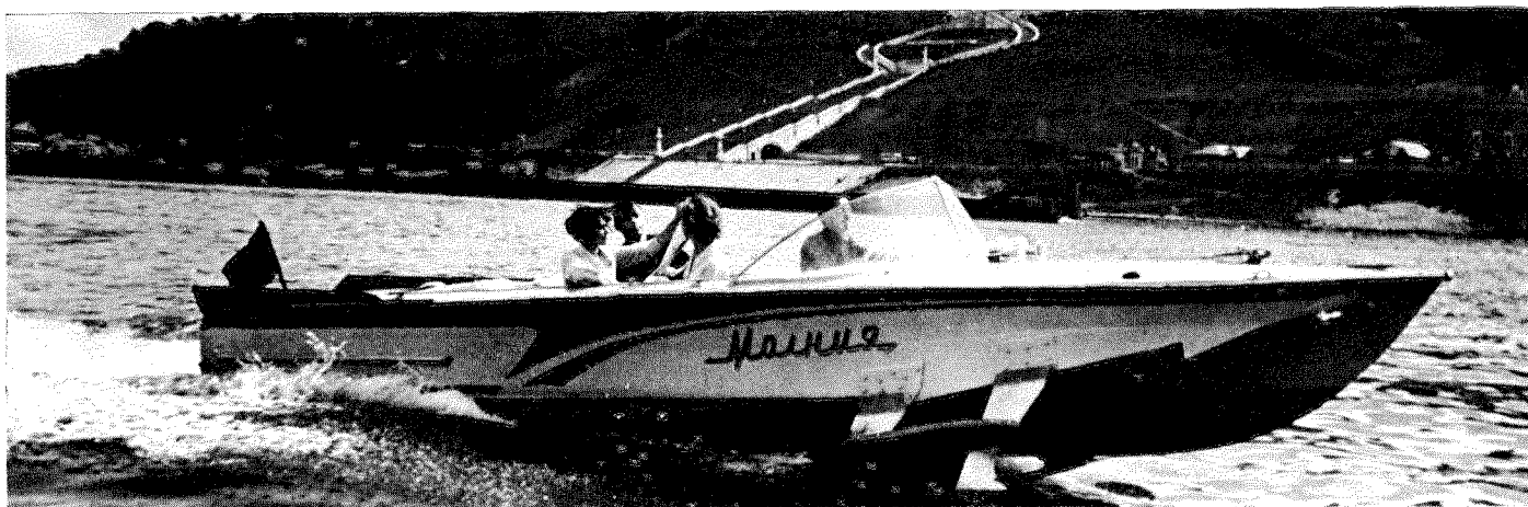
MOLNIA, a popular six-seat runabout, is said to be navigable in protected off-shore waters up to two miles from land, and ideal for water-taxi services and joy-ride operators. Top speed is 32 knots
