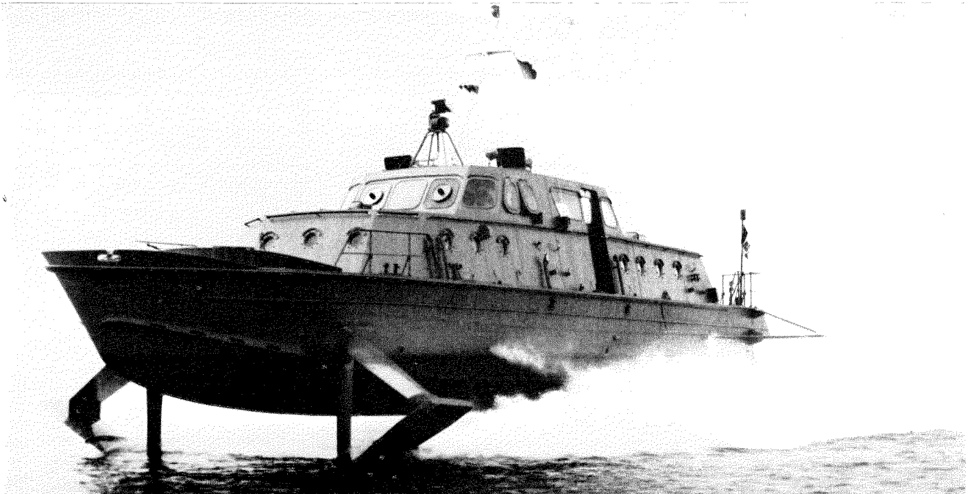
A Rodriquez PAT 20 fast patrol hydrofoil under test off Messina. Two are employed by the Philippine Navy on contraband patrol and coastguard duties.
