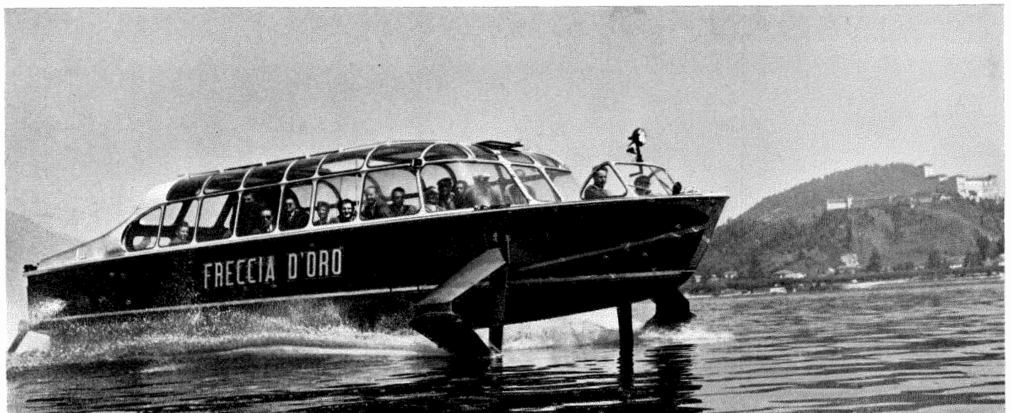
The Supramar PT10 (one 1,100 hp MB 820 Db diesel), a 32 passenger hydrofoil for sightseeing or commuter services on inland waters and protected bays
