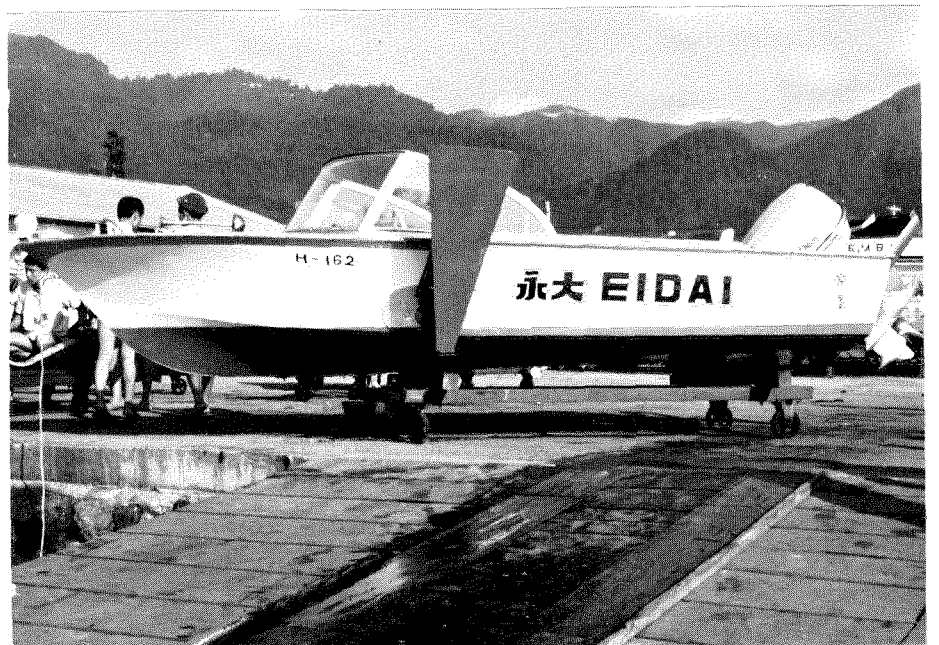
YODO-16, a 5-6 seat, 34 knot sports hydrofoil built by Eidai Sangyo Co. and fitted with Hitachi-Supramar retractable AT-foils
