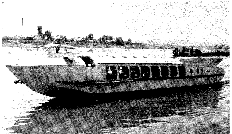
Byelorus, a 30-45 seat hydrofoil developed for fast ferry service on shallow waters, seen on the Irtysch river. Powered by a 735 hp M-50 diesel the craft cruises at 60 km/h
