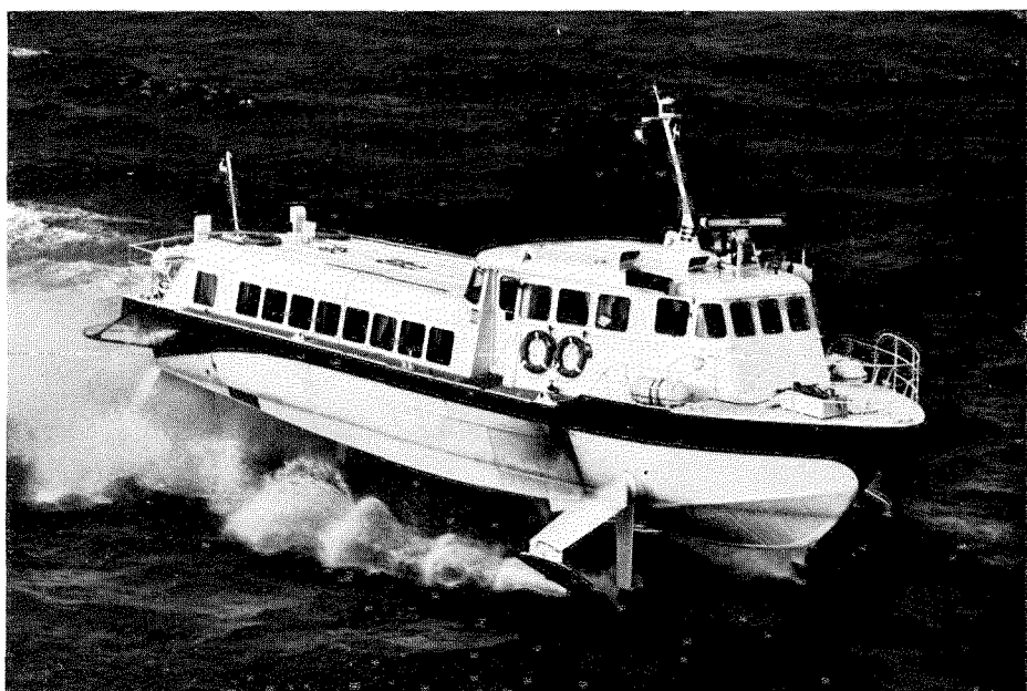
Bridge of the PT 20B is located in the foreship to provide improved vision. Sixteen passengers are accommodated in the forward cabin above the engine room and fifty-four in the main cabin. Powered by an MB 820Db diesel rated at 1,100 hp continuous, the craft cruises at 34 knots (63 km/h)
