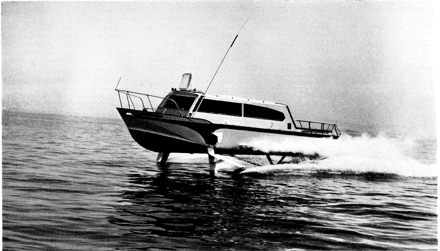
Seating 12 passengers and capable of speeds in excess of 45 mph (72 km/h), the FMC L312G is a 30 ft (9.14 m) test and demonstration craft. It was used to obtain data for the design of the 48-passenger L548D
