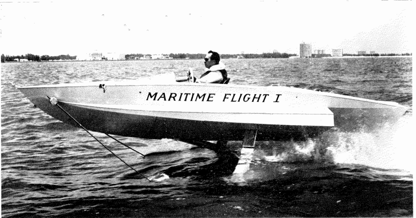
The Wynne-Gill Maritime Flight I 4-seat sports hydrofoil prototype. The craft has a fully submerged foil system with mechanical wave sensors operating trailing edge flaps to maintain the foils at the required depth.
