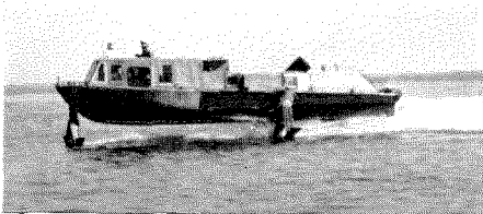
Mitsubishi's waterjet research craft. The waterjet is generated by a double-section centrifugal pump powered through a reduction gearbox by a General Electric T58
