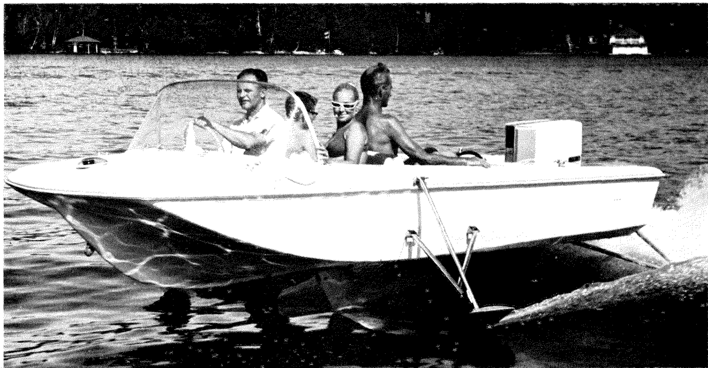
Water Spyder 6-A is a six-seat hydrofoil. The main foil, trim-tab support and engine fold upward so the craft can be floated on and off a trailer
