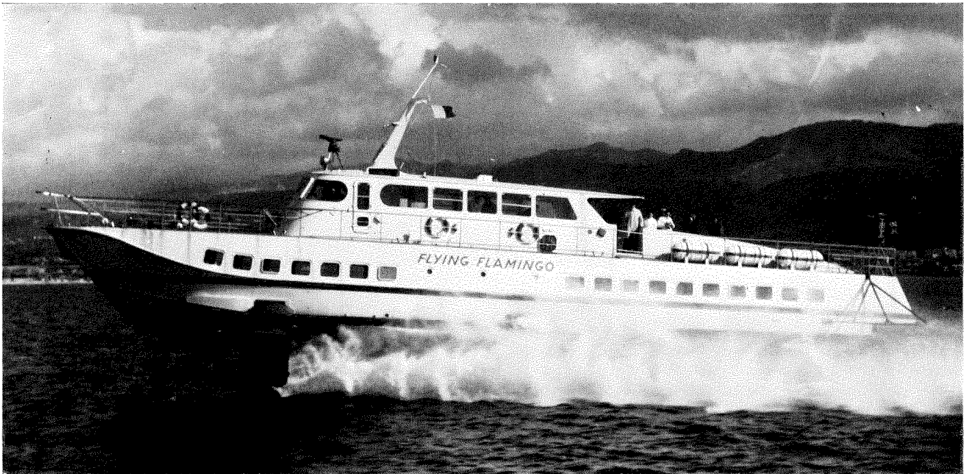
Flying Flamingo, a Rodriguez-built 125-seat PT 50/S, operated by the Hong Kong Macao Hydrofoil Company. Cruising speed is 34 knots.
