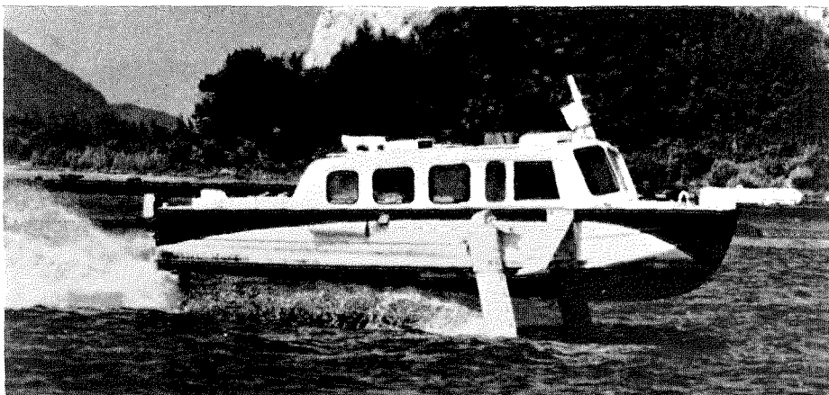
The Mitsubishi M3 submerged foil test craft
