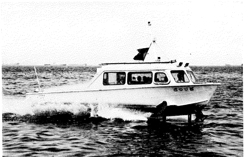
The PT 4 (one Chrysler M413D) is designed for services on lakes and rivers. As a sightseeing craft it will seat 12 passengers.
