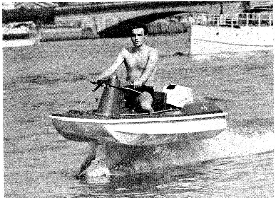
Hi-Foil 2, a two-seat, fibreglass-hulled sports hydrofoil. Steering is similar to that of a motorcycle. Top speed is 25-35 mph according to the outboard motor installed
