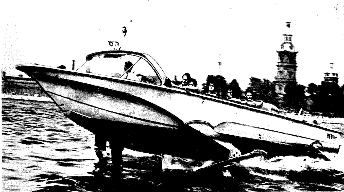
The Nevka is available as a 12-14 seat open cockpit water-taxi, cabin cruiser or sightseeing craft with a transparent roof. A 250 hp diesel provides a speed of 60 km/h
