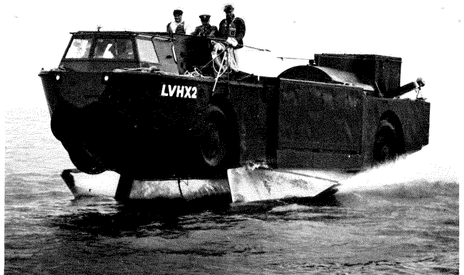
The LVHX2, an amphibious hydrofoil landing craft built by FMC for the US marines. The craft operates at 35 knots to the surf zone, negotiates shallow areas as a displacement craft, then moves quickly inland on four sand-type tyres
