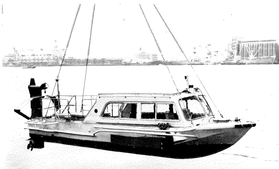
The IHF-3's foil system is retracted hydraulically. The forward foil assembly is folded and swings aft above the waterline. The complete aft foil assembly is rotated through 180° bringing the hullborne propeller into position.
