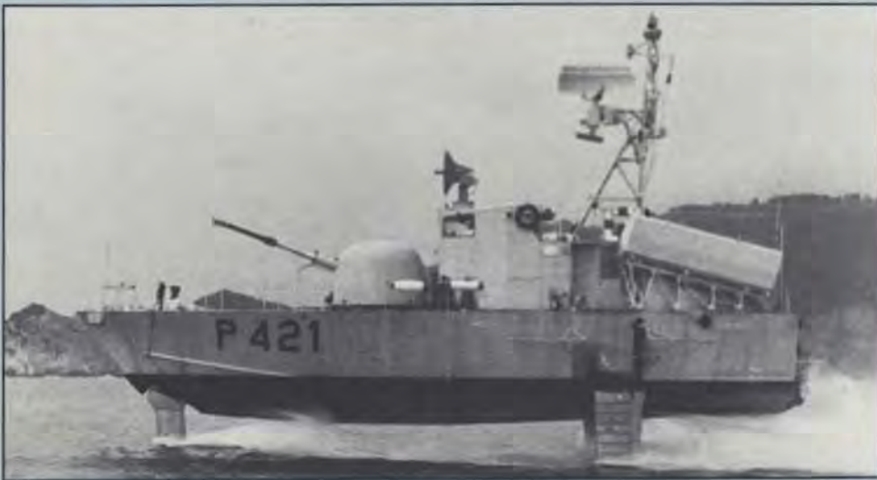
◀ The Italian navy hydrofoil Nibbio , one of seven (including the prototype, Sparviero ) to be ordered. The design of the light (62.5t), compact (23m) craft was derived from that of Boeing's Tucumcari , forerunner of the US Navy's PHM class.
