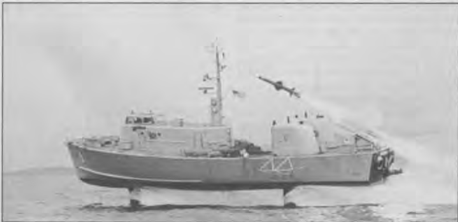
PCH 1, High point, was the first military hydrofoil by Boeing to USN BuShips design. It was used for foil experiments and Harpoon missile developments.
