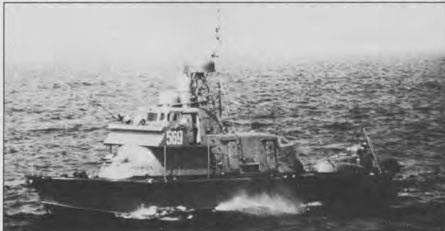
The Soviets were the first to put the hydrofoil concept into naval service, at first adapting fixed foils to FPBs such as Mo VI, above, and then purpose built fixed-foil craft like the Pchela class, seen cruising hullborne, below.
