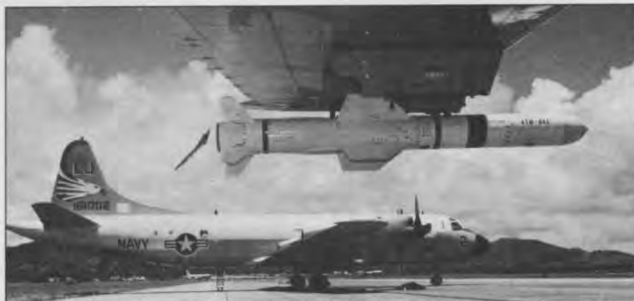
The first U.S. Navy aircraft to use the RGM-84A air-launched Harpoon missile was the P-3C Orion. These long range patrol aircraft are often called "sub-chasers," but armed with a full complement of anti-ship missiles, they become a lot more potent!
