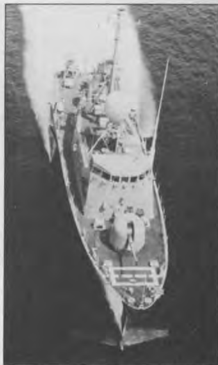
Vertical view of USS Taurus, PHM 3, second ship in commission, clearly shows deck layout and forward foil deployed.
