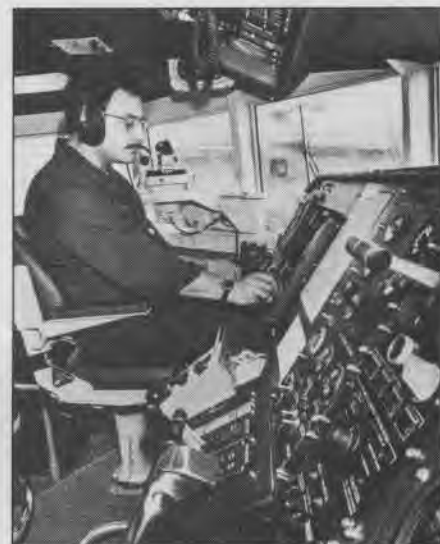
Ships controls are more reminiscent of aircraft than traditional naval vessel. Foilborne ship actually acts like plane.
