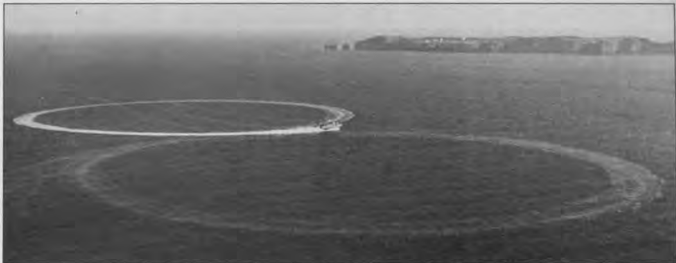
PHM's true turning radius is classified, but an idea of the agility can be gathered from this view of Pegasus cutting perfect figure eights at high speed during the early test period.
