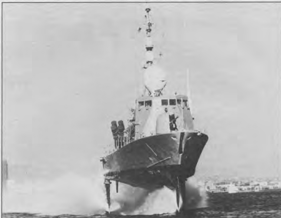
USS Pegasus (PHM 1), foilborne, top, hullborne and moored, below, was first of eventual six-ship squadron, now operational as PHMRON 2. Budget-caused delays of five years allowed time for construction improvement, and ensuing ships differ in detail. Compact CIC, bottom, controls Harpoon missiles, gun.
