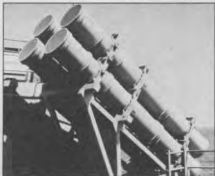
The Harpoon canister launcher was developed so that the missile could be readily adapted to almost any surface launch application. The launch structure holds four canisters, and the missile's fins and wings are folded to fit inside them.
