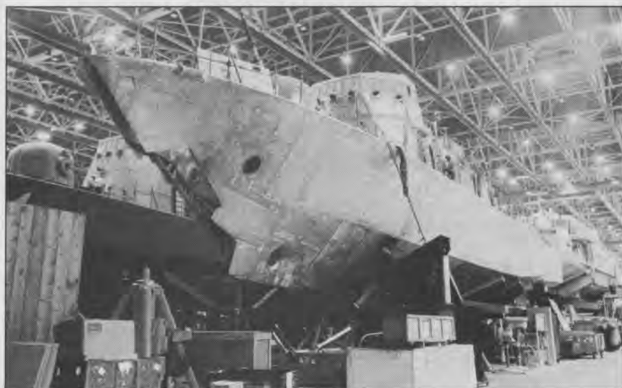
Construction of PHMs is actually a combination of aircraft and seacraft techniques. View of Boeing Marine plant shows both PHM and Jetfoil in the building stages.
