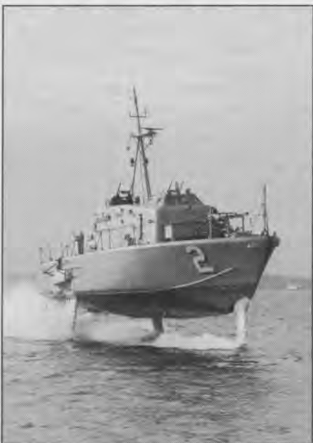
Boeing-built USS Tucumcari, PGH 2 was counterpart of Grumman PGH 1. It became the basis for the Italian CNR Sparviero.
