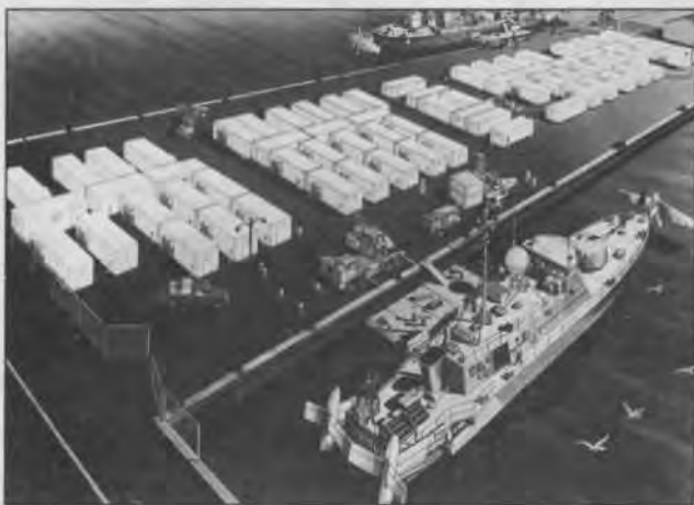
Artist's rendition of mobile PHM base which can be set up in marinas and fishing ports in almost any part of the world. Shops, offices, supplies and living quarters are all set up in modular trailer complex. Right: The difference between surface-piercing and retractable submerged foils. See sidebar.
