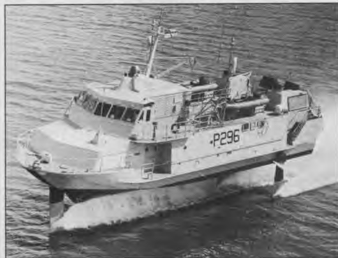
HMS Speedy was built for Royal Navy on Boeing's commercial Jetfoil hull and fitted to RN specs by Vosper Thornycroft. It began North Sea patrol duty in 1980 for multi-role evaluation. Above: the Italian Sparviero class missile hydrofoils are license-built from Boeing PGH 2, USS Tucumcari design but carry Otomat 1 missiles and Oto Melara 76 mm auto cannon.
