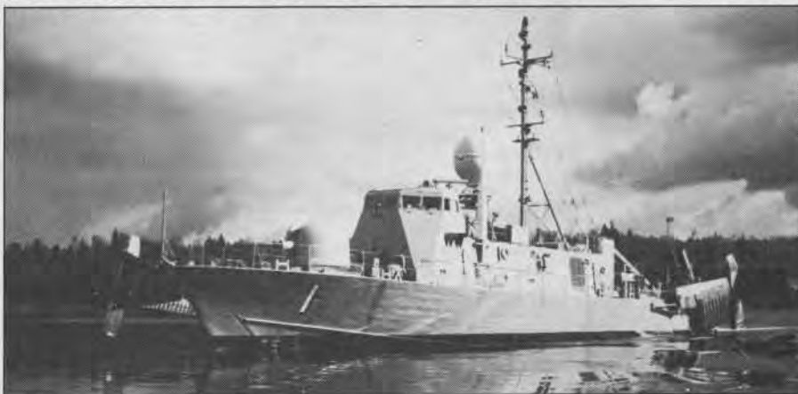
USS Pegasus (PHM 1), foilborne, top, hullborne and moored, below, was first of eventual six-ship squadron, now operational as PHMRON 2. Budget-caused delays of five years allowed time for construction improvement, and ensuing ships differ in detail. Compact CIC, bottom, controls Harpoon missiles, gun.
