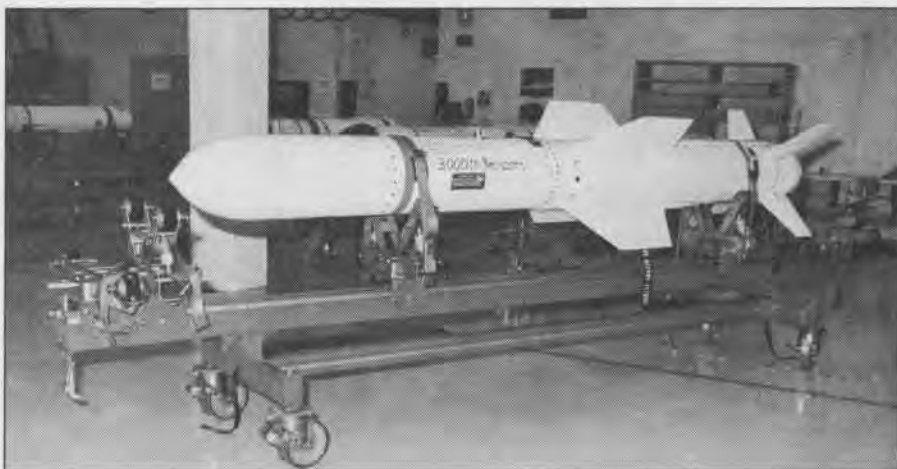
The missile's solid propellant booster launches the missile and accelerates it to cruise velocity. The turbojet engine then kicks in and the missile descends until pullout is commanded by radar altimeter. It then levels out at low cruise altitude.
