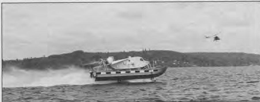
FRESH 1 was the experimental vessel built by Boeing to test foil types and configurations at high speeds. It still holds hydrofoil speed record of 84 knots.
