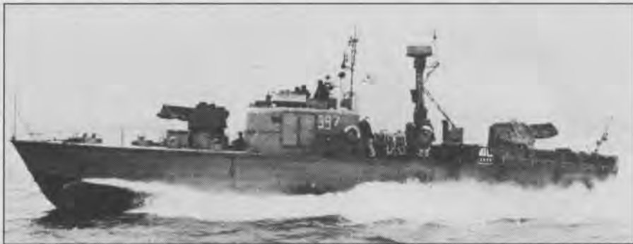
The Soviets were the first to put the hydrofoil concept into naval service, at first adapting fixed foils to FPBs such as Mo VI, above, and then purpose built fixed-foil craft like the Pchela class, seen cruising hullborne, below.
