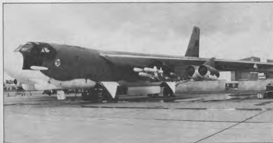
A variety of aircraft can carry the Harpoon, including the Navy's A-6E Intruder (left) and the Air Force's big B-52 bombers (below). Information on a target's location must be programmed into the missile before launch, for the Harpoon is a true "fire and forget" weapon.
