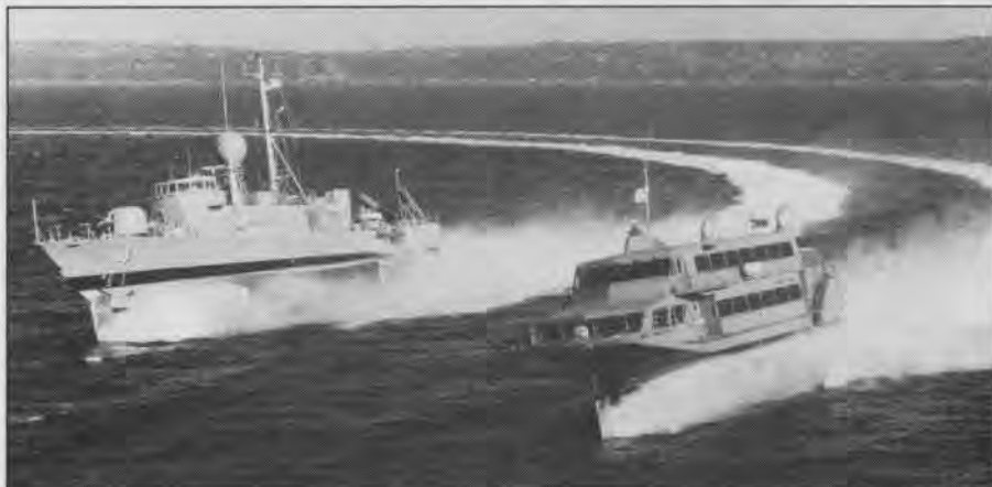
The USS Aquila, PHM 4, in Puget Sound tests with Boeing Jetfoil Bima Samudera I, built for the Indonesian navy. Performance is similar but purpose differs widely.
