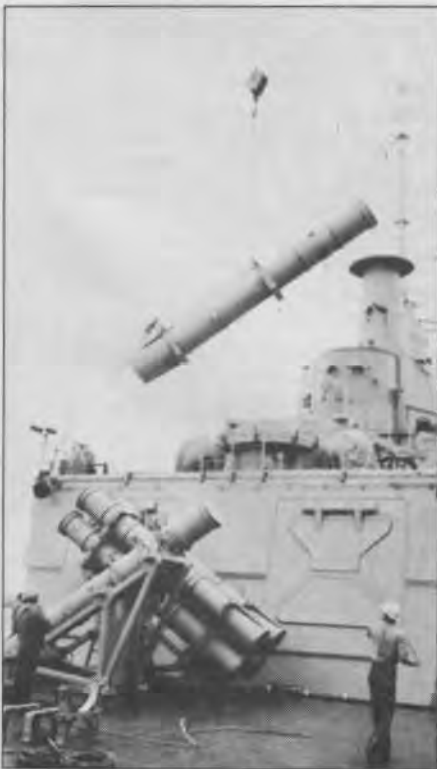
The Harpoon canister launcher was developed so that the missile could be readily adapted to almost any surface launch application. The launch structure holds four canisters, and the missile's fins and wings are folded to fit inside them.
