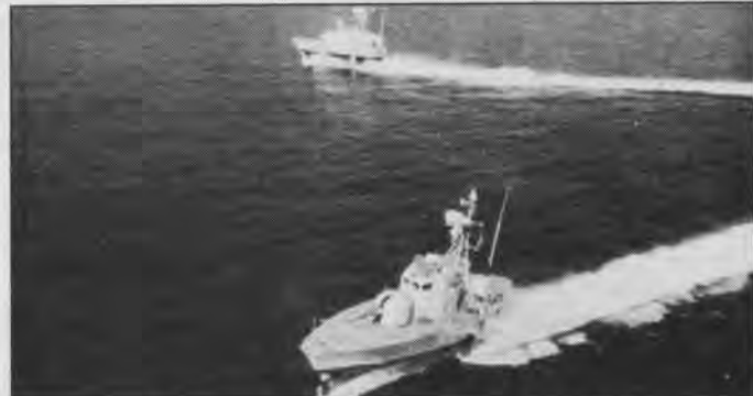
HMS Speedy was built for Royal Navy on Boeing's commercial Jetfoil hull and fitted to RN specs by Vosper Thornycroft. It began North Sea patrol duty in 1980 for multi-role evaluation. Above: the Italian Sparviero class missile hydrofoils are license-built from Boeing PGH 2, USS Tucumcari design but carry Otomat 1 missiles and Oto Melara 76 mm auto cannon.
