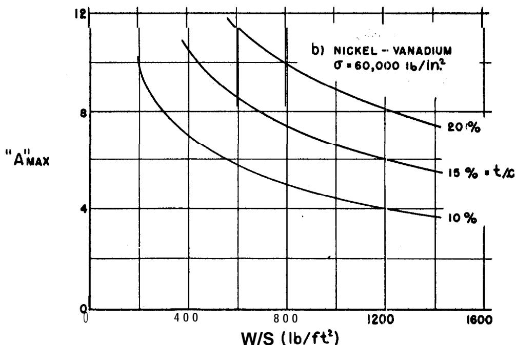
LIMITING ASPECT RATIO BETWEEN STRUTS, FOR F-4
