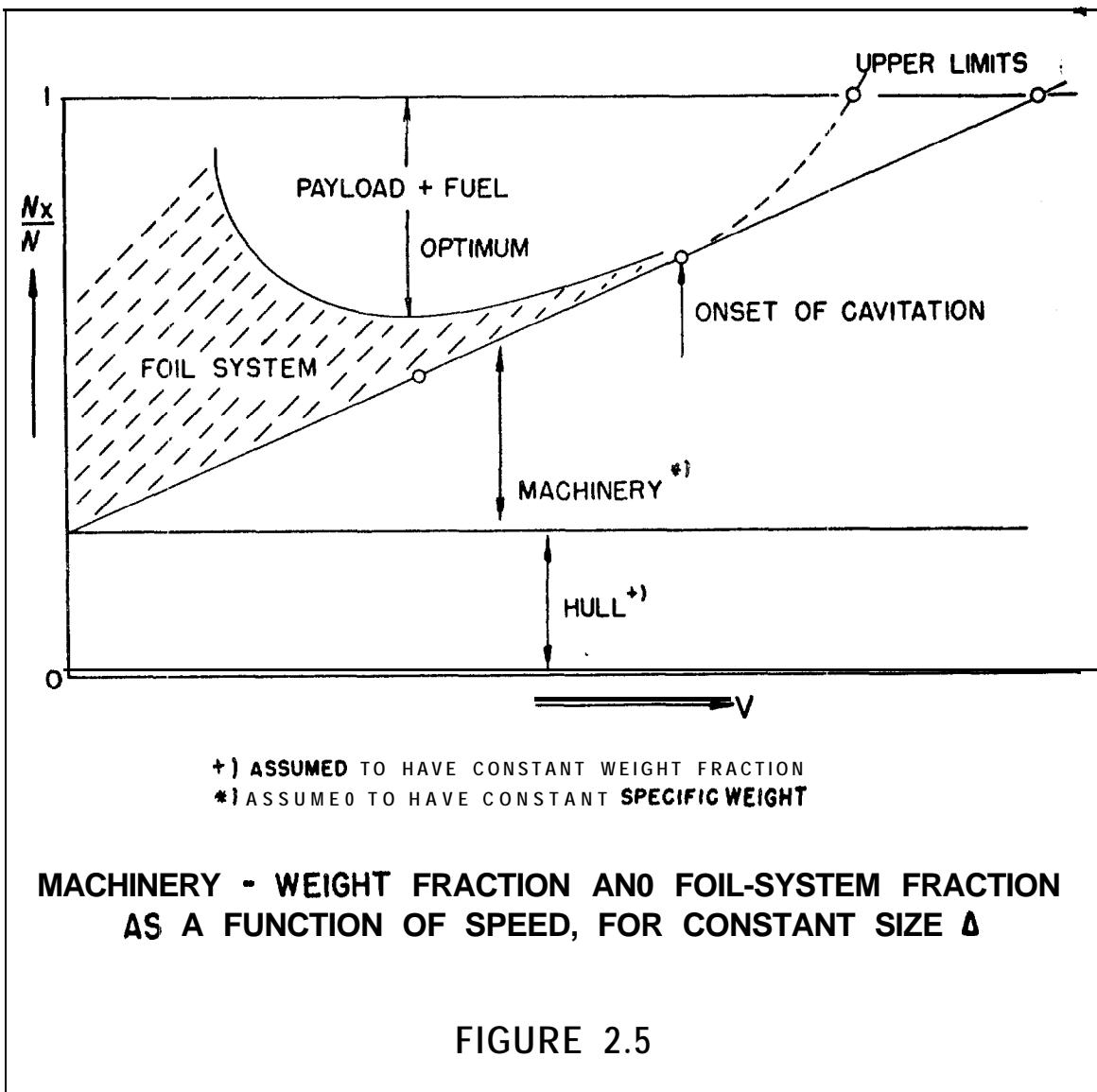
may be comparatively high; it is not realistic, however, because of cavitation setting on at some lower speed.
