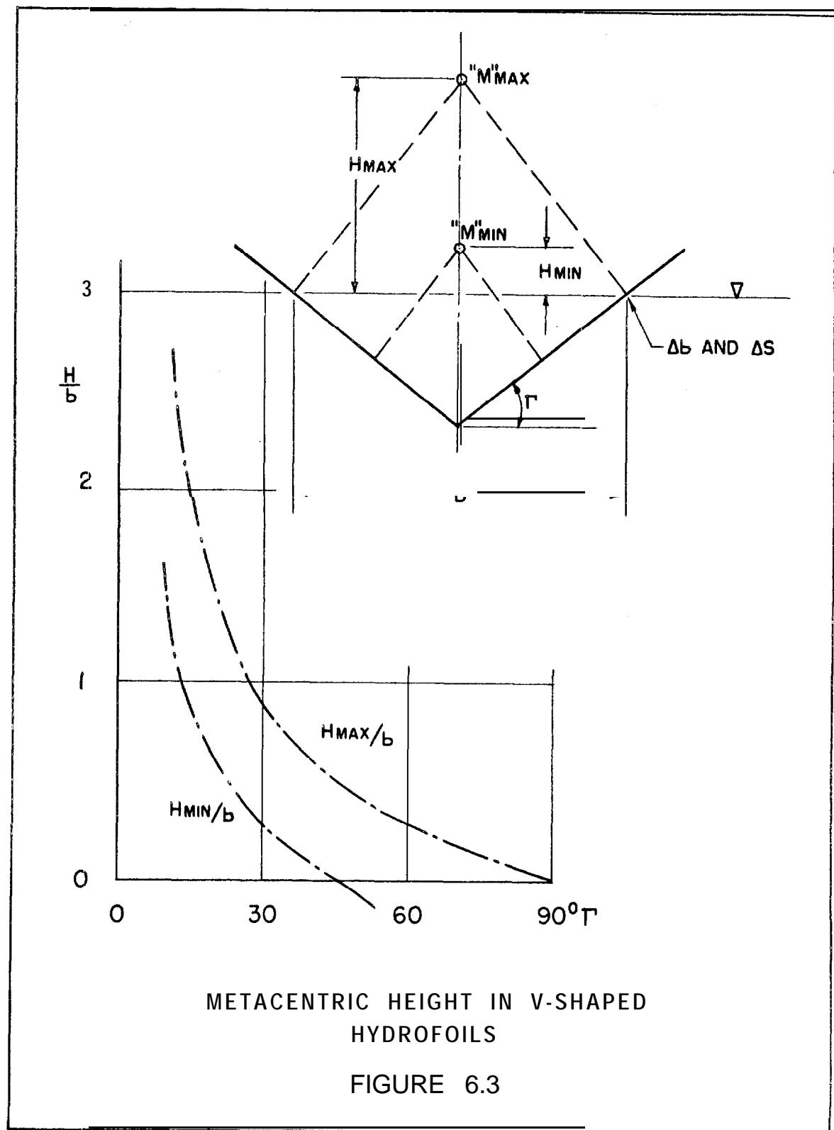
metacenter. Actually, however, it is believed that with a change at each side in submerged span, the lift is slightly changed over the entire span of the foil. As a consequence, the metacentric height due to pure rolling (without yawing) is believed to be somewhat below the " $M$ "<sub>max</sub> as indicated in Figure 6.3.
