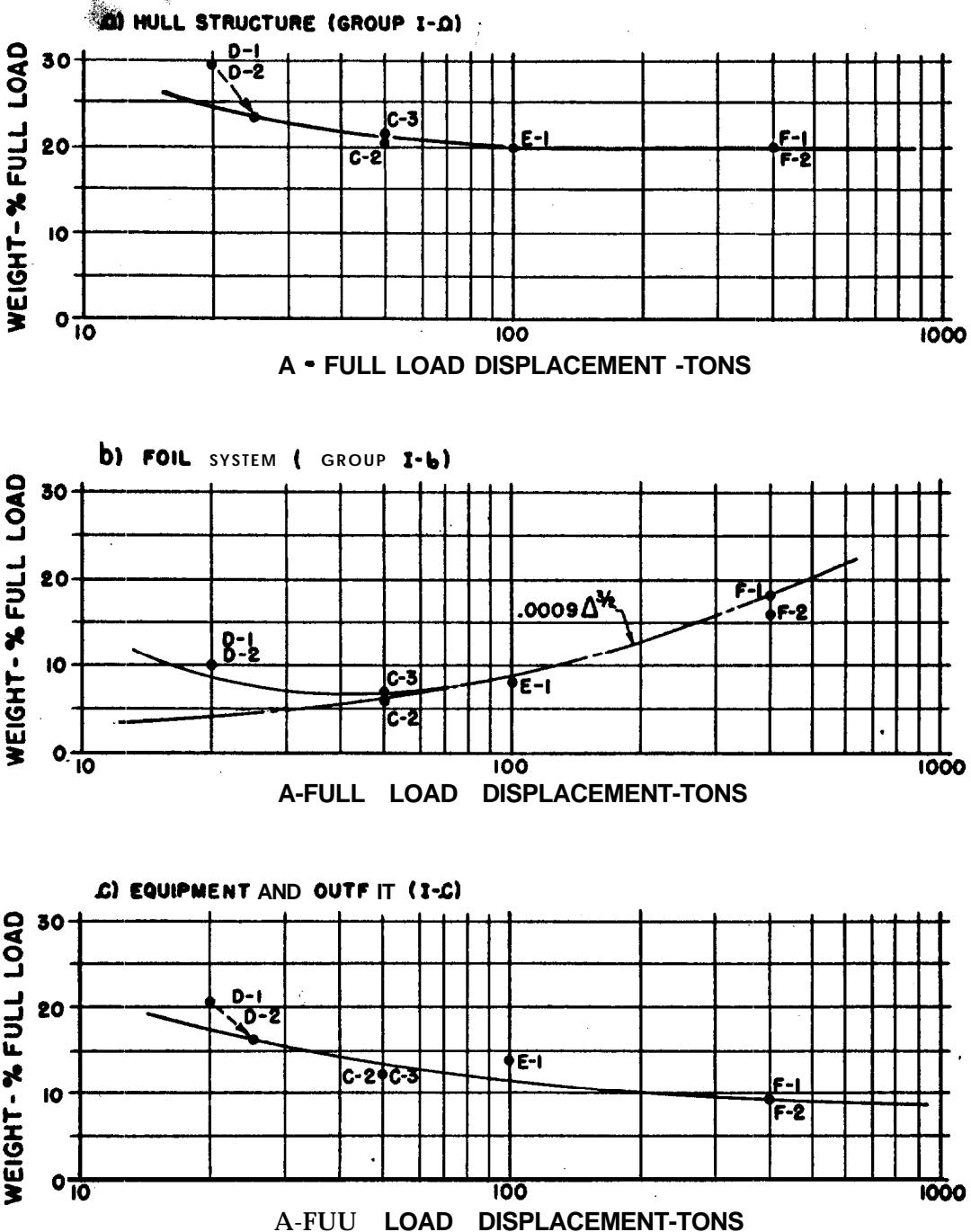
WEIGHT FRACTIONS 'OF HULL, FOIL SYSTEM, AND EQUIPMENT
