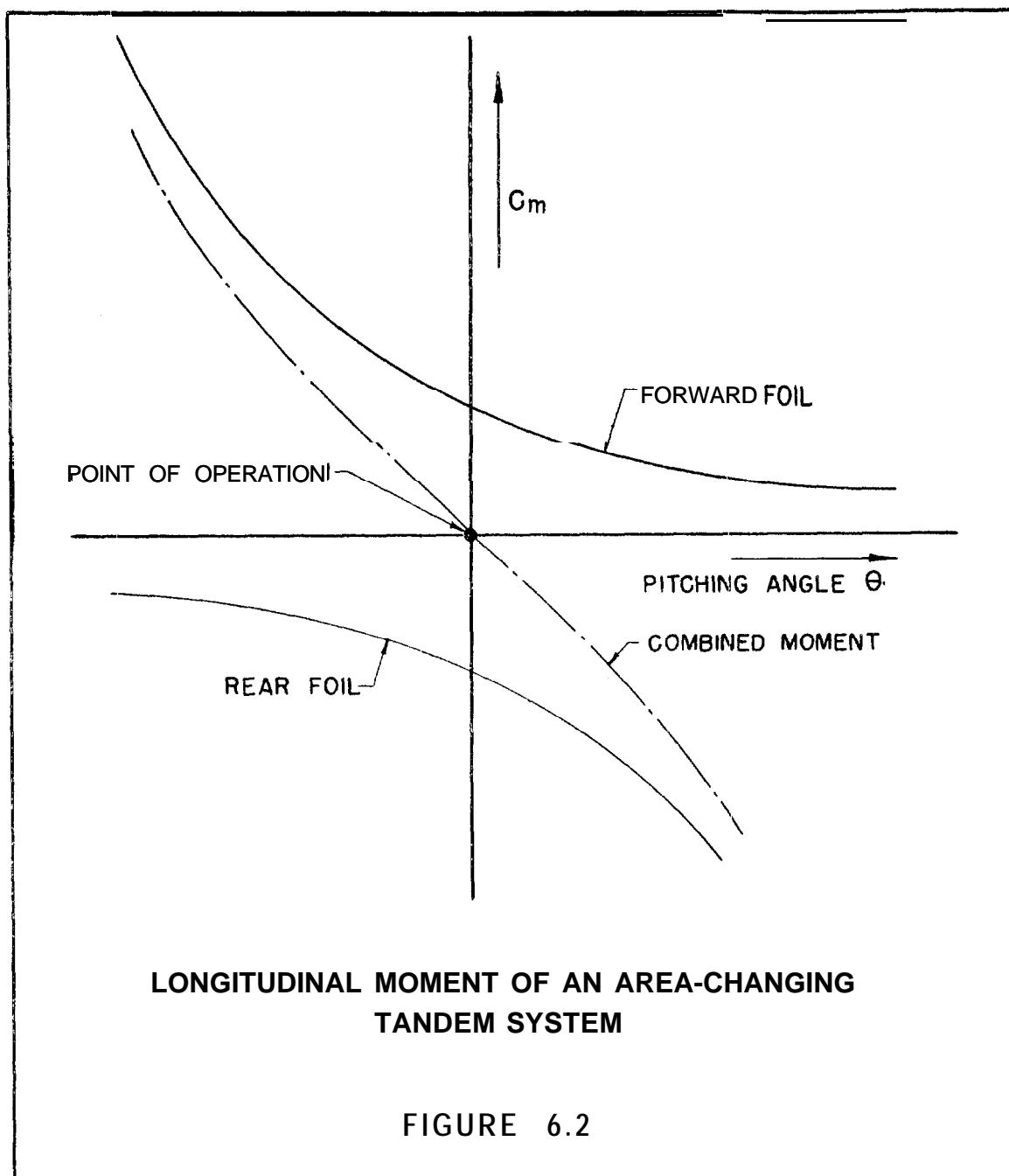
Longitudinal stability requires arrangements with at least two foils in tandem, one behind the other. In dealing with such a system, it is **convenient** to refer the lift coefficients to one and the same area, which may be selected to be the sum of the individual areas ( $S$ ). As requirement for positive **stability** it follows then from equations (6.5) and (6.8) that
