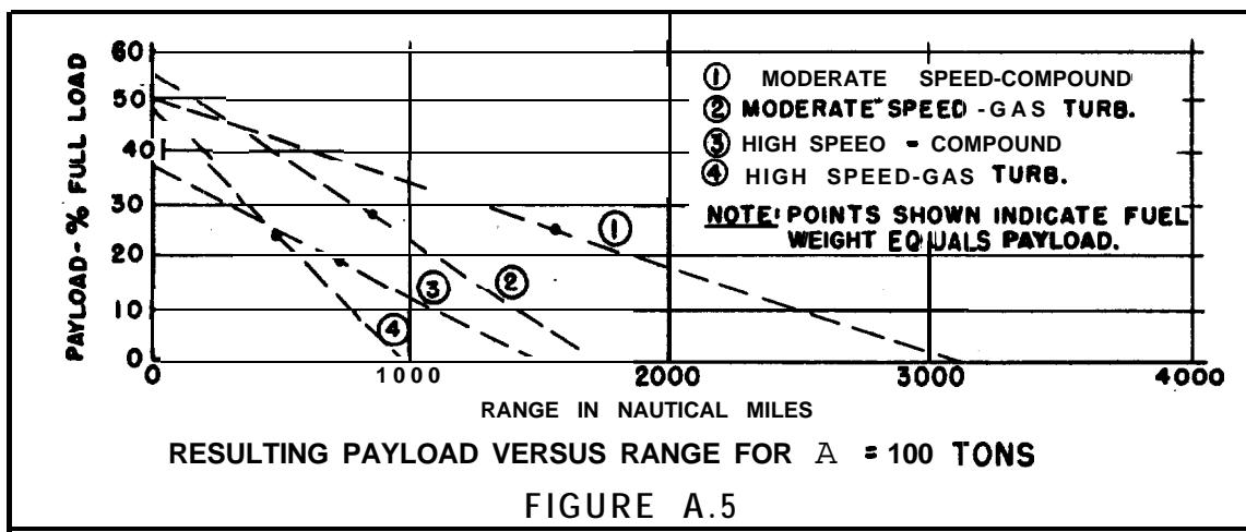
for **each combination** of each engine and design. Finally, by assuming 20% payload, the remaining weight may be translated into range. A corresponding range curve is shown in Figure A.4, showing the superiority of the compound **engine** on this basis for all but the larger (over 200 ton) high-speed craft. The latter case represents a **condition** where the better fuel rate of the **compound** engine is negated by the smaller amount of fuel available due to the large machinery weight.
