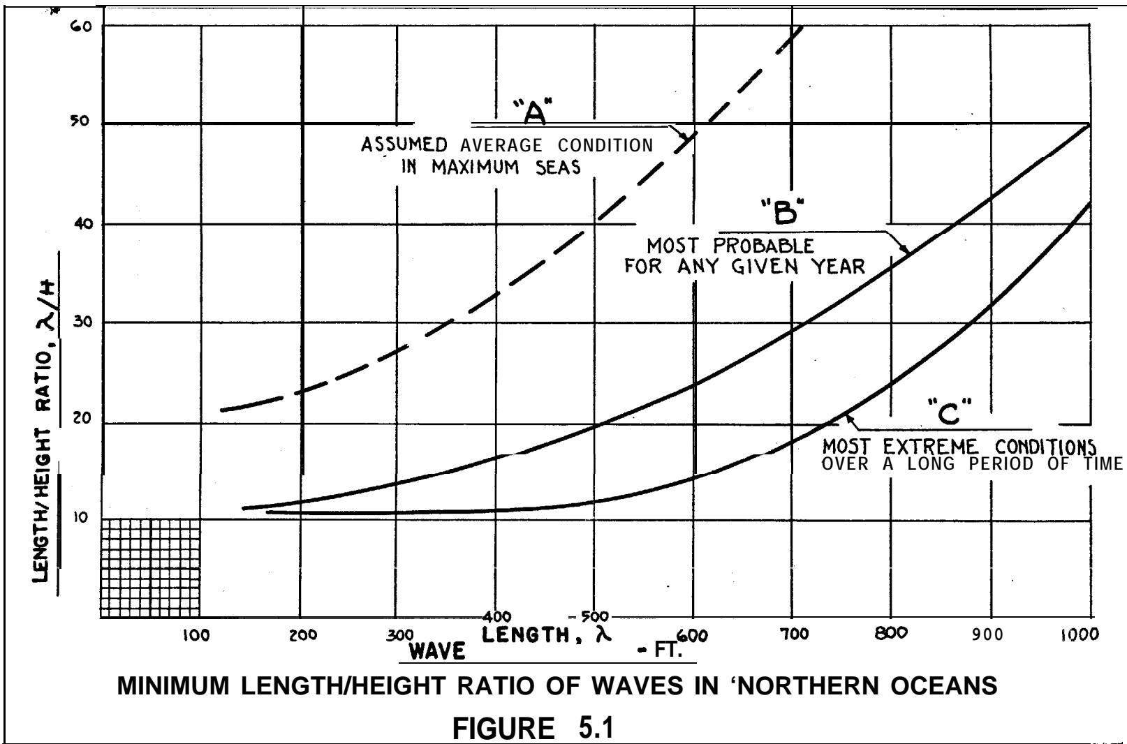
The curve identified in Figure 5.1 as "most probable relationship for any given year" (curve "B") is considered to represent the average of the 1/10th highest waves that may be experienced at sea. The curve identified as "relationship for most extreme conditions over a long period of time" (curve "C") is considered to represent the most extreme wave that may arise out of the group of waves that occur.
