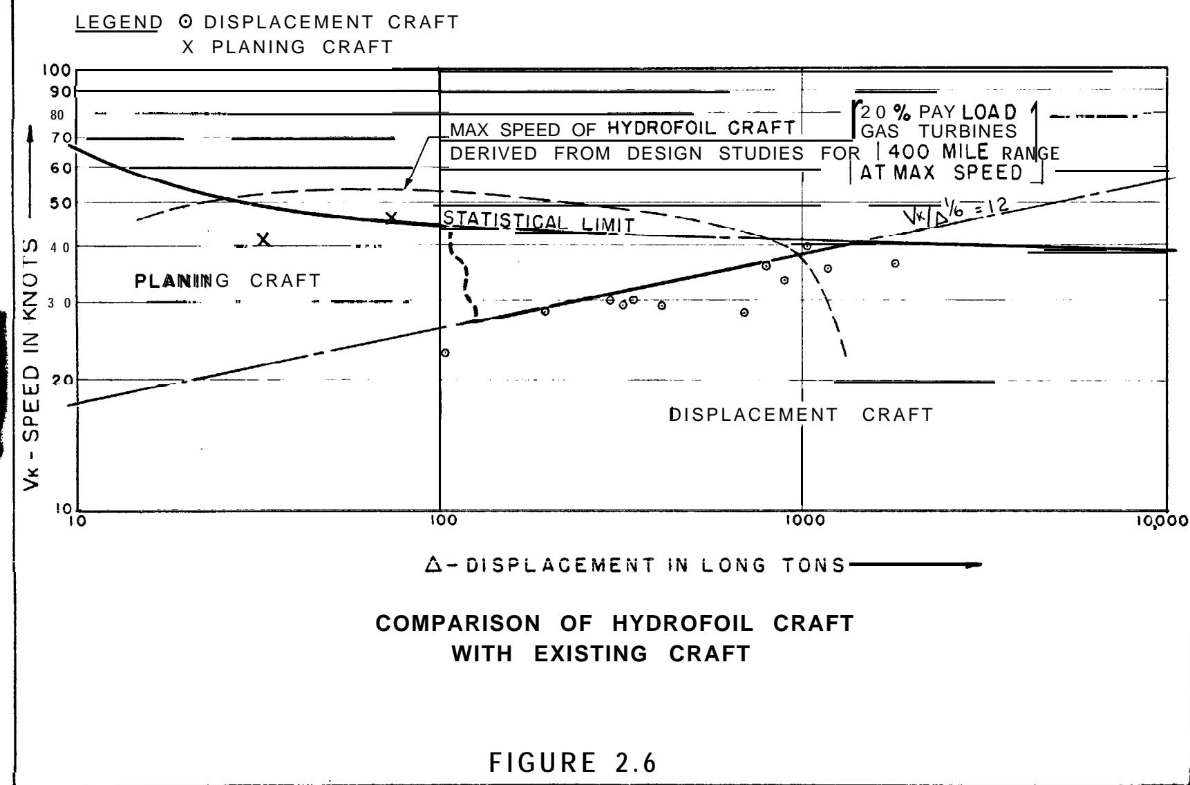
While this curve should be taken only as an illustration of such an analysis, the basic **characteristics** are probably true of hydrofoil craft in **general**; i.e. there is a size (around 1000 tons in Figure 2.6) beyond which the possible maximum design speed drops off rapidly due to running out of machinery weight.
