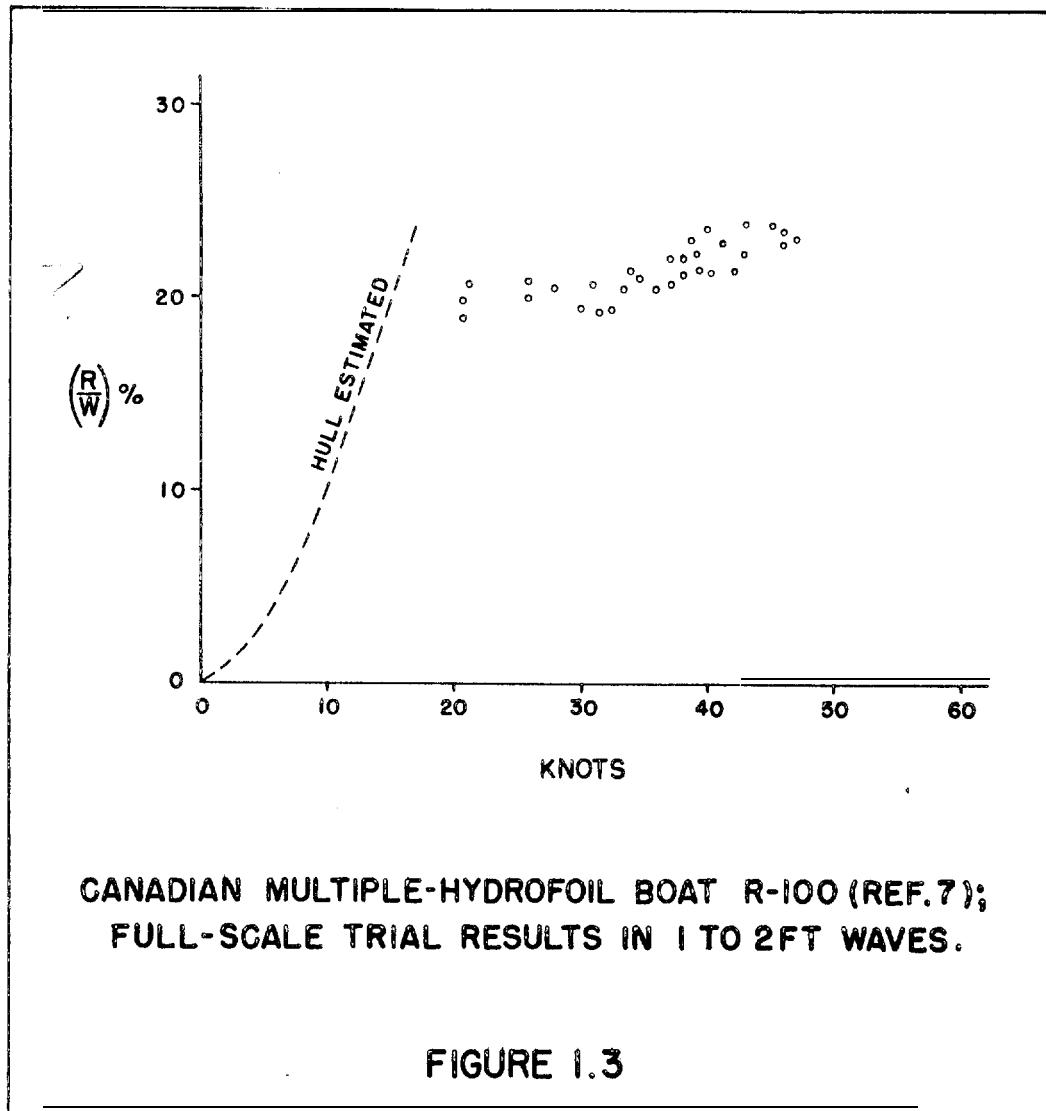
the Bell-Baldwin's optimum smooth-water value (which can be derived from reference 6, as in the order of 14%). At any rate, because of interference between foils and supporting struts and possibly because of ventilation, the efficiency of the ladder-type hydrofoil system is generally low. Disregarding this aspect, the Canadian boat has successfully operated at high speed in rough waters. Photographs of this craft are presented in reference 27.
