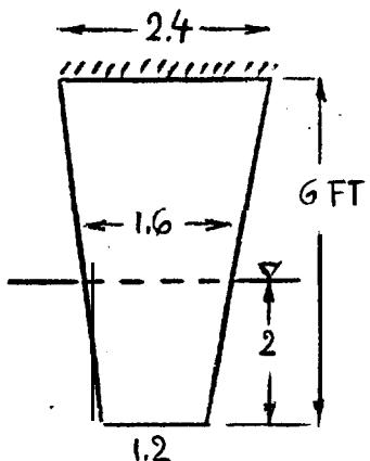
Use maximum load condition ( $2950 \text{ lb/ft}^2$ ) for the section at 6 ft; extreme loading ( $3120 \text{ lb/ft}^2$ ) for the section at 2 ft. Include a safety factor of 1.15 on the yield for both.
