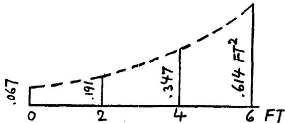
Note: Strut weight appears excessive compared to foil weight; may be greatly reduced by employing hollow sections, particularly above the 2 ft section.
