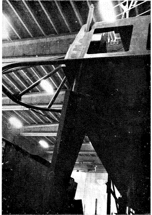
The upper section of the foil support, with rudder and rudder cylinder. The rudder shaft is extended upwards in compliance with the Shipping Directorate's demand for an emergency rudder.
