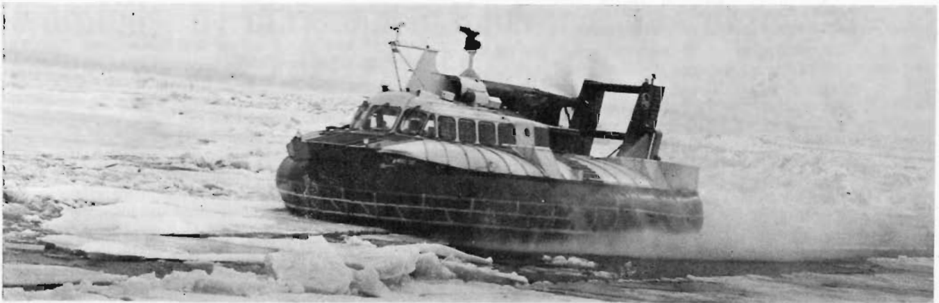
At a time when no sensible mariner would be seen out of port, the Bell Aerosystems SK-5 air cushion vehicle skims over jagged ice as it proceeds across Lake Erie. In making this trip, the SK-5 became the first surface vehicle to travel the length of Lake Erie—a 500-mile round trip journey—under winter conditions before the opening of the navigation season. The craft also successfully demonstrated the feasibility of an ACV to provide year-round transportation between Pelee Island and the Canadian and US mainlands
