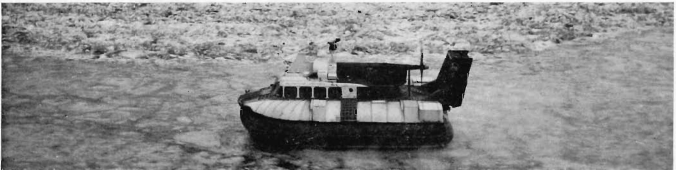
Two different ice conditions encountered by the SK-5 are visible here as the craft skims over Lake Erie. The craft was heavily instrumented to record its performance, and crossed ice obstacles up to 5 ft high achieving speeds exceeding 50 mph
