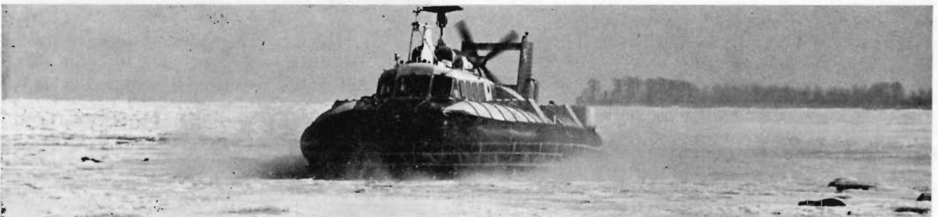
Boulders locked in ice were only some of the obstacles encountered by the SK-5. During its 500-mile round trip the craft gathered engineering data on the overall performance, handling qualities and operation of an ACV over a maximum range of Lake Erie winter conditions, such as rough, broken and smooth ice, calm and rough water, freezing temperatures, snow and fog
