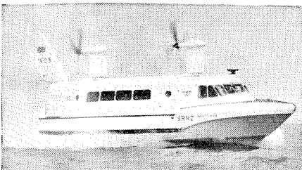
The Westland SRN 2 powered by four Nimbus engines.
