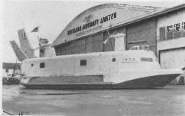
Westland's SR.N3 has recently been completed by the company's Saunders-Roe Division and is now undergoing preliminary trials at Cowes, Isle of Wight. Largest ACV in the world, it weighs 37½ tons and has been built specifically for evaluation by the British armed services
