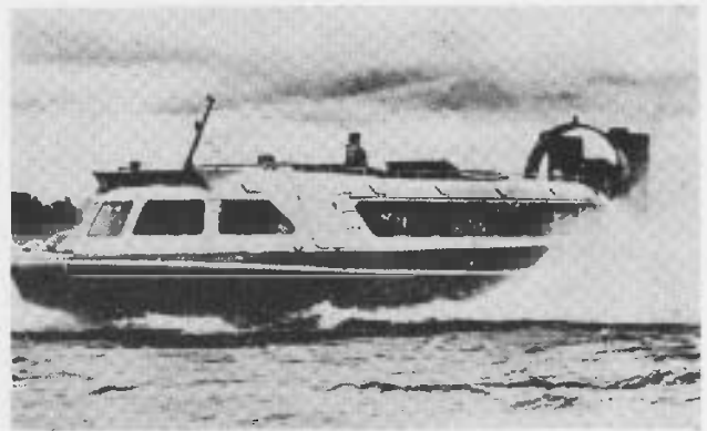
Figure 14. Russia, Leningrad Institute of Water Transport 38-seat plenum chambered craft
