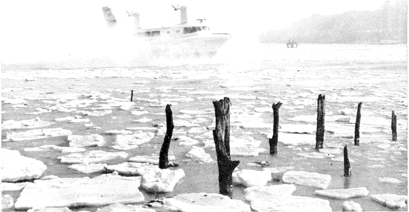
The Westland SR.N2 operating over pack ice up to 9 in. thick and floes 6 ft. long in Wootton Creek, Isle of Wight. Icing tests at sub-zero water and air temperatures showed that the craft's operation at normal speeds and hovering heights was unimpaired and its fundamental mechanisms were unaffected
