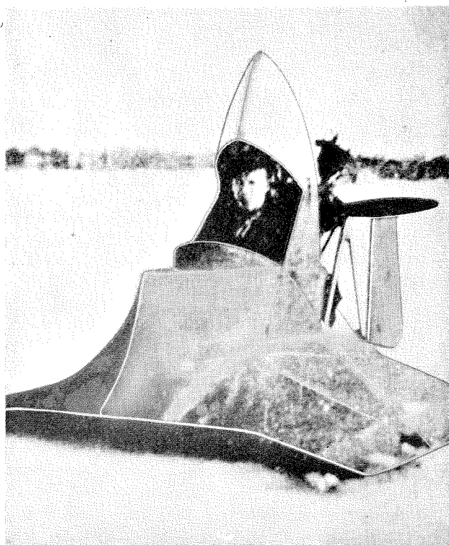
Figure 29. Kaario's first ground effect machine, built in Finland in 1935. It attained a speed of 12 knots with a 16 hp engine
