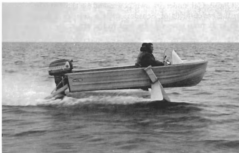
The Sea Wings were a spin-off from Grumman's hydrofoil research.
