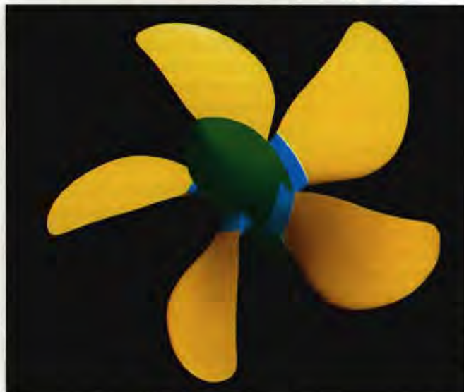
A propeller modeled in MultiSurf and rendered with IRISView on a Silicon Graphics Personal Iris.
