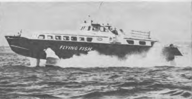
FIRST PASSENGER HYDROFOIL in U. S., beginning operation this summer between Bellingham, Wash., and Victoria, B. C., is foreign-built Flying Fish—a 60-passenger, 27-ton vessel.
