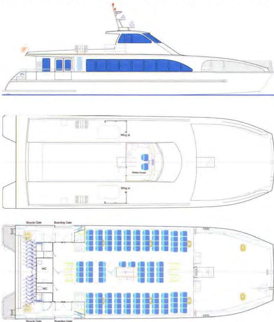
General arrangement of Teknicraft Design 24m foil assisted catamaran Rich Passage 1
