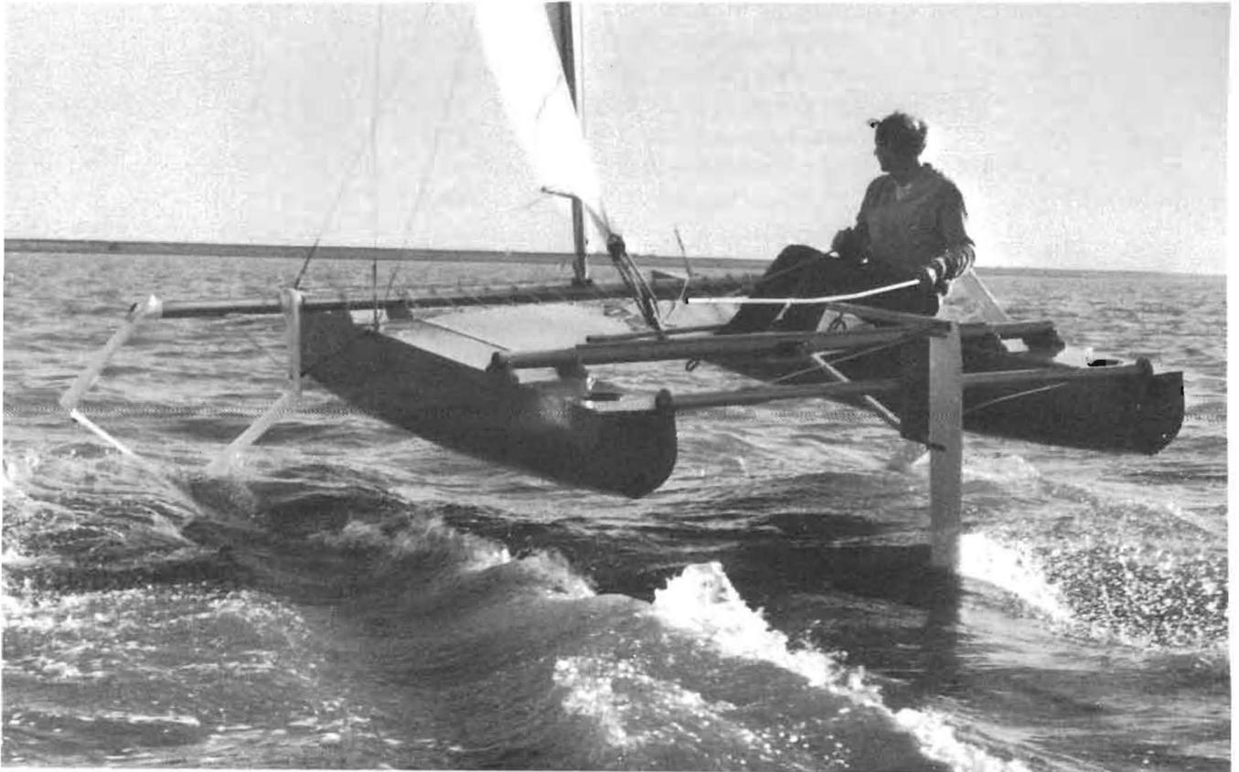
possible theoretical objections, the front foils were set to 4°. The boat was found to lift-out easily, and sail in a fast and stable manner (fig. 51). She is highly manoeuvrable, both in displacement sailing and on the foils, and can tack either on or off the foils, without performing a stern-board. The only problem in stability is a tendency for the bow to go down at speed, and this has been corrected by making a special seat each side to carry the helmsman's weight back almost to the transom.
