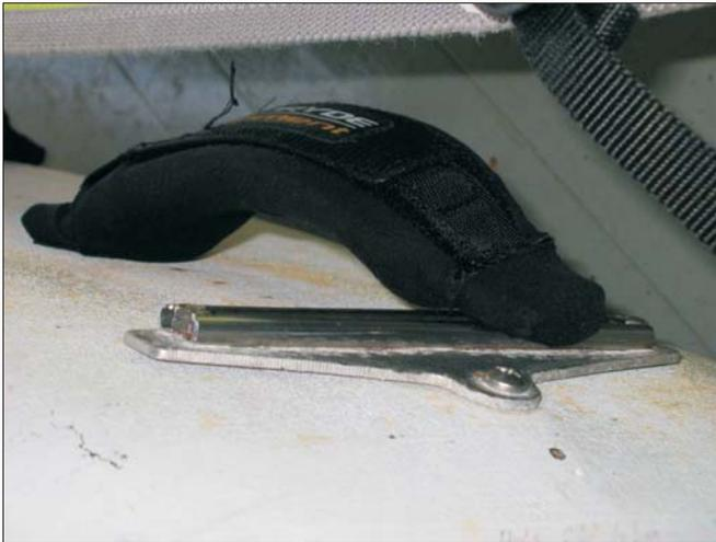
Mount a single aft foot strap on the board centerline, centered fore and aft over the main retaining screw. The picture shows an alternate installation with aft end sliding on a transverse track. This arrangement lets the heel of the foot come more over the board centerline.
