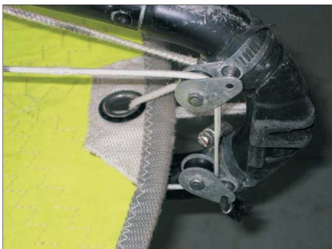
The tail blocks are attached below(!) and at the rear corners of the boom by means of the integral stainless hose clamps
