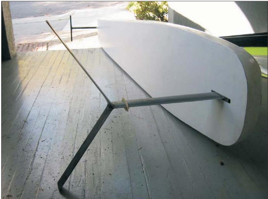
The main foil assembly consists of a fin and two wings -- a small fence located on the fin above the “Y” junction is visible in the photo
