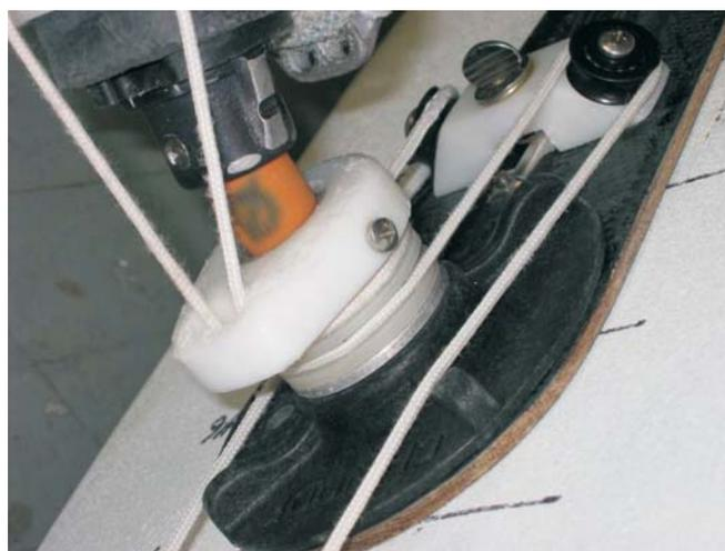
A good initial position for the base universal is 46" forward of the main foil retaining screw
