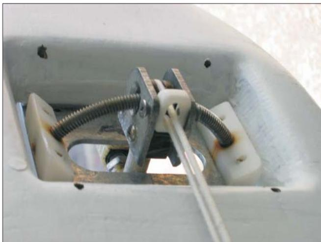
Feed the control loop cord (the "canard loop") through the frame so that it comes out on the deck side
