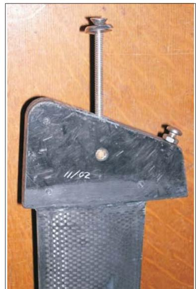
Fin head showing retaining screw and washers and the adjusting screw with jam nut
