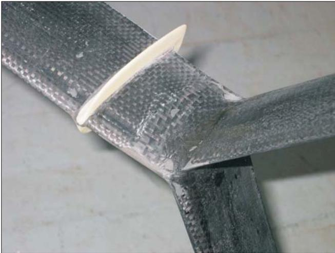
One small ventilation fence located 2" up from the "Y" junction at a small positive attack. Helps prevent flow of air down the suction side of the fin to the wings.
