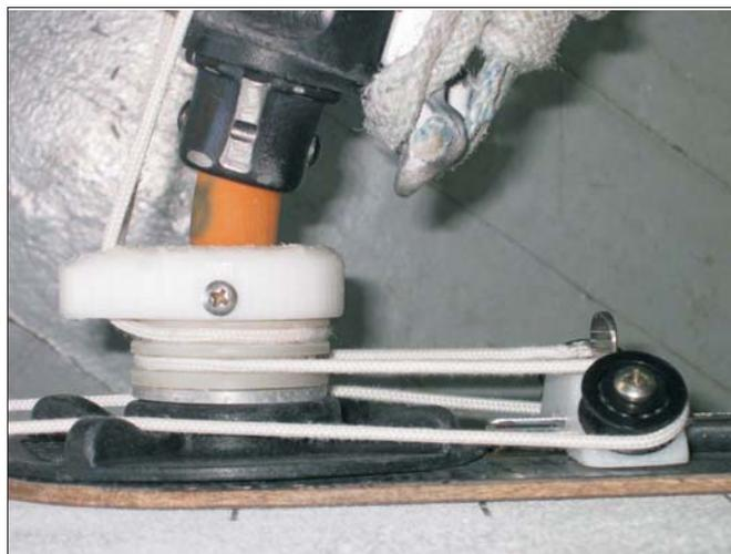
Mount the mast base and canard loop tensioner in the mast track, with the tensioner aft of the base
