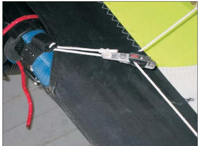
Port mast block and webbing, with boom loop in place -- make a final test of the canard mechanism by pulling on the boom loop
