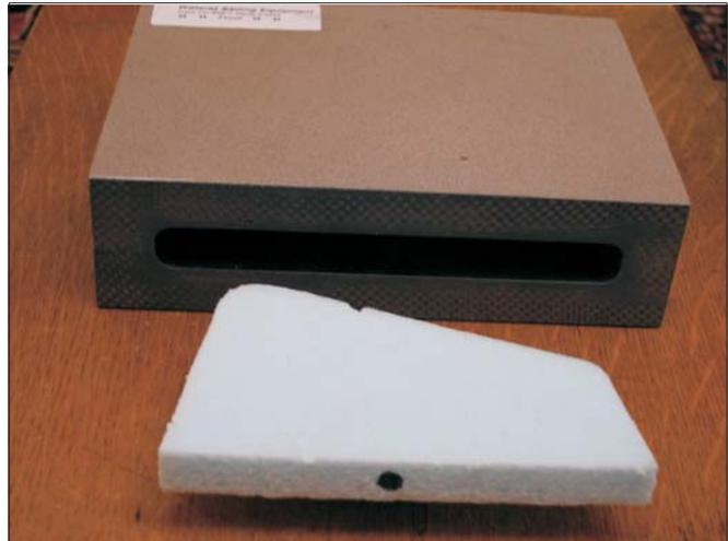
Tuttle box shown from bottom and Styrofoam plug used in adapting the box to carry the fin head --The opening in the box is 5/8" x 6" and the outside dimensions are 2" x 7.75" x 5.75"
