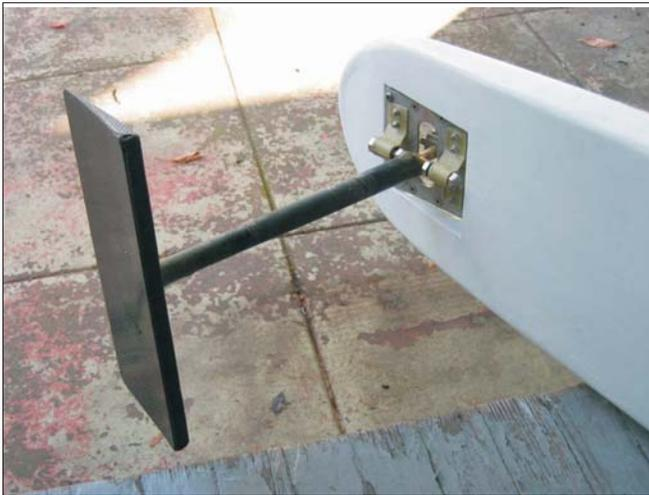
The front foil (canard) assembly consists of a supercavitating-type foil (section looks like a meat cleaver, with a sharp leading edge and a blunt trailing edge), and a stiff strut
