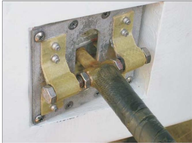
The canard assembly must be hinged at its top end (where it attaches to the nose of the board) so that it can be deflected in roll and locked in deflected position
