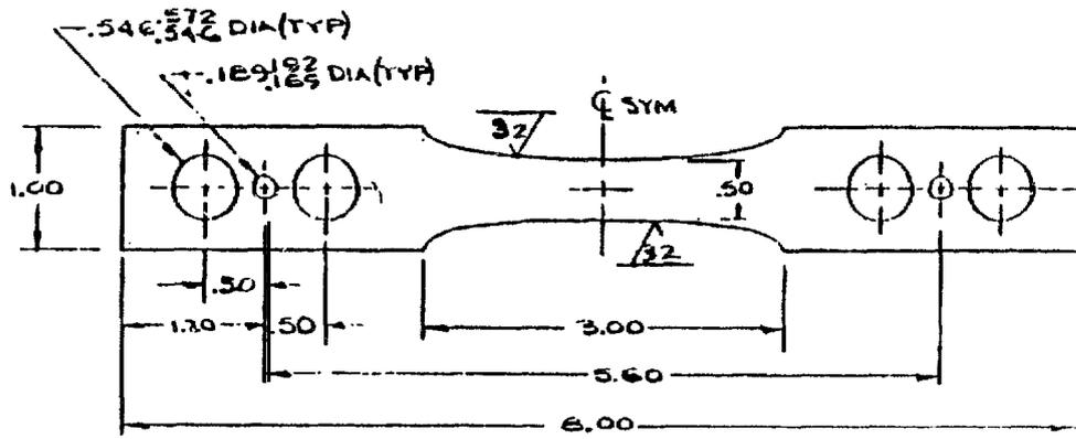
NOTE: THE NATURAL SURFACE FINISH OF THE SPECIMEN MUST BE PRESERVED. DO NOT POLISH. USE EXTREME CARE IN CLAMPING SPECIMEN IN JIGS FOR MACHINING. SCRIBE MARKS, SCRATCHES, NICKS, GOUGES, ETC, WILL BE CAUSE FOR REJECTION.
