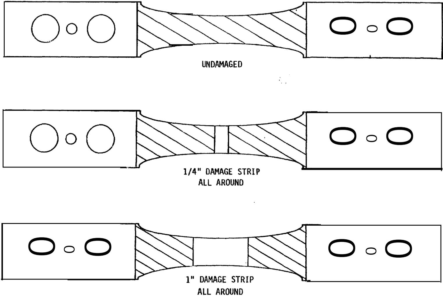
FIGURE 2 COATING CONFIGURATION
