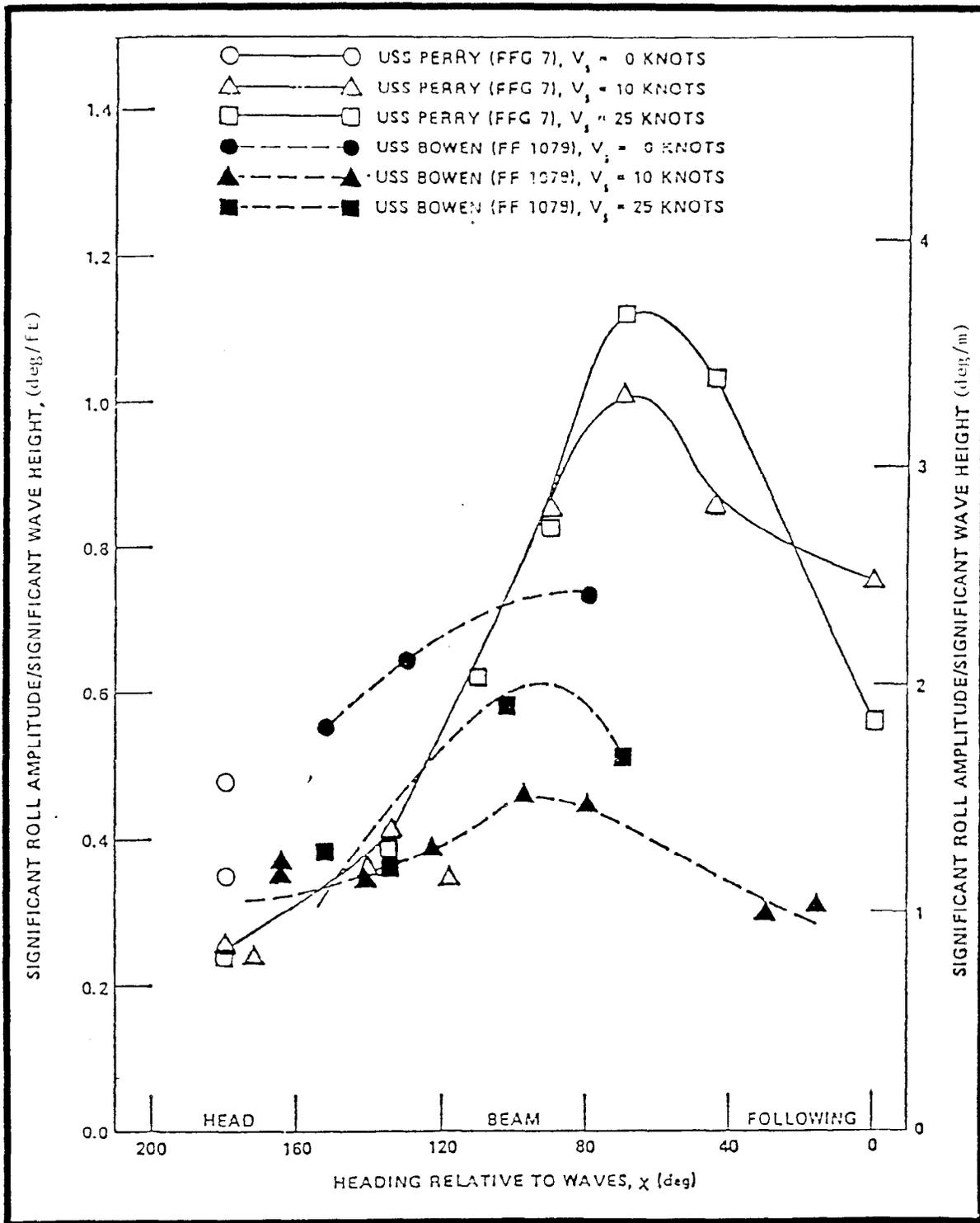
Figure 3.2.3-19. Significant Roll Amplitude Per Unit Significant Wave Height Versus Heading Relative to Waves from the Trials Conducted on the USS PERRY (FFG-7) and the USS BOWEN (FF 1079) at Ship Speeds of 0, 10 and 25 Knots (Reference 17)
