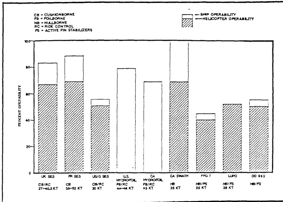
Figure 3.2.3-57. Comparison of Percentage Operabilities of ASW Ships at High Speed in the Northern North Atlantic in Winter
