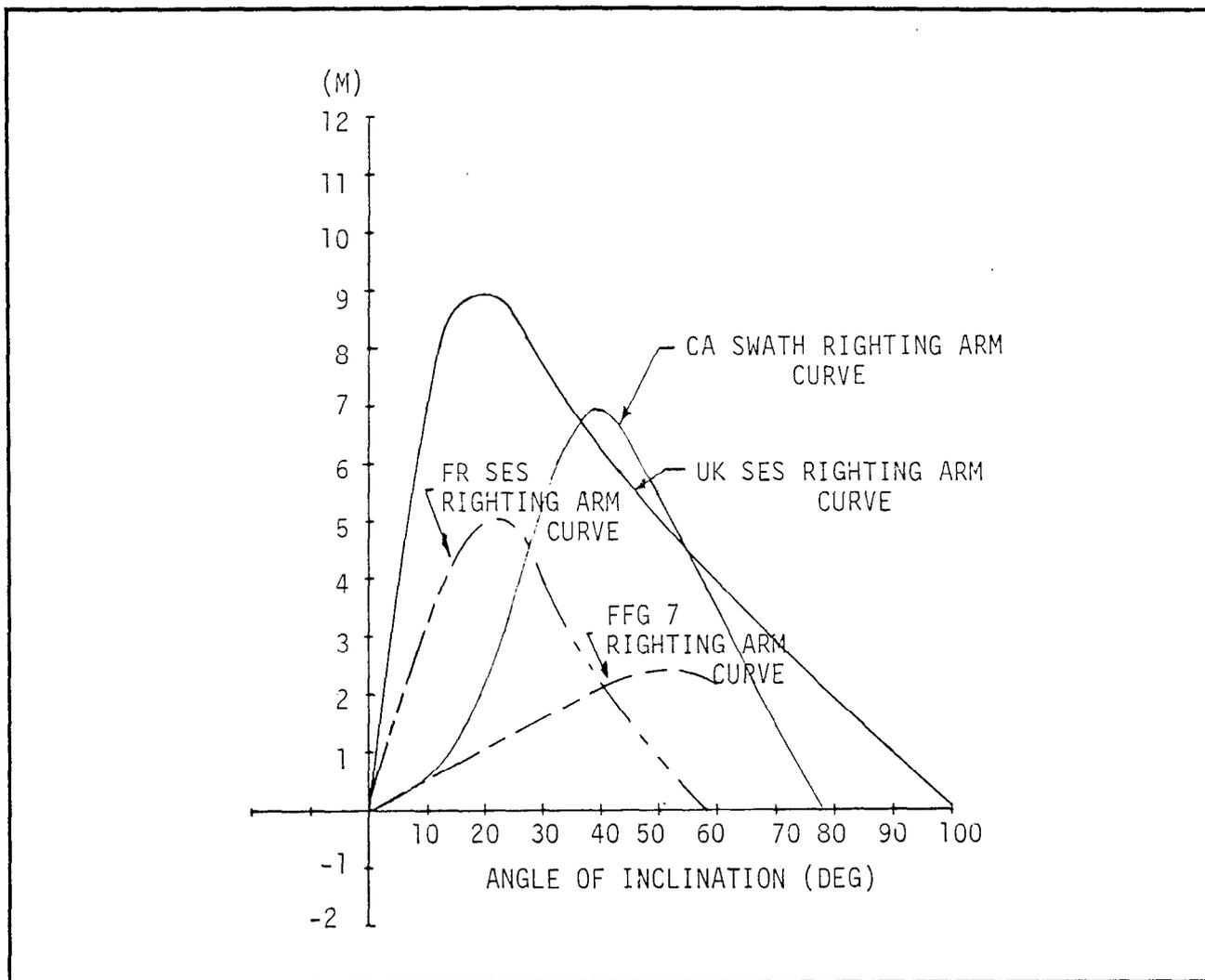
Figure 3.3.21-1. Intact Righting Arm
