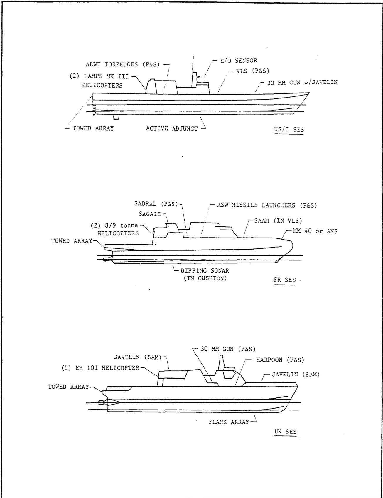
Figure 3.2.6-2. Combat Systems Arrangements Profile View (Sheet 1 of 2)
