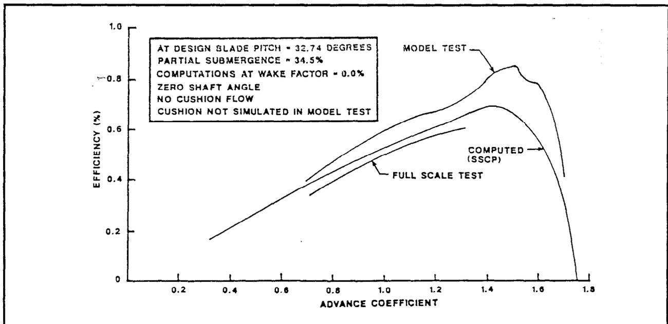
Figure 3.3.6.3-2. SES 100B Propeller Performance
