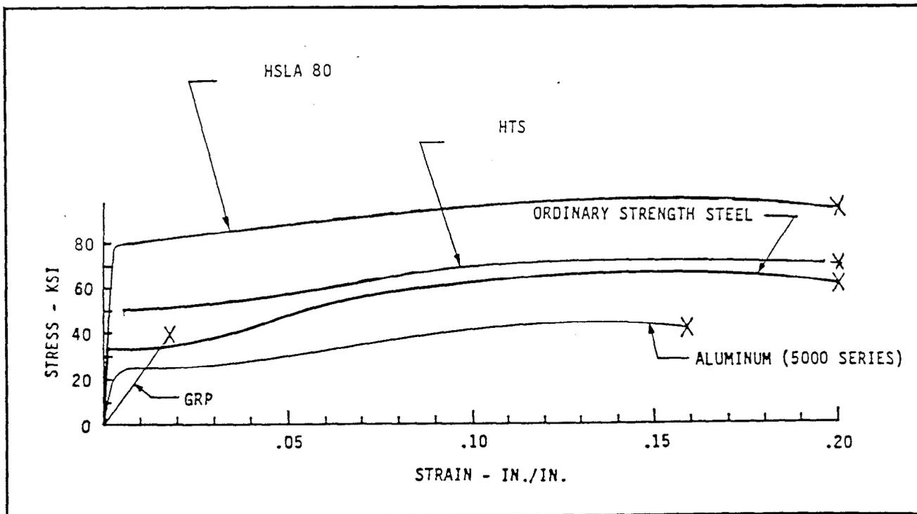
Figure 3.3.3-2. Representative Tensile Stress Strain Curves
