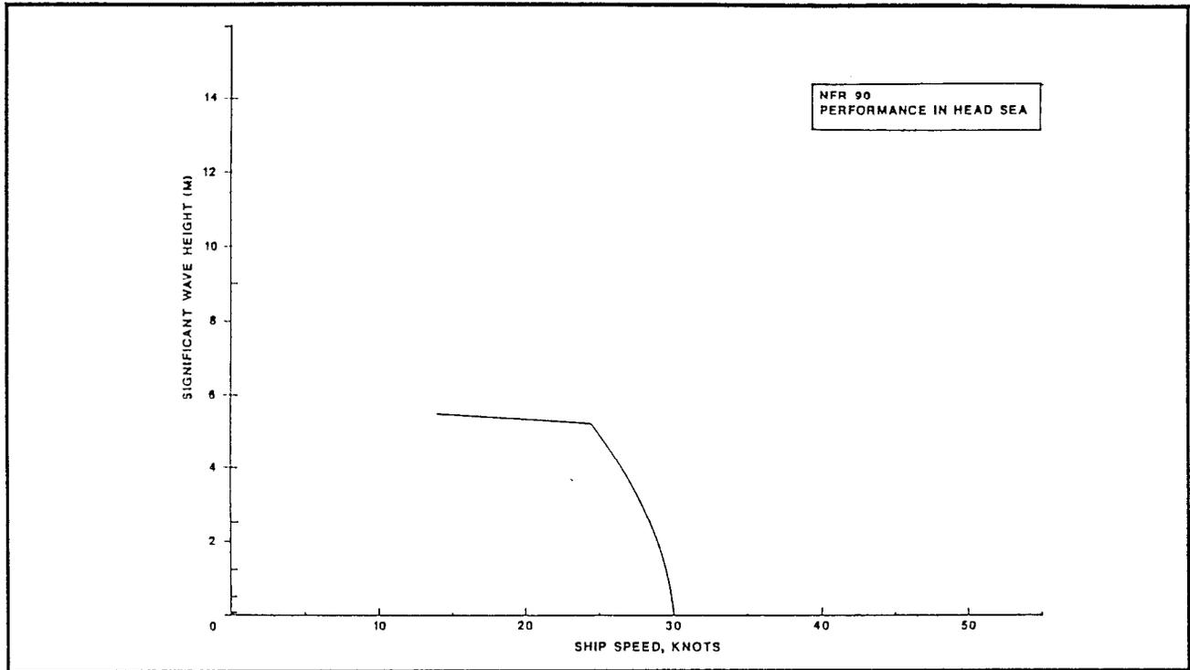
Figure 3.2.1-11. Maximum Sustained Speed Versus Sea State - NFR 90
