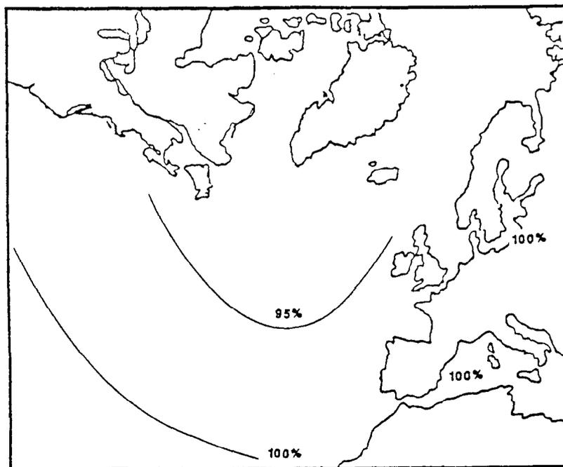
Figure 3.2.3-48. Operability Contour, UK SES, 27-40.6 Knot Range, Ride-Control, On-Cushion, Annual North Atlantic Average (Ship Operability)
