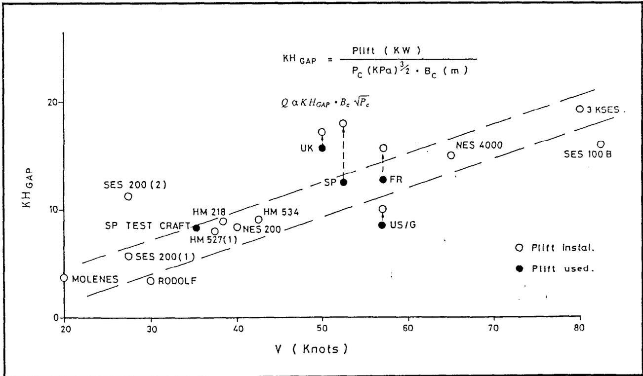
Figure 3.3.7-3. SES Cushion-Air-Flow Seal-Leakage Air Gap Related to Forward Speed
