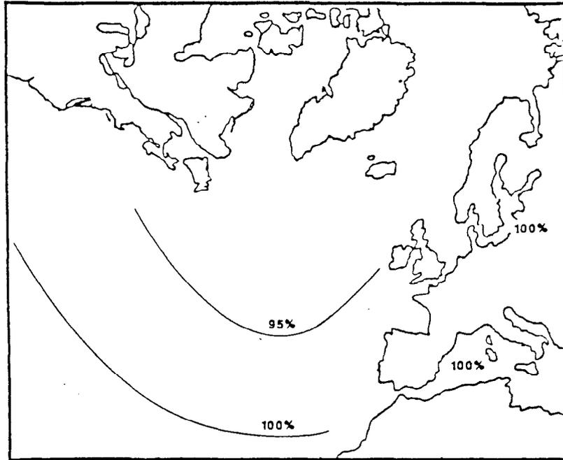
Figure 3.2.3-49. Operability Contour, UK SES, 11-17 Knot Range, Off-Cushion, Annual Average, (Ship Operability)
