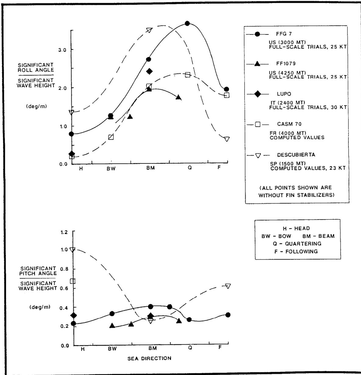
Figure 3.2.3-20. Comparison of Monohull Frigate Seakeeping Data
