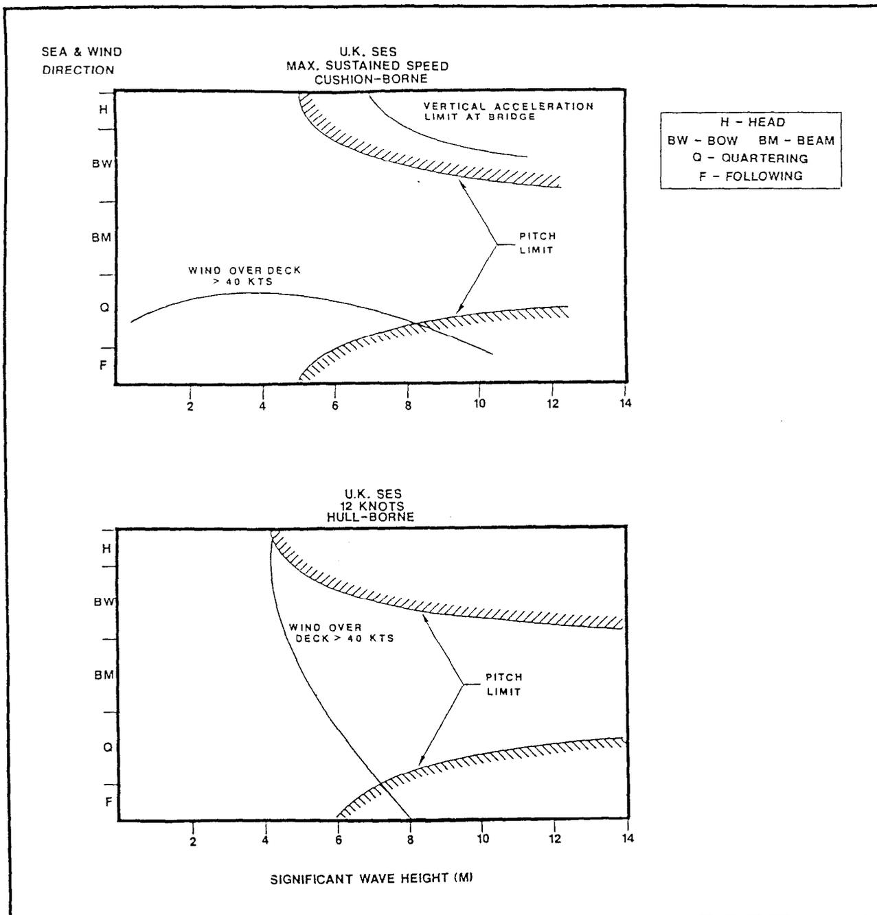
Figure 3.2.3-23. UK SES Seakeeping Limits - Effect of Wave Height and Heading
