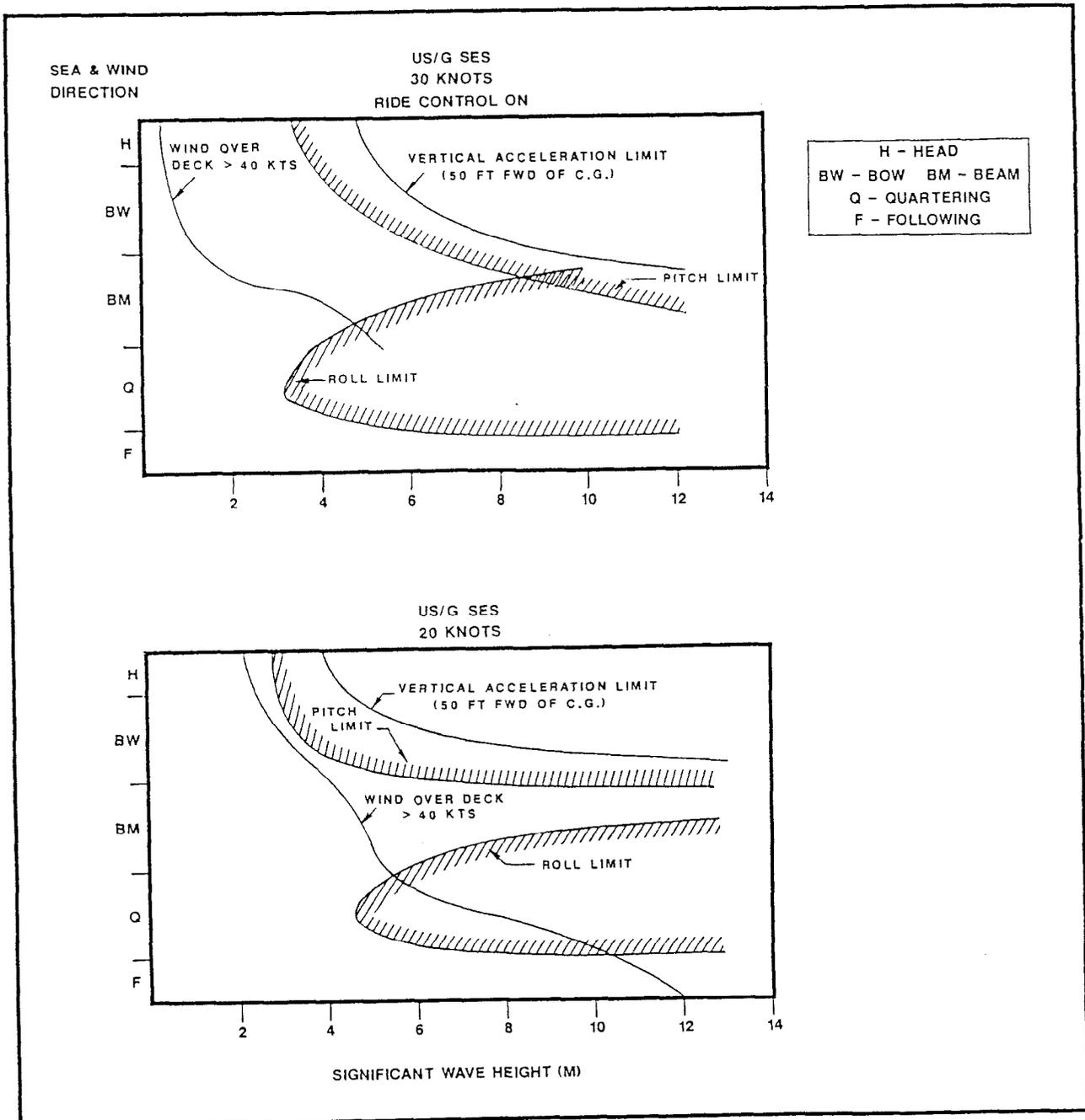
Figure 3.2.3-25. US/G Seakeeping Limits - Effect of Wave Height and Heading
