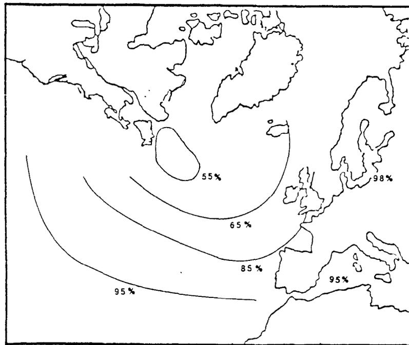
Figure 3.2.3-37. Operability Contour, US/G SES, 30 Knots, Ride-Control, On-Cushion, Winter (Ship Operability)
