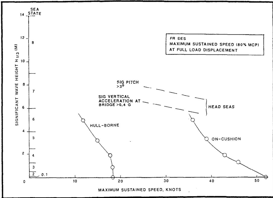
Figure 3.2.1-5. Maximum Sustained Speed Versus Sea State - FR SES
