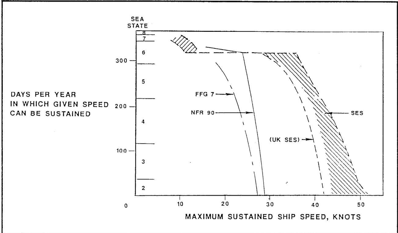
Figure 3.1.2-5. Maximum Sustained Speed for SES in North Atlantic
