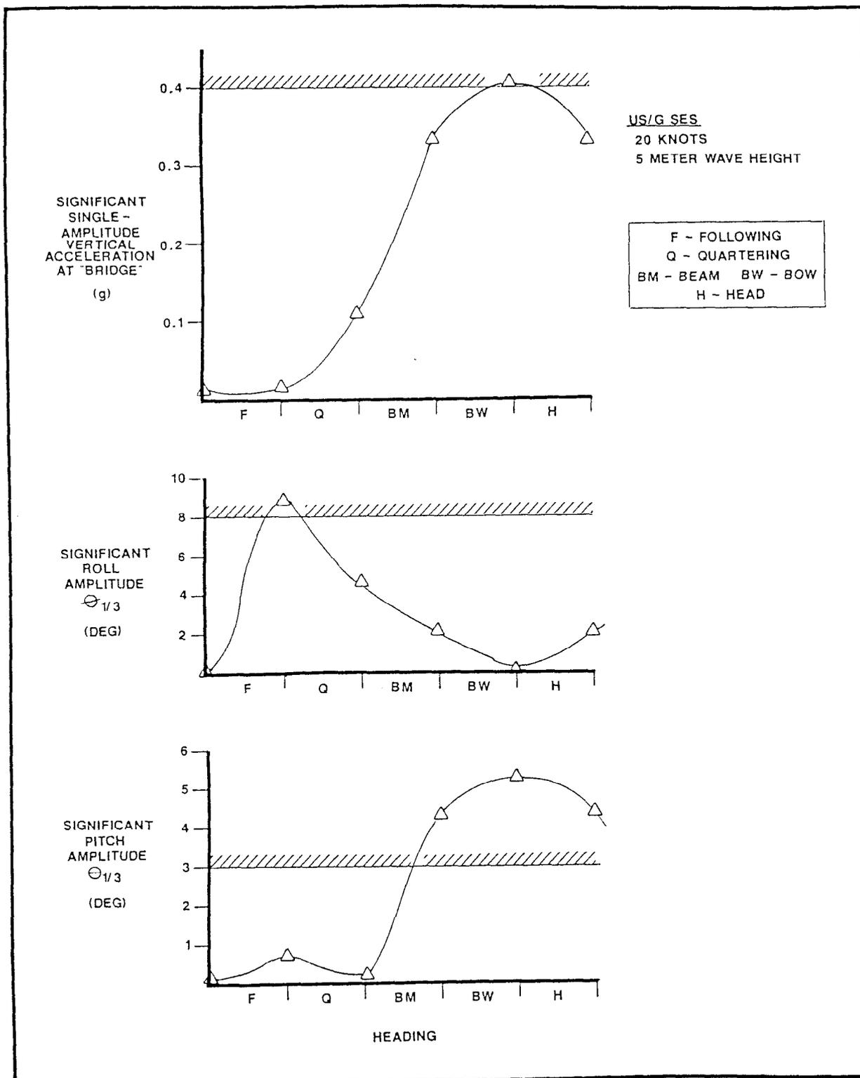
Figure 3.2.3-13. Predicted Variation of Motions and Accelerations With Heading for US/G SES at 20 Knots in 5 Meter Waves
