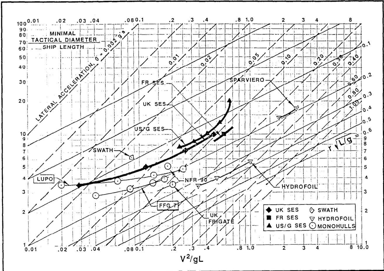
Figure 3.2.4-1. Comparisons of Maximum Non-Dimensional Maneuvering Performance in Calm Water
