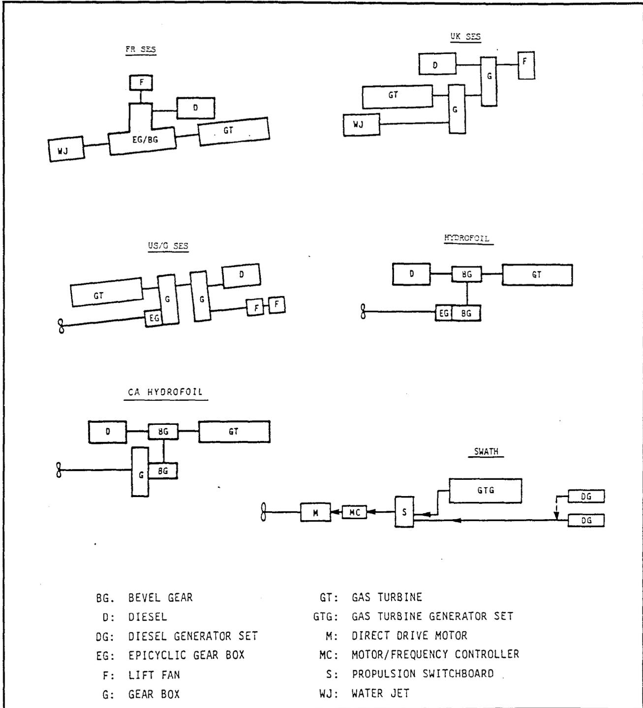
Figure 3.3.9-1. Transmission Schematics
