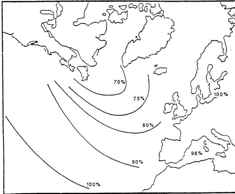
Figure 3.2.3-55. Operability Contour, Italian LUPO, 20 Knots, Active Fin Stabilizers, Winter (Ship and Helicopter Operability)
