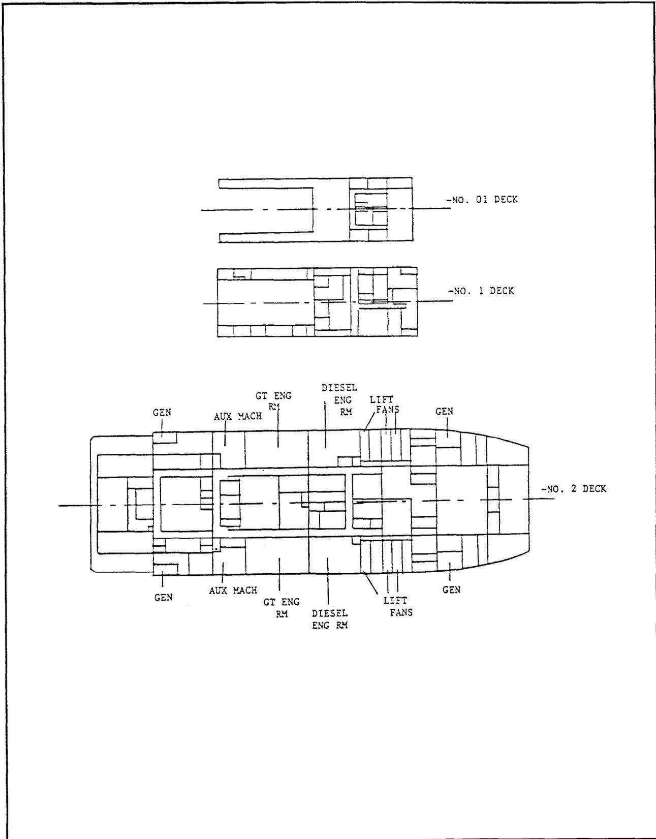
Figure 3.2.8.7-2. UK SES Machinery Arrangement (Sheet 2 of 2)
