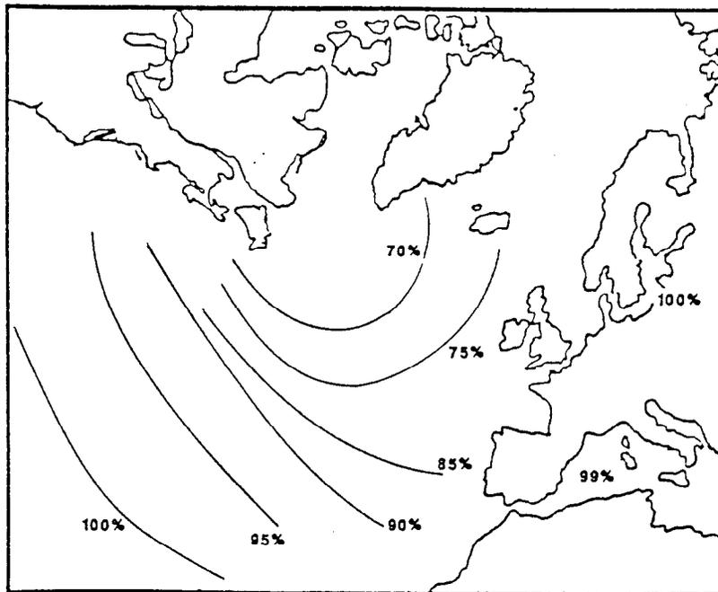
Figure 3.2.3-52. Operability Contour, UK SES, 27-40.5 Knot Range, On-Cushion Winter (Helicopter Operability)
