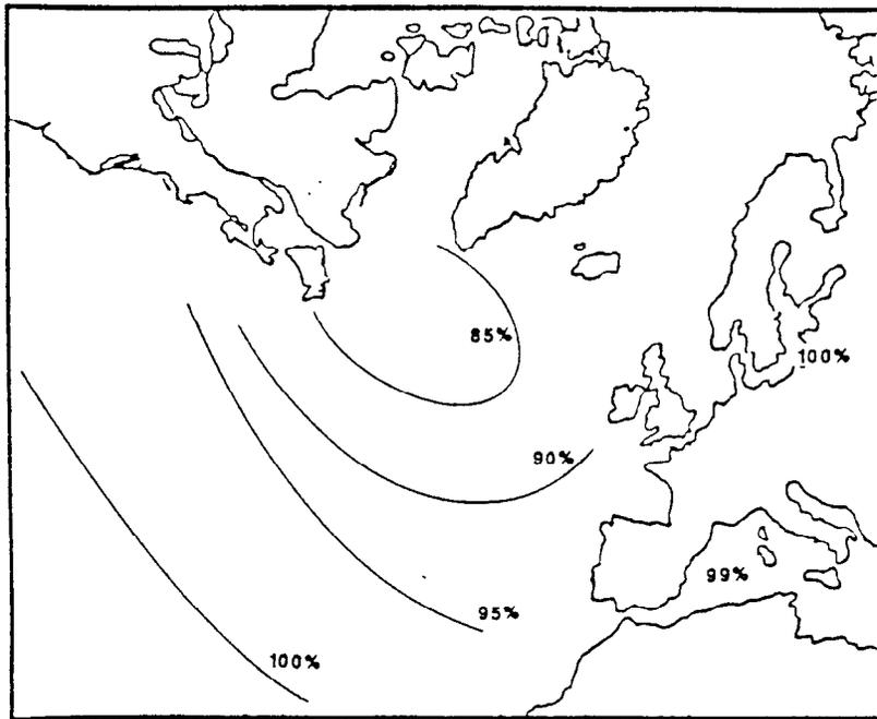
Figure 3.2.3-51. Operability Contour, UK SES, 11-17 Knot Range, Off-Cushion, Annual Average (Helicopter Operability)
