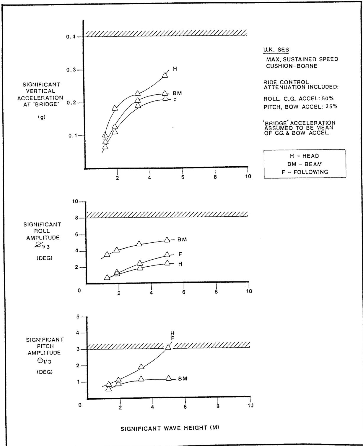
Figure 3.2.3-9. Predicted Variation of Motion and Acceleration Data With Sea State for UK SES at Maximum Sustained Speed, Cushionborne
