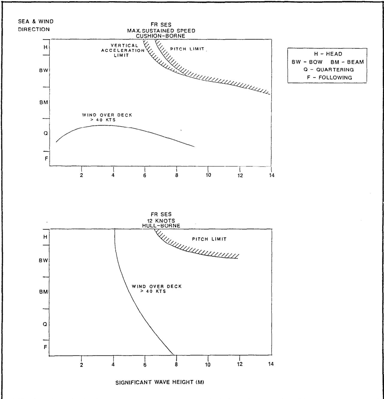
Figure 3.2.3-24. FR SES Seakeeping Limits - Effect of Wave Height and Heading
