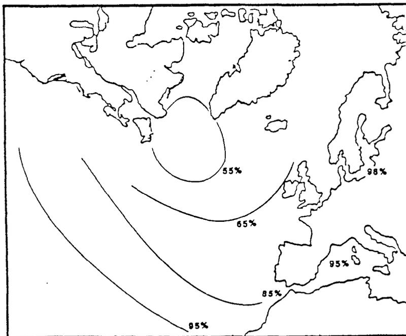
Figure 3.2.3-46. Operability Contour, NFR 90, 24-30 Knot Range, Active Fin Stabilizers, Winter (Ship Operability)
