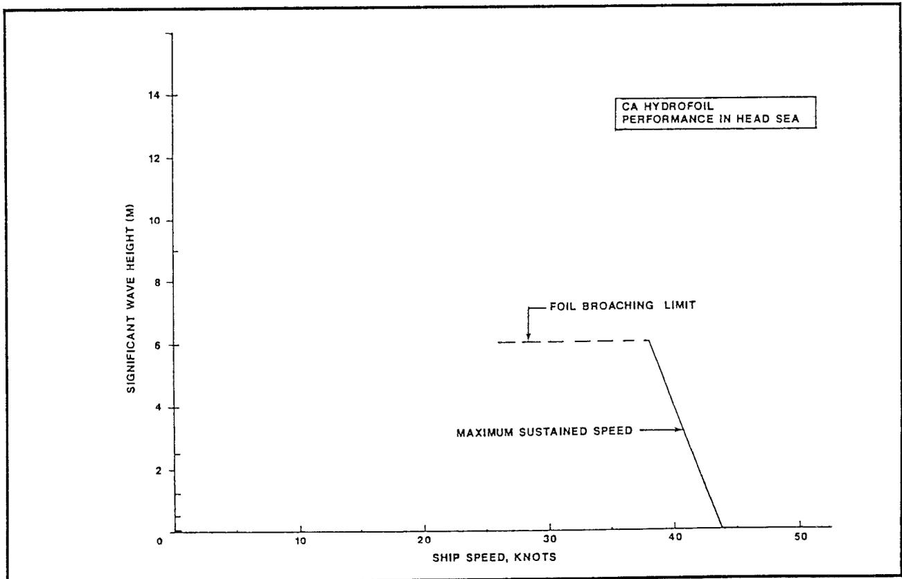
Figure 3.2.1-8. Maximum Sustained Speed Versus Sea State - CA Hydrofoil
