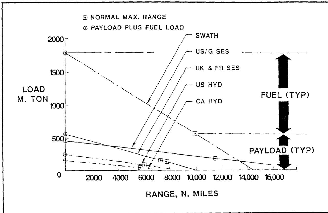
Figure 3.2.2-6. Payload - Range Trade-Off (10 Knots, Sea-State 0)
