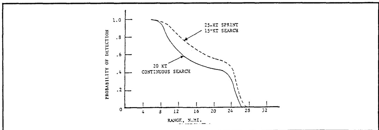
Figure 3.2.1-2. Comparison of Sprint-and-Search Mode of Operation Versus Continuous Search Mode for 20-Knot Convoy SOA.
