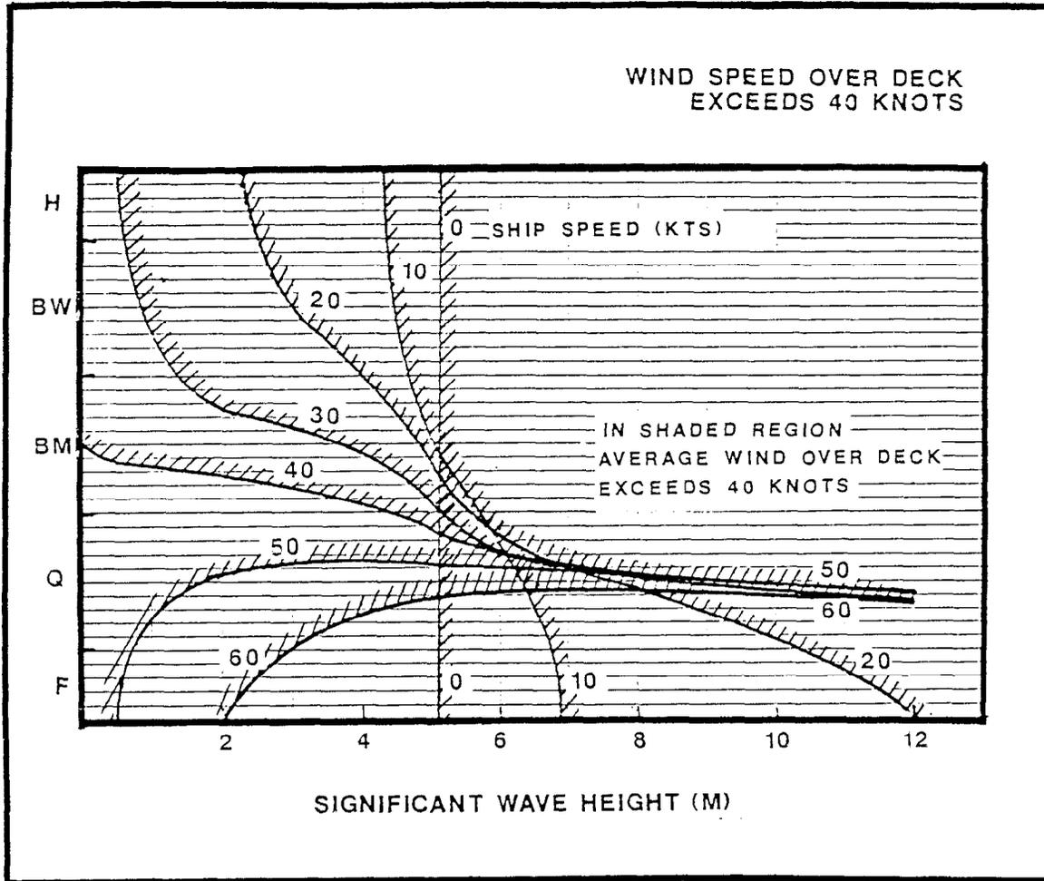
Figure 3.2.3-6. Effect of Ship Speed, Heading to Wind and Significant Wave Height on Average Relative Wind Speed
