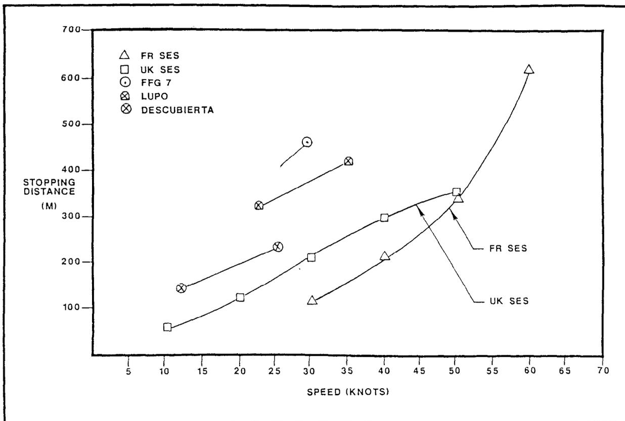
Figure 3.2.4-4. Comparison of Stopping Distance vs. Speed.
