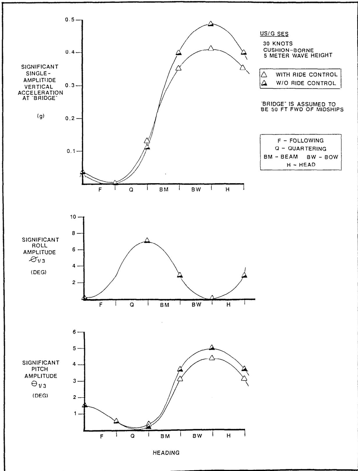
Figure 3.2.3-12. Predicted Variation of Motions and Accelerations With Heading for US/G SES at 30 Knots in 5 Meter Waves
