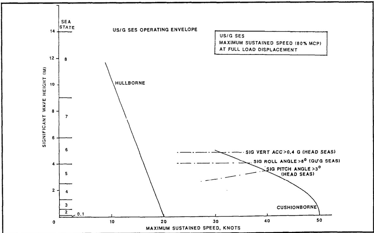
Figure 3.2.1-6. Maximum Sustained Speed Versus Sea State - US/G SES
