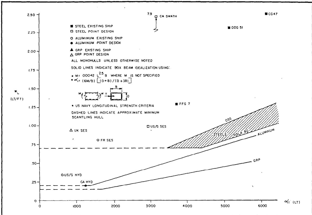
Figure 3.3.3-8. Normalized Longitudinal Structural Weight Versus Ship Size Parameter
