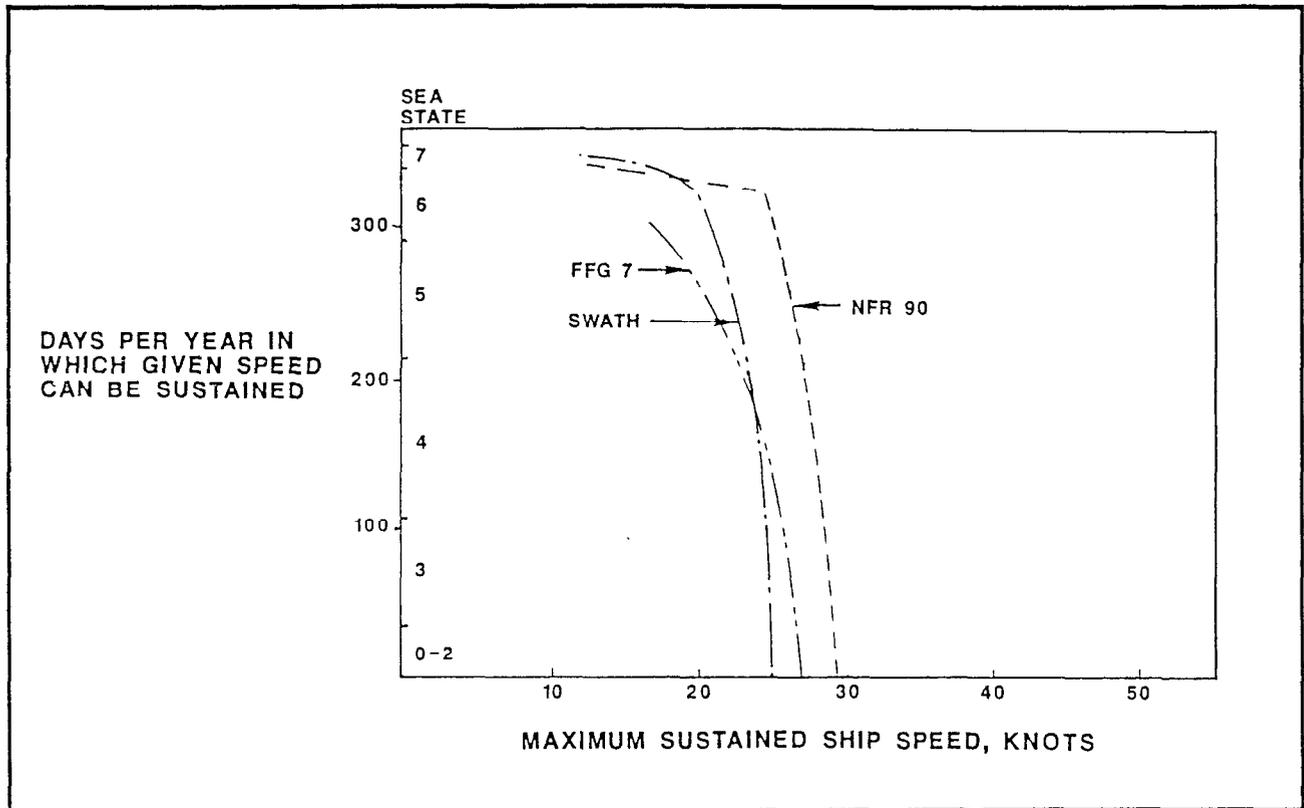
Figure 3.1.2-7. Maximum Sustained Speed Versus Sea State - SWATH in North Atlantic
