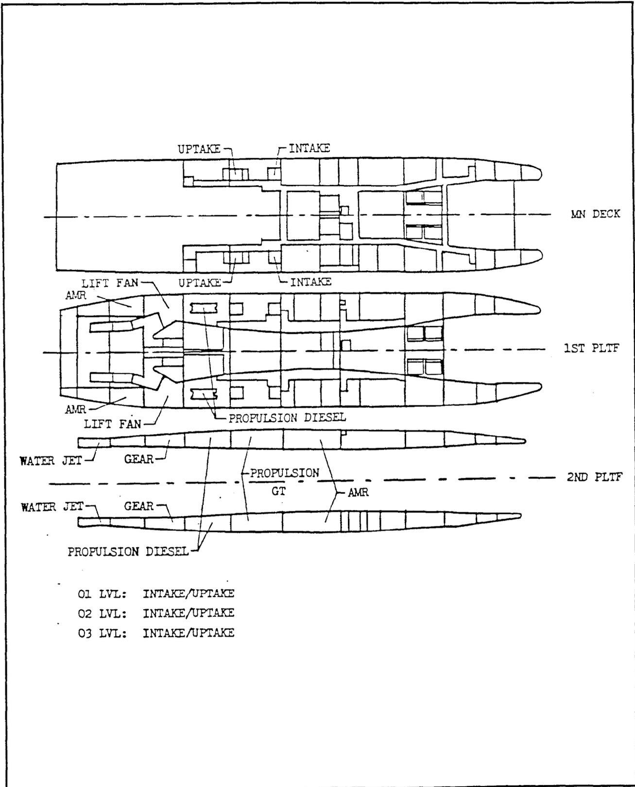
Figure 3.2.8.7-3. FR SES Machinery Arrangement (Sheet 2 of 2)
