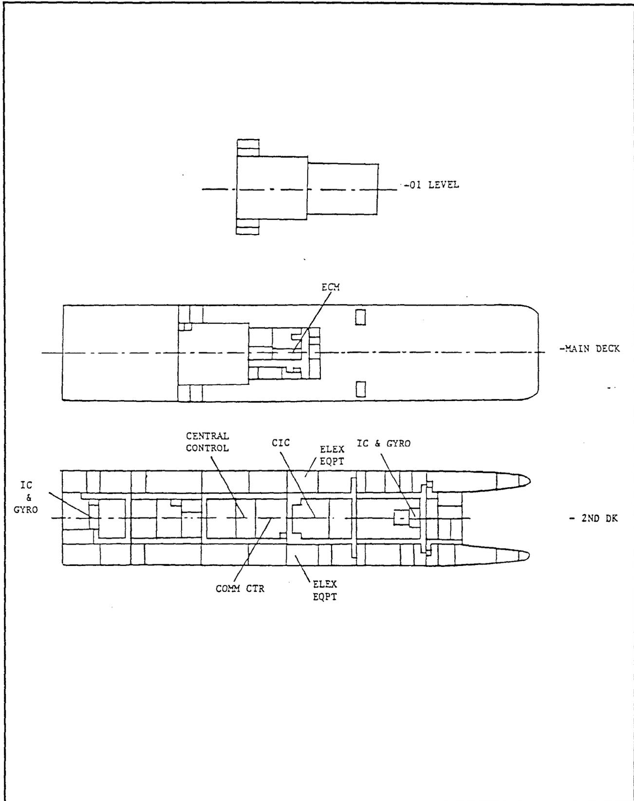
Figure 3.2.8.7-1. US/G SES C<sup>3</sup>I Space Arrangement (Sheet 1 of 2)
