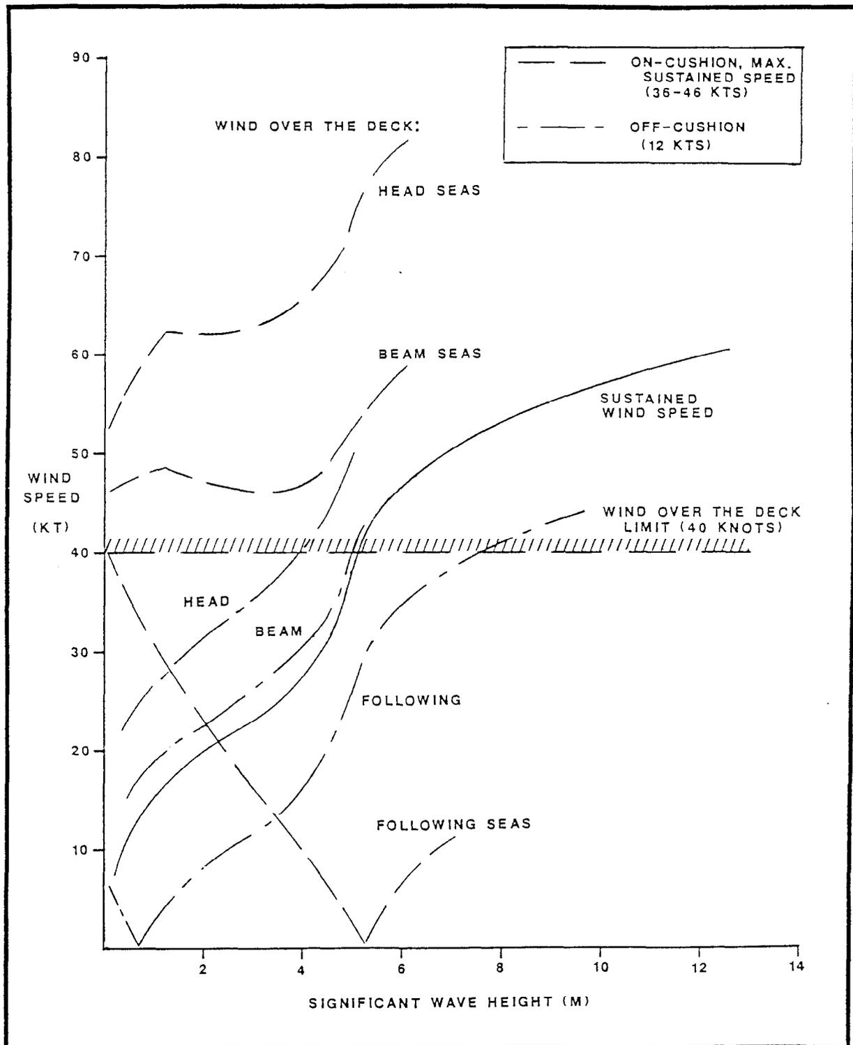
Figure 3.2.3-5. Average Relative Speed Over the Deck for an SES at Maximum Sustained Speed and at 12 Knots as a Function of Wave Height.
