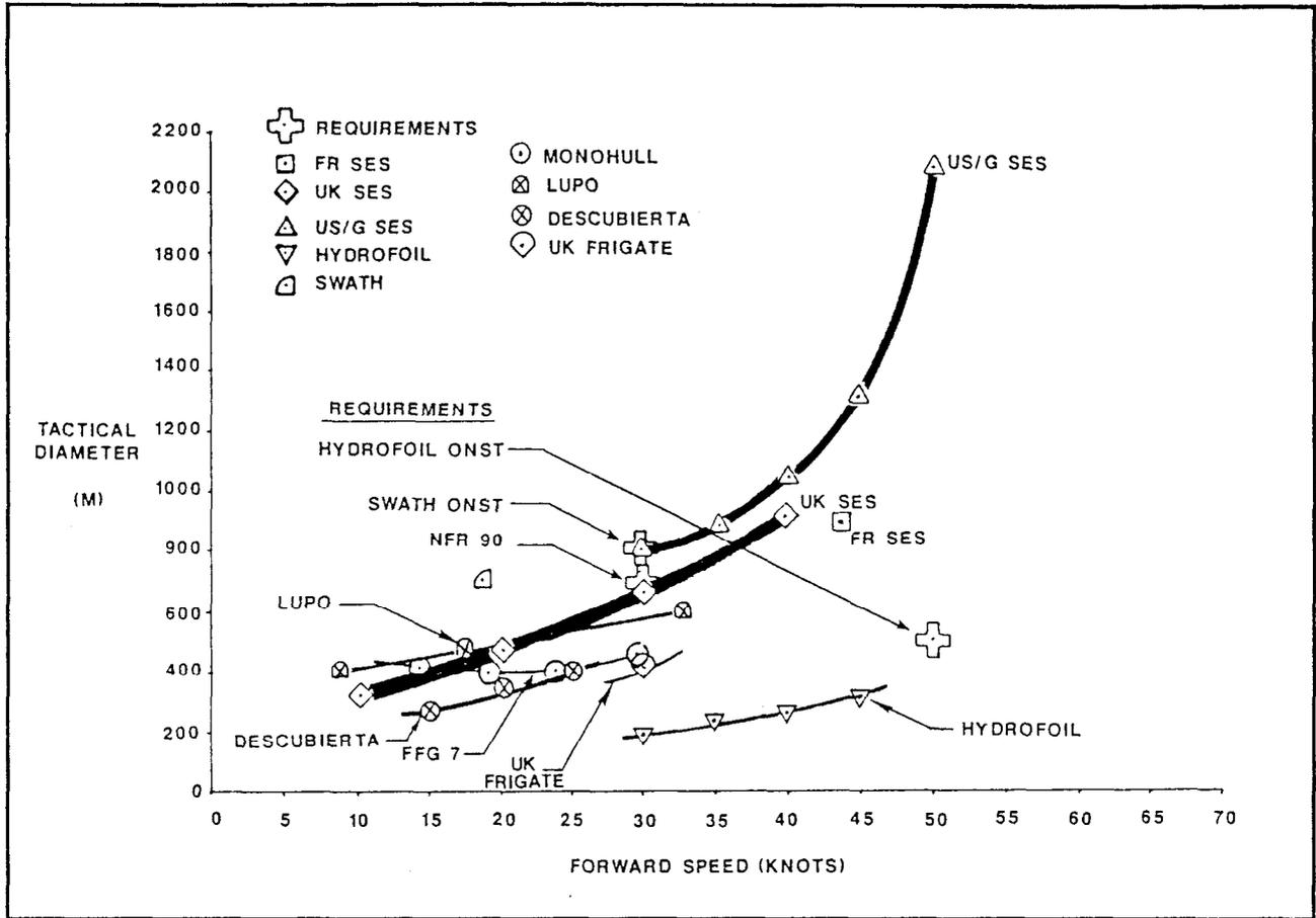
Figure 3.2.4-2. Tactical Diameter Versus Forward Speed in Calm Water
