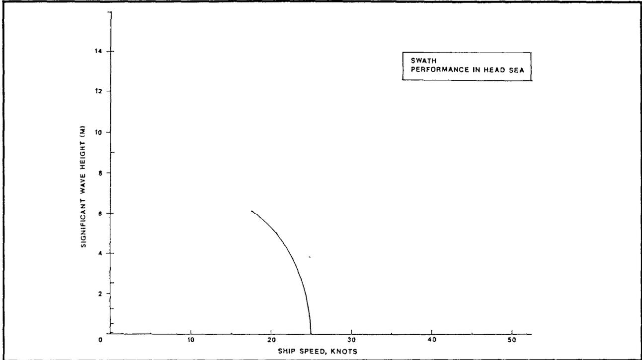
Figure 3.2.1-9. Maximum Sustained Speed Versus Sea State - SWATH
