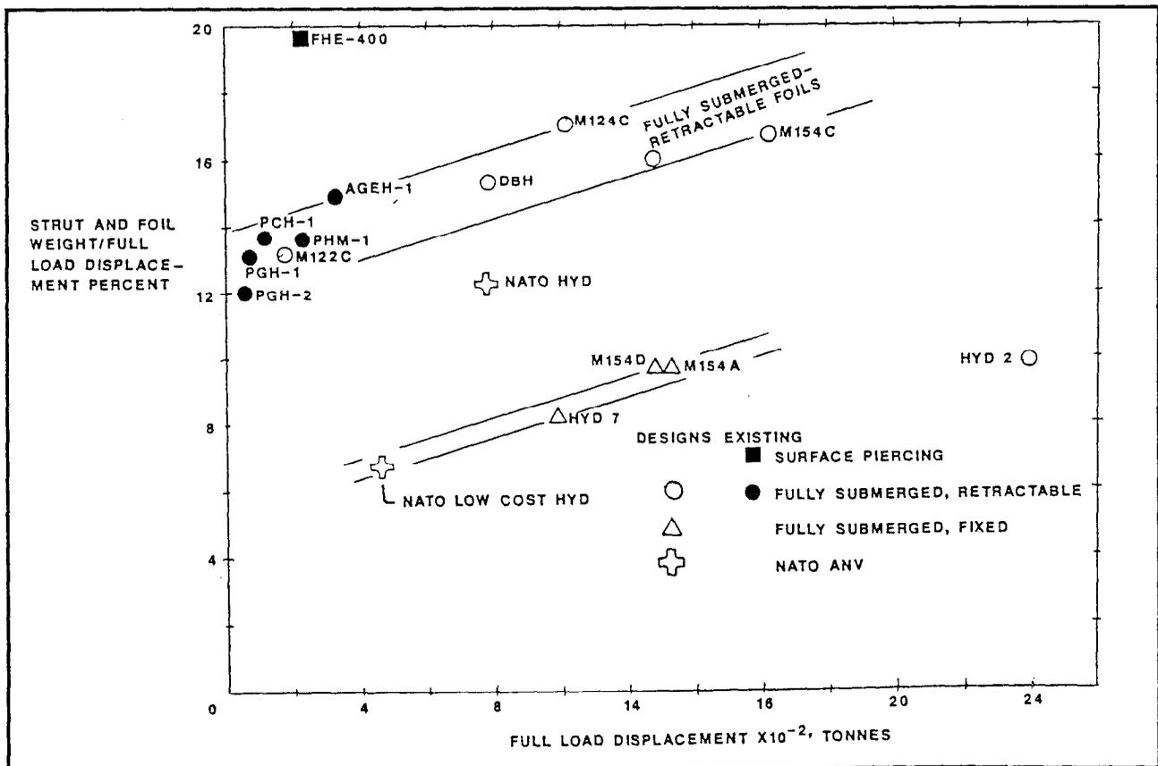
Figure 3.3.13-2. Comparison of Hydrofoil Lift-System Weight
