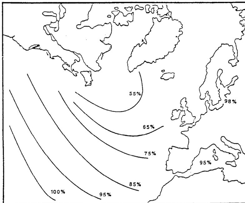
Figure 3.2.3-56. Operability Contour, Italian LUPO, 28 Knots, Active Fin Stabilizers, Winter (Ship and Helicopter Operability)
