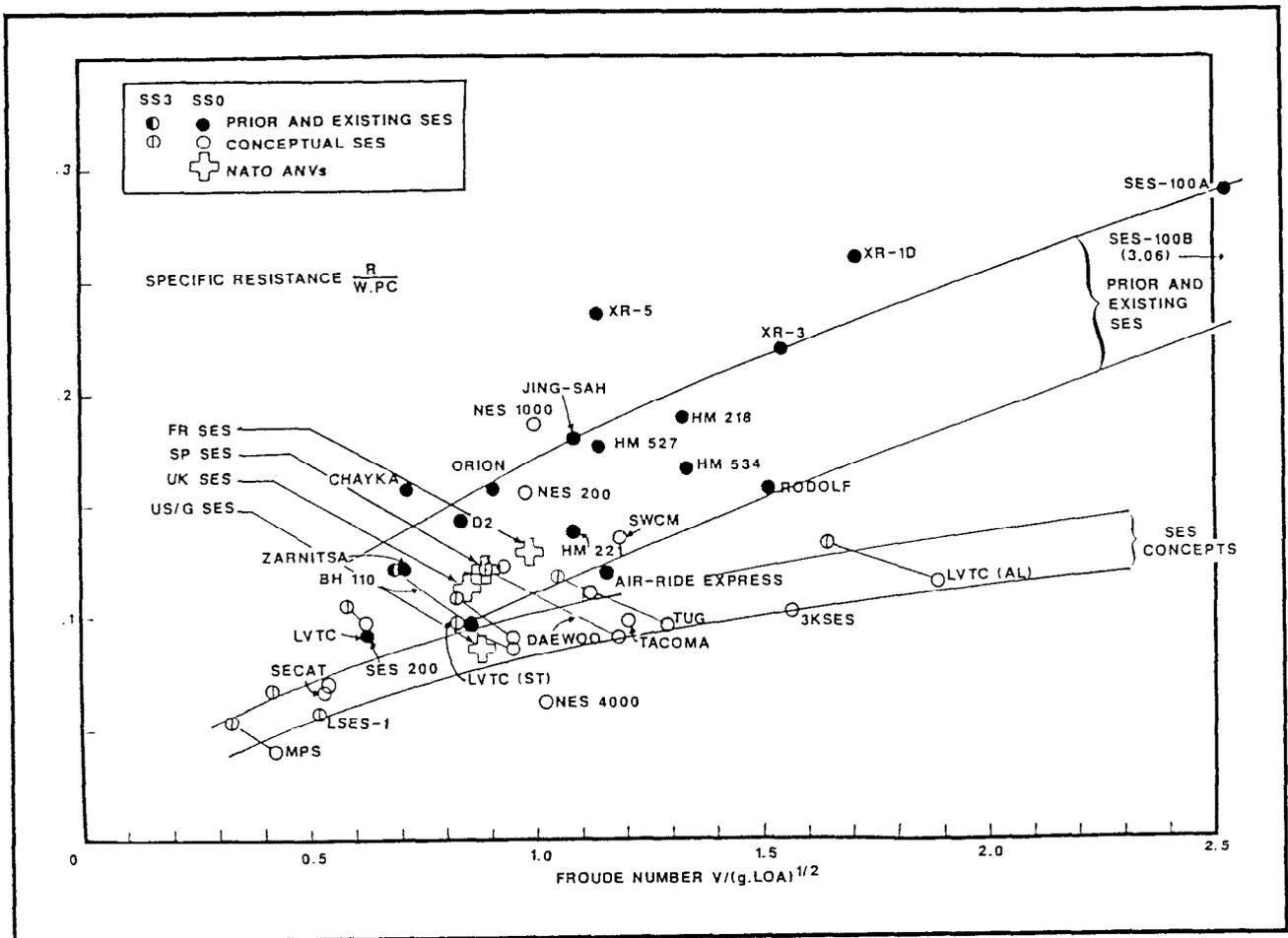
Figure 3.3.5-14. Specific Resistance for Prior, Existing and Conceptual SES in the High-Speed, On-Cushion Mode of Operation
