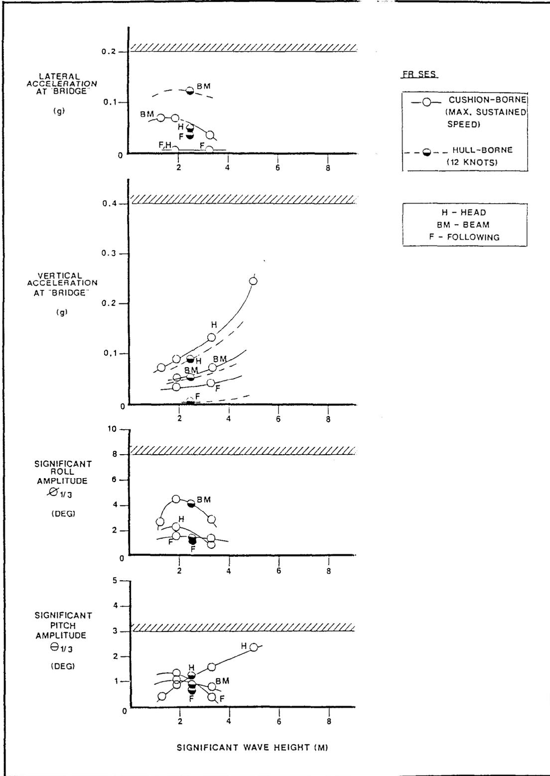
Figure 3.2.3-10. Predicted Variation of Motion and Acceleration Due to Significant Wave Heights for the FR SES and Maximum Sustained Speed
