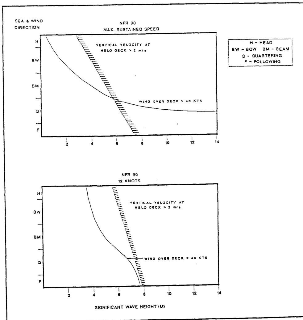
Figure 3.2.3-31. Estimated NFR 90 Seakeeping Limits - Effect of Sea State and Heading
