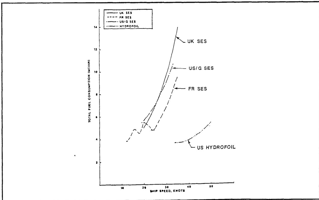
Figure 3.2.2-4. Fuel Consumption Versus Ship Speed - High-Speed, Cushion or Foilborne Mode in Sea State 6
