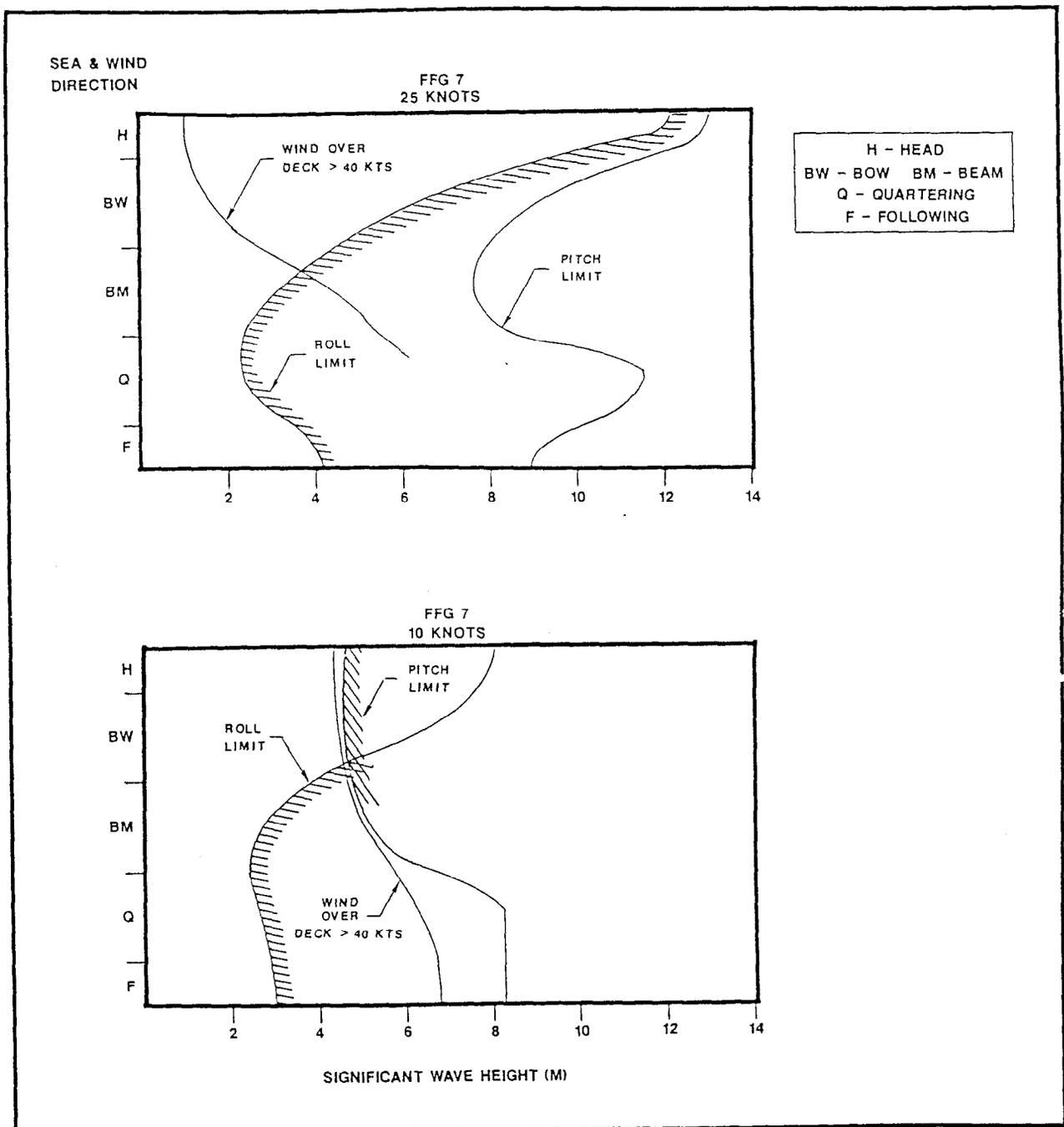
Figure 3.2.3-29. FFG-7 Seakeeping Limits
