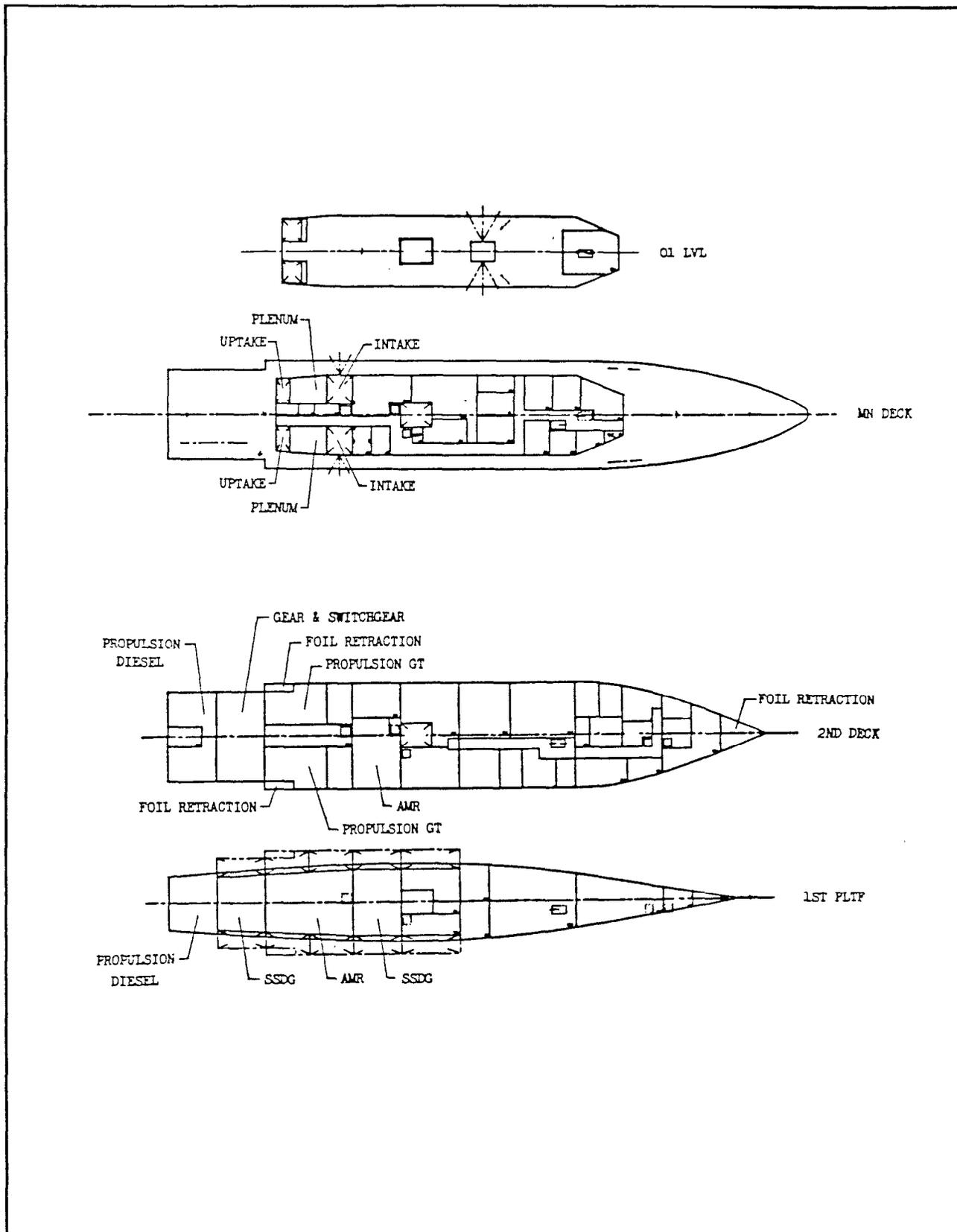
Figure 3.2.8.7-4. US Hydrofoil Machinery Arrangement (Sheet 2 of 2)
