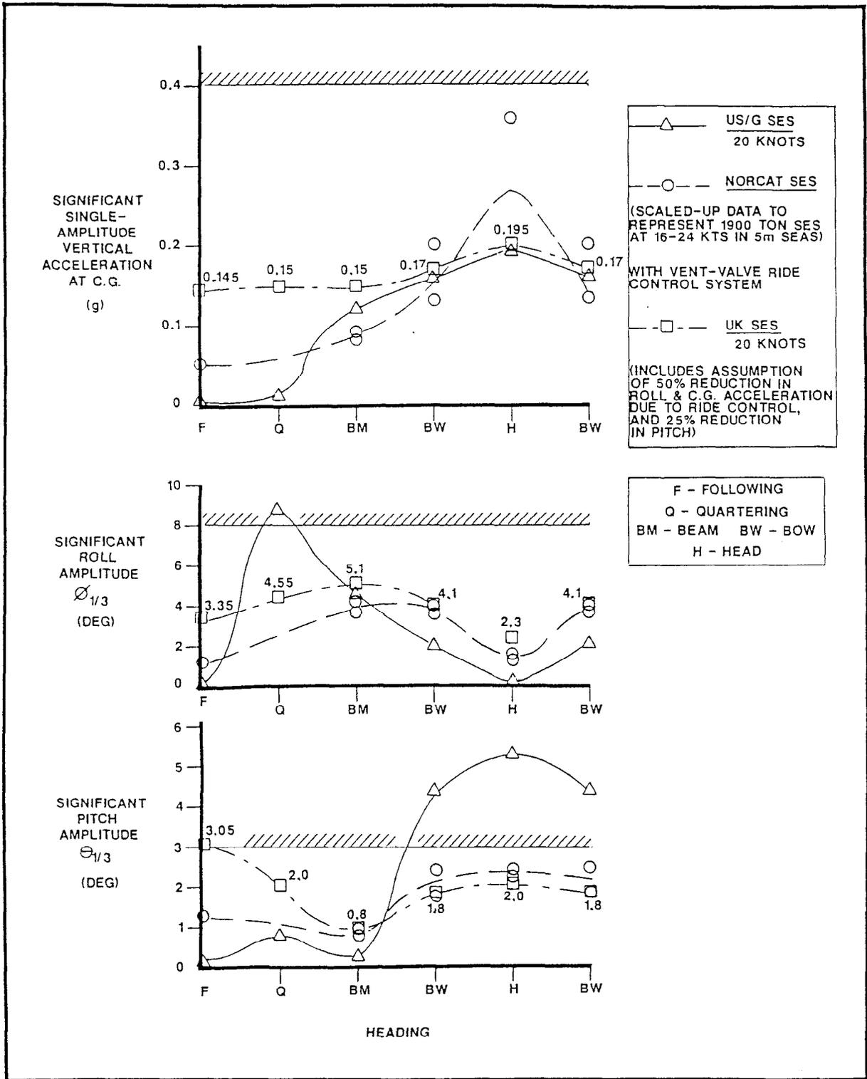
Figure 3.2.3-15. Comparison of Motions and Acceleration for UK SES, US/G SES and NORCAT
