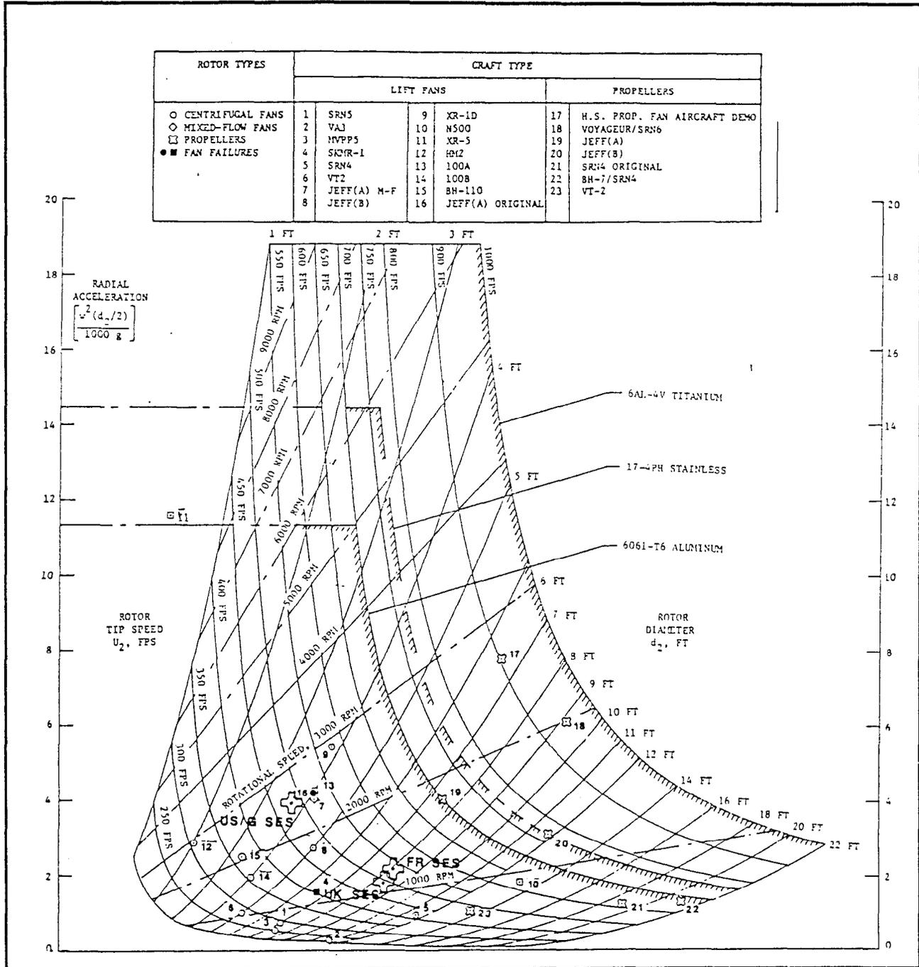
Figure 3.3.7-5. Lift-Fan Rotor Speed Limitations
