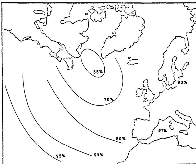
Figure 3.2.3-36. Operability Contour, FR SES, 12-18 Knot Range, Off-Cushion, Winter, (Ship Operability)
