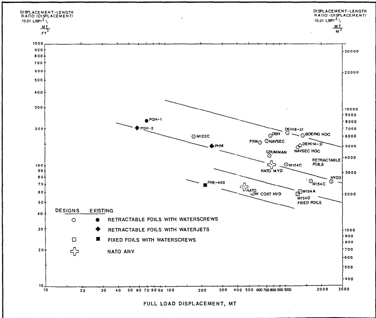
Figure 3.3.13-1. Displacement-Length Ratio for Hydrofoil Craft
