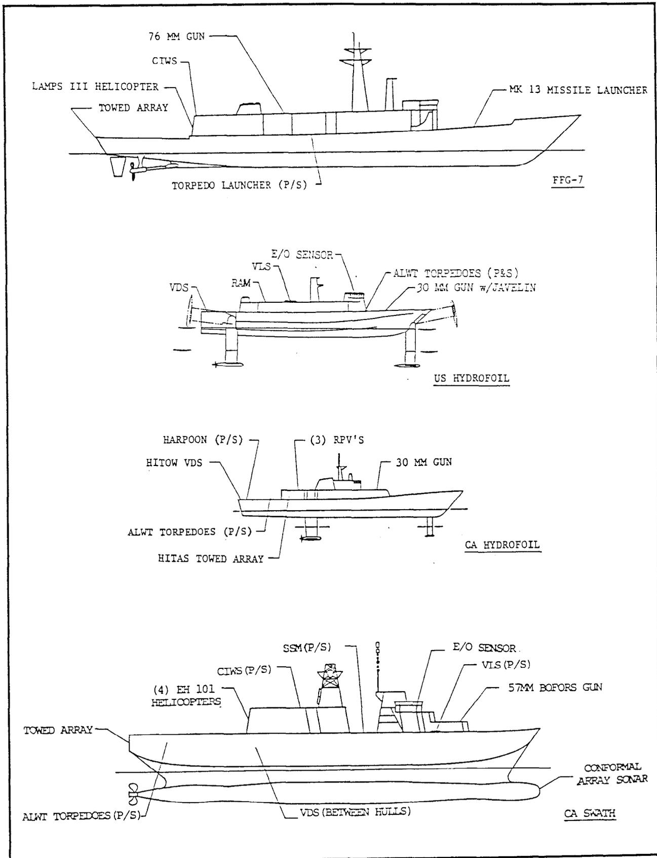
Figure 3.2.6-2. Combat Systems Arrangements Profile View (Sheet 2 of 2)
