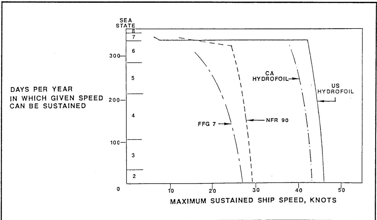
Figure 3.1.2-6. Maximum Sustained Speed Versus Sea State - Hydrofoil in North Atlantic
