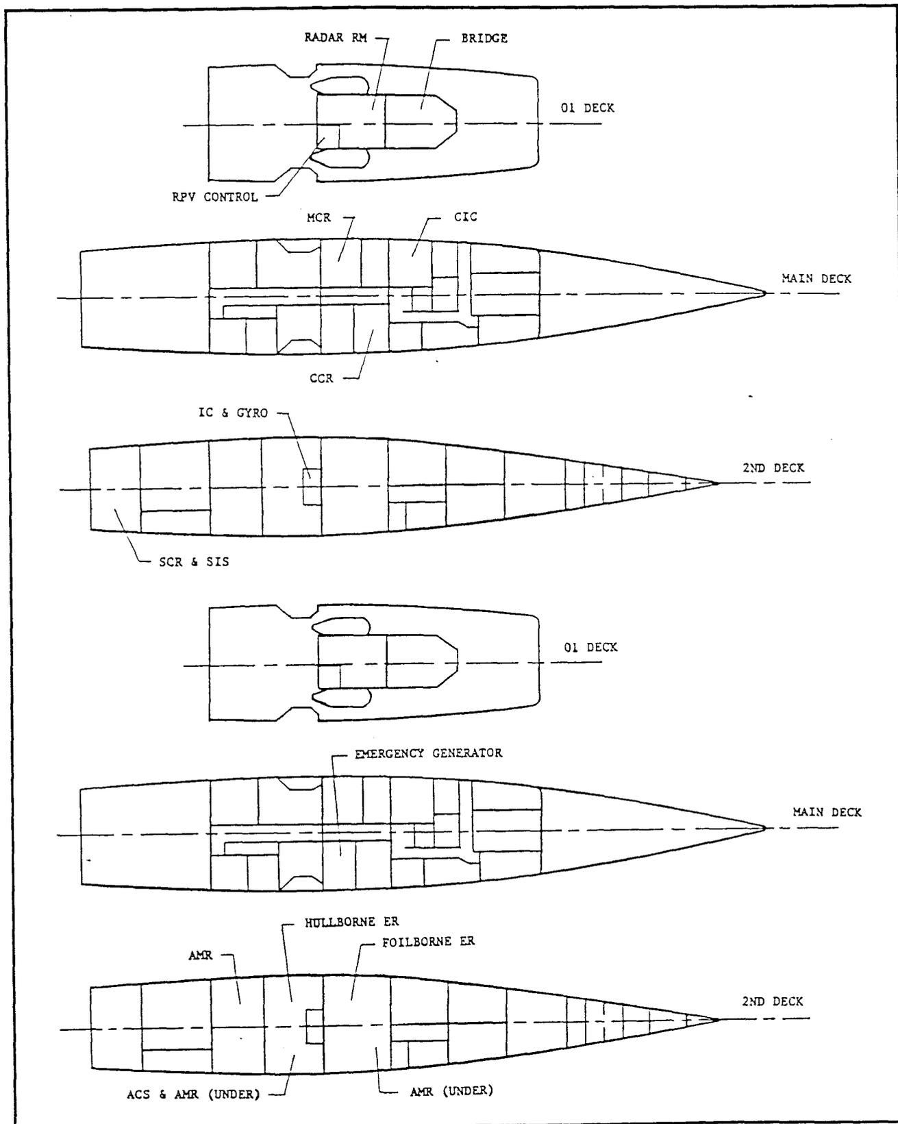
Figure 3.2.8.7-5. CA Hydrofoil C<sup>3</sup>I Space Arrangements
