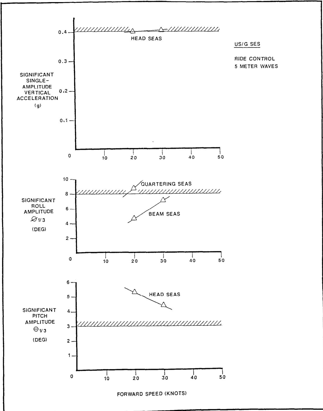
Figure 3.2.3-11. Predicted Variation of Motions and Accelerations With Forward Speed and Heading for US/G SES (With Ride Control)
