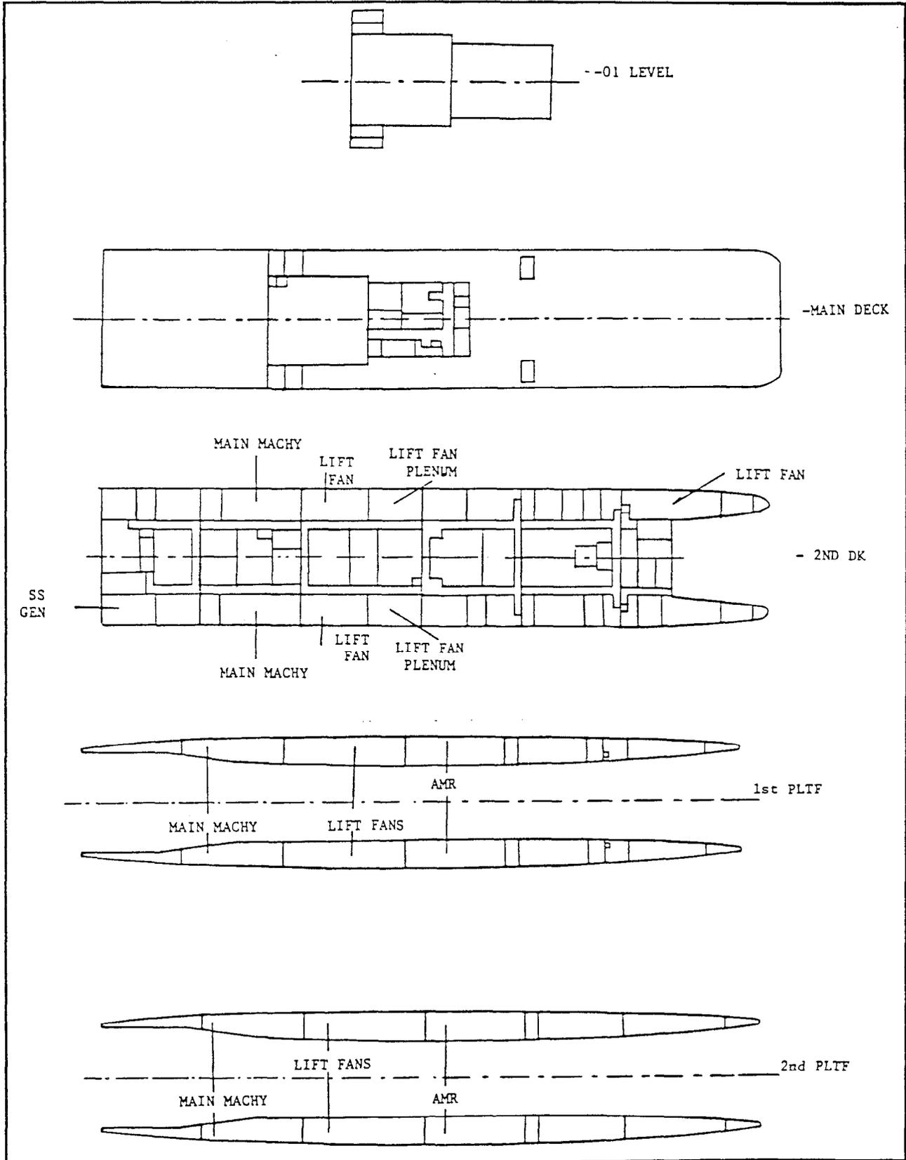
Figure 3.2.8.7-1. US/G SES Machinery Arrangement (Sheet 2 of 2)
