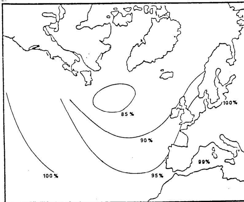
Figure 3.2.3-34. Operability Contour, UK SES 11-17 Knot Range, Off-Cushion, Winter (Ship Operability)
