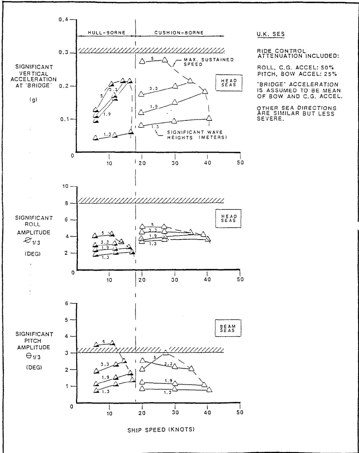
Figure 3.2.3-7. Predicted Variation of Motions and Accelerations With Sea State and Ship Speed for UK SES
