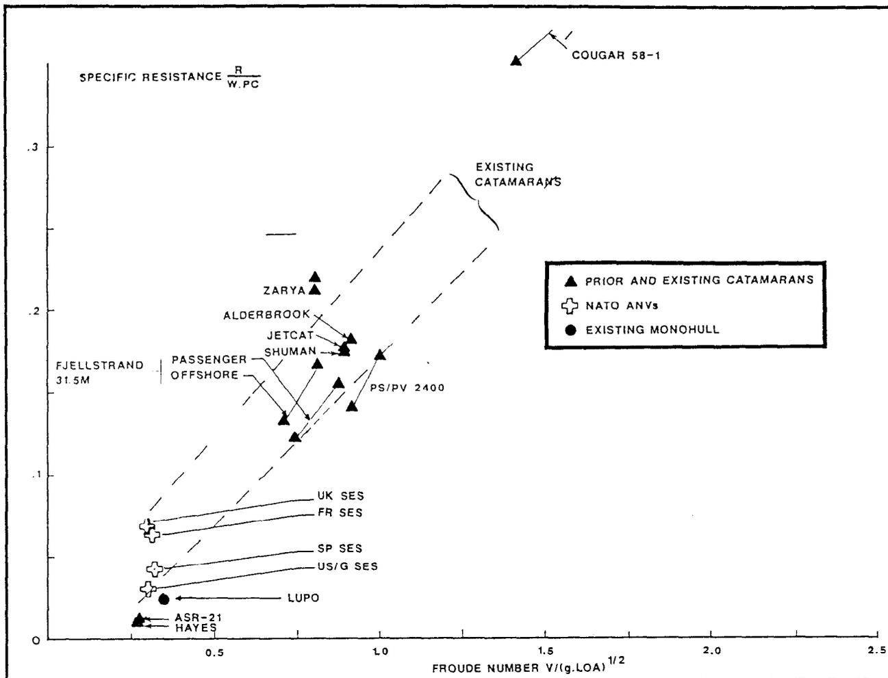
Figure 3.3.5-12. Specific Resistance for Prior, Existing and Conceptual SES Operating in the Hullborne Mode and for Catamarans
