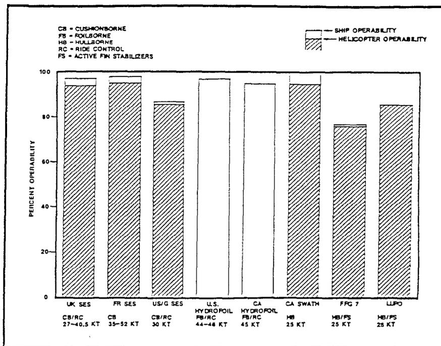
Figure 3.2.3-58. Comparison of Percentage Operabilities of ASW Ships at High Speed in the North Sea in Winter
