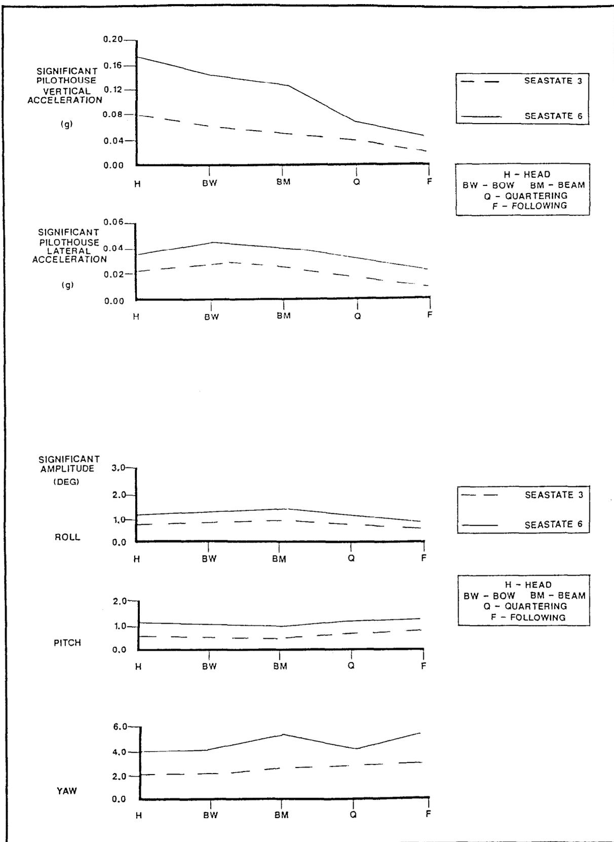
Figure 3.2.3-16. U.S. Hydrofoil Foilborne Motions and Accelerations as a Function of Heading
