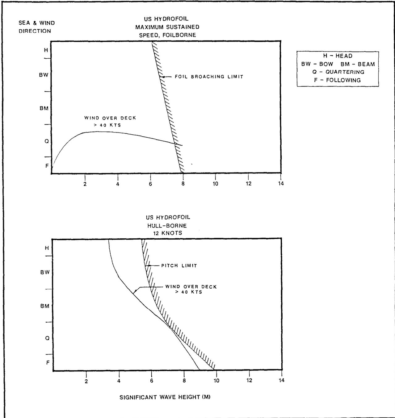
Figure 3.2.3-26. U.S. Hydrofoil Seakeeping Limits - Effect of Wave Height and Heading
