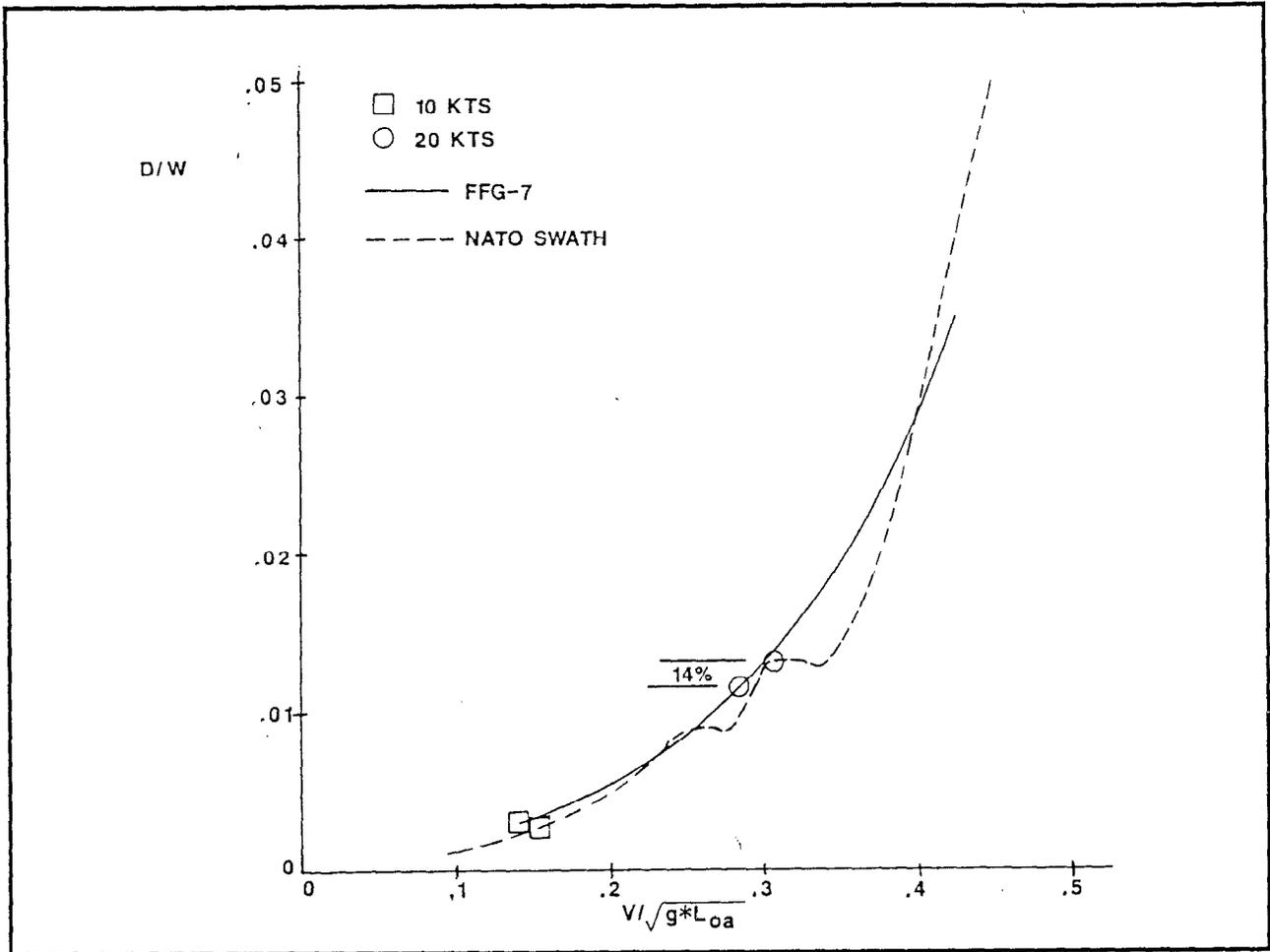
Figure 3.3.5-16. Comparison of NATO SWATH and FFG 7 Non-Dimensional Drag in Calm Water
