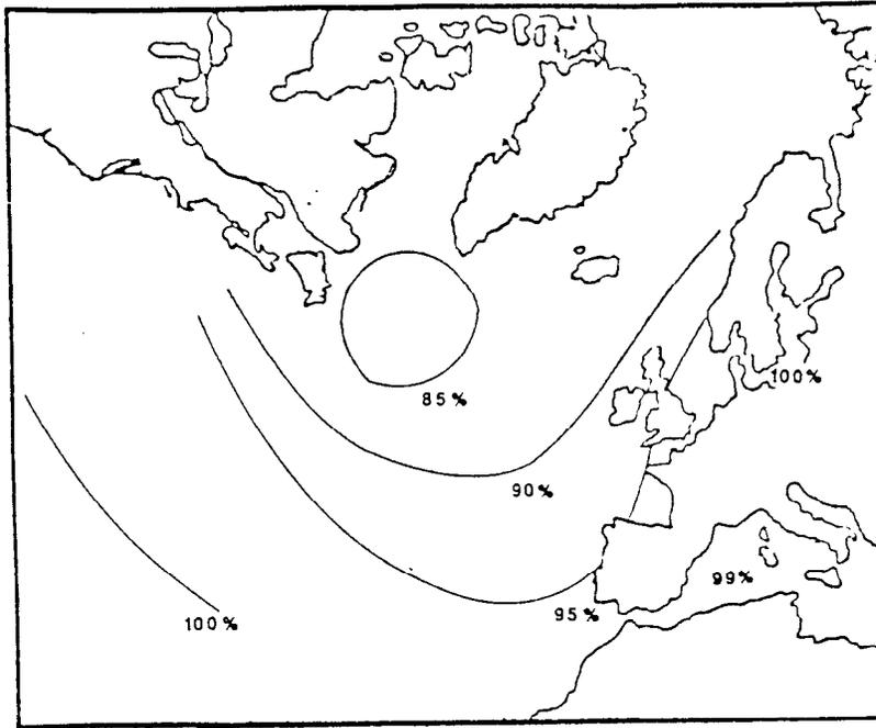
Figure 3.2.3-33. Operability Contour, UK SES, 27-40.5 Knot Range, Ride-Control, On-Cushion, Winter (Ship Operability)
