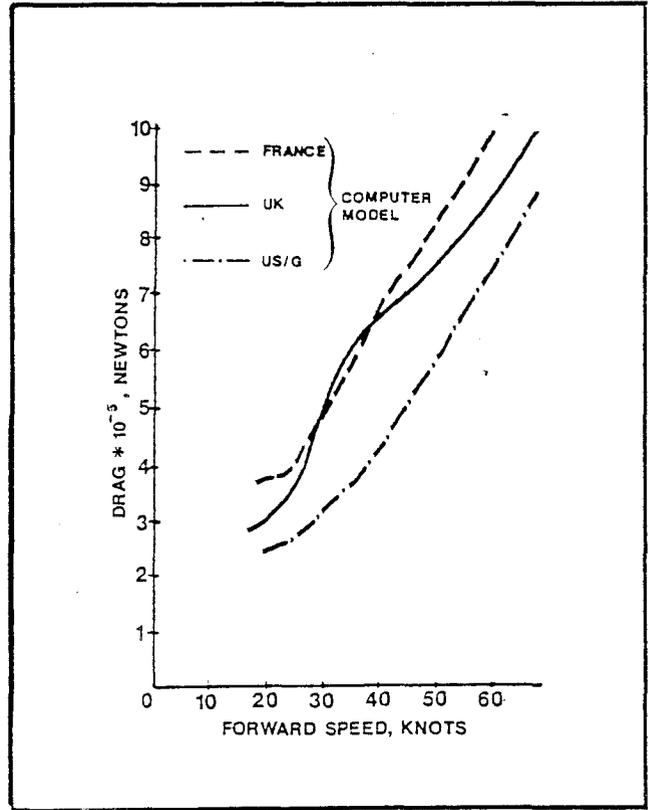
Figure 3.3.5-5. Comparison of Predicted Drag of SES Point Designs at Comparable Weights
