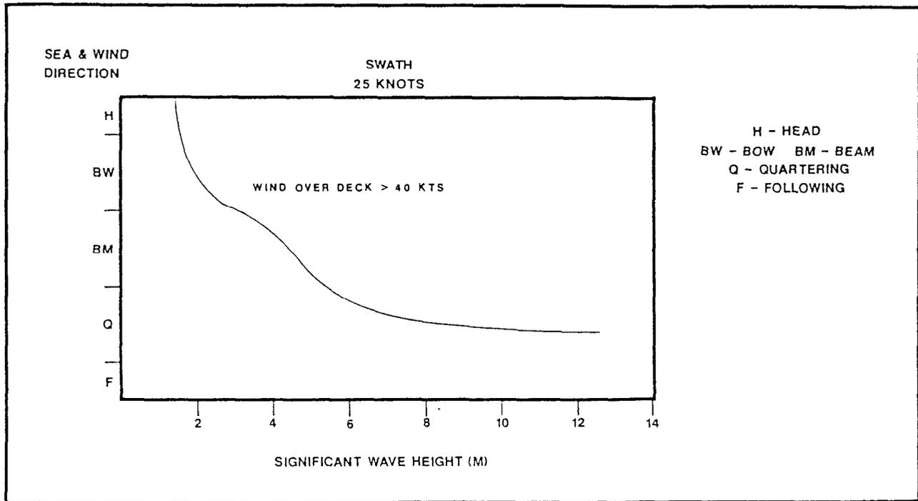
Figure 3.2.3-28. SWATH Seakeeping Limits
