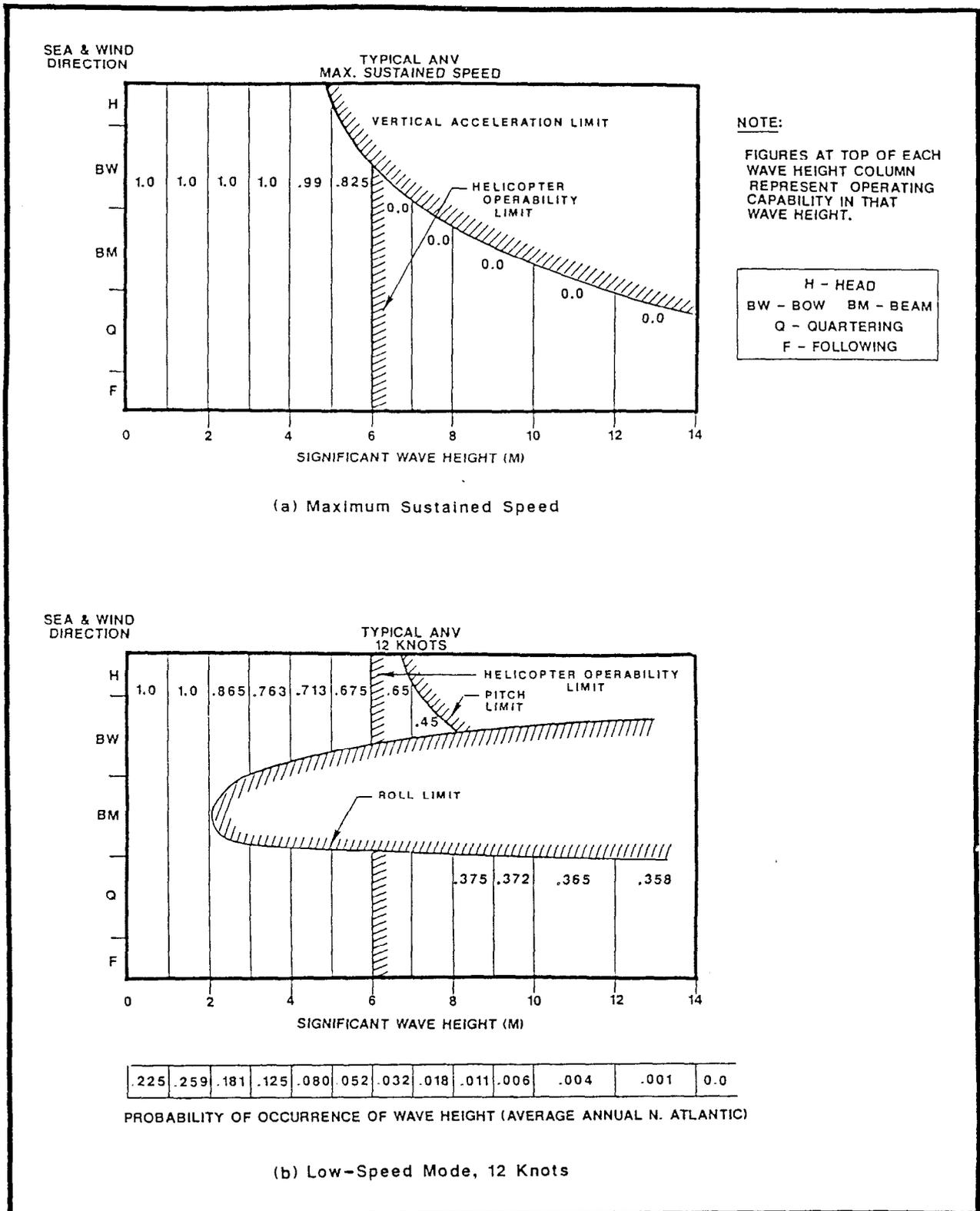
Figure 3.2.3-32. Zones of Unrestricted Operational Capabilities for Typical ANV
