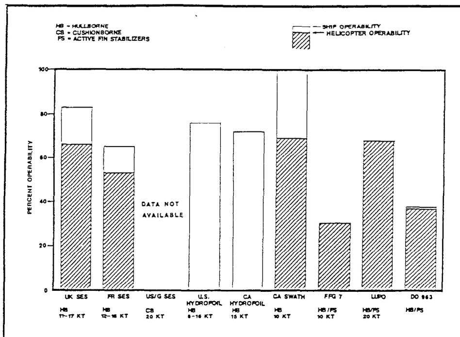
Figure 3.2.3-60. Comparison of Percentage Operabilities of ASW Ships at Low Speed in the Northern North Atlantic in Winter
