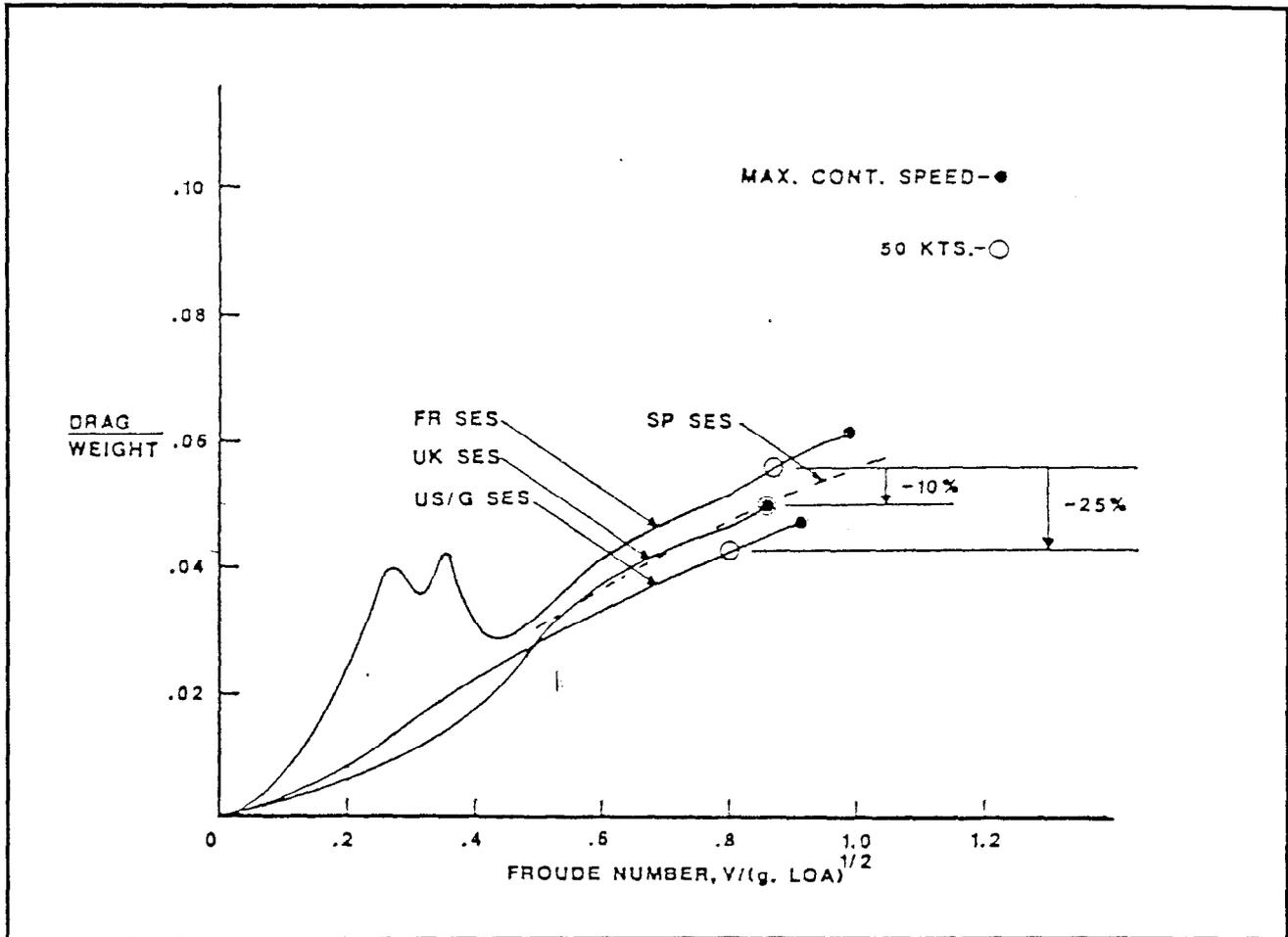
Figure 3.3.5-1. Comparison of SES On-Cushion Drag in Sea-State 0.
