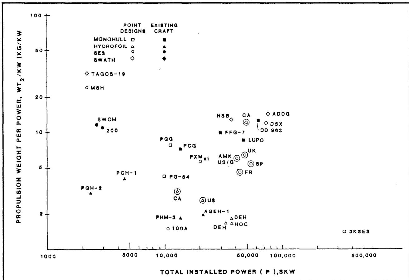
Figure 3.3.18-4. Propulsion System Weight Per Installed Horsepower
