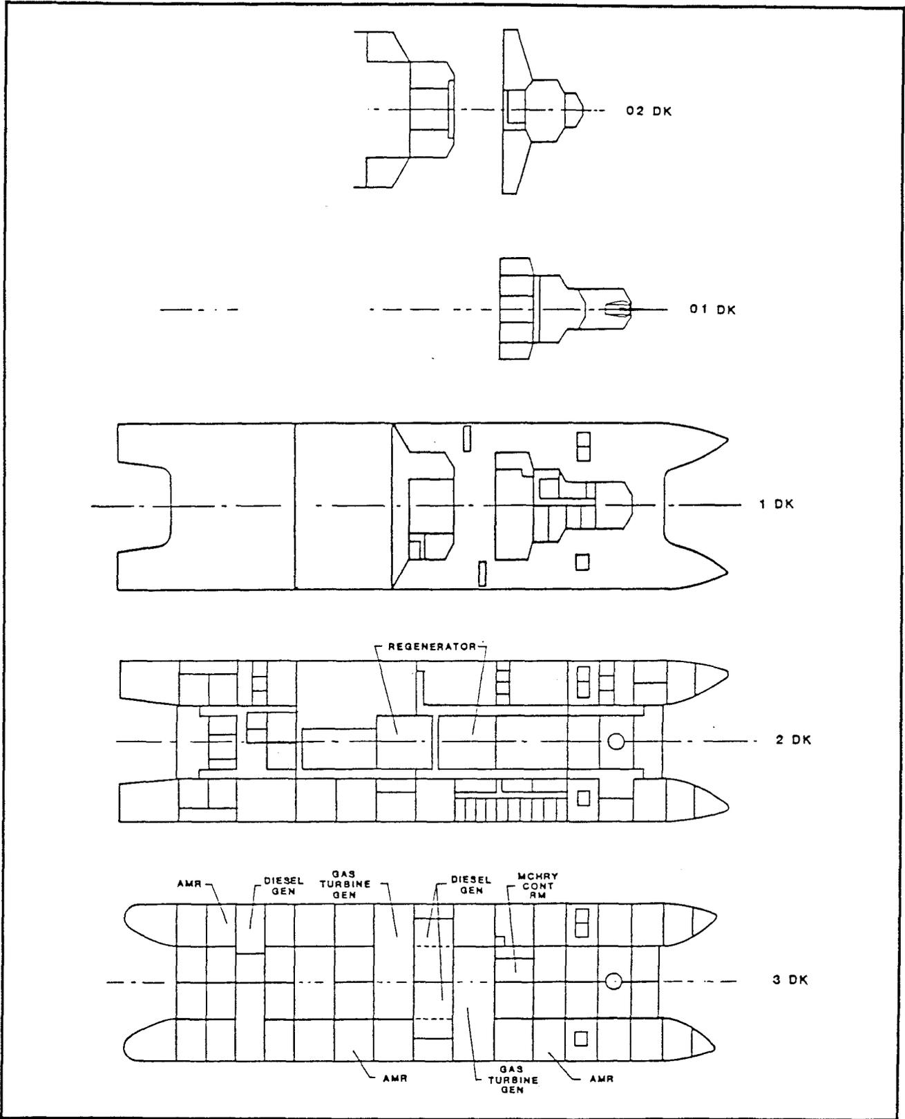
Figure 3.2.8.7-6. SWATH Machinery Arrangements (Sheet 3 of 4)
