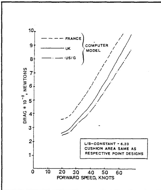
Figure 3.3.5-8. Comparison of Predicted Drag of High L/B Versions of SES Point Designs at Comparable Weights
