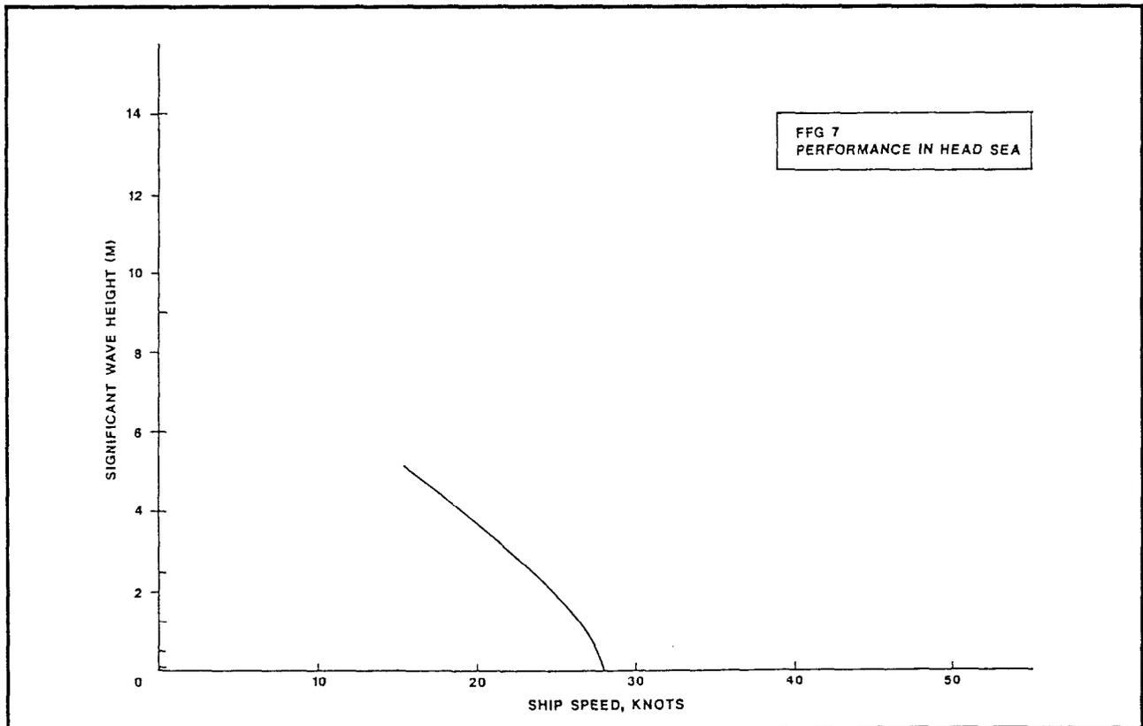
Figure 3.2.1-10. Maximum Sustained Speed Versus Sea State FFG 7
