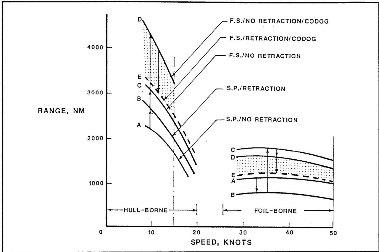
Figure 3.2.2-7. Trade-Off Results Showing Range as a Function of Speed for Various Hydrofoil Configurations
