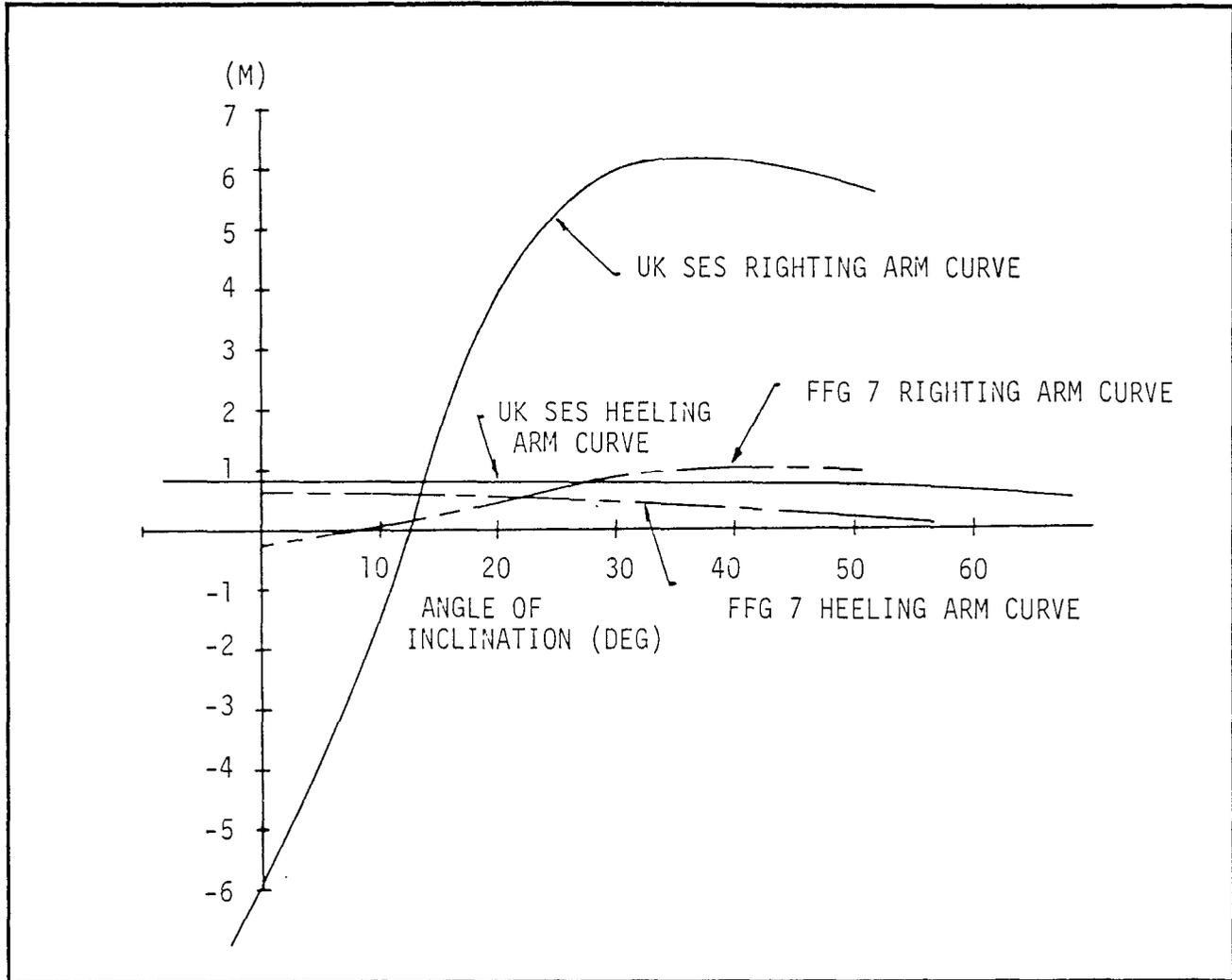
Figure 3.3.21-3. Worst-Case Damage Curves of Stability
