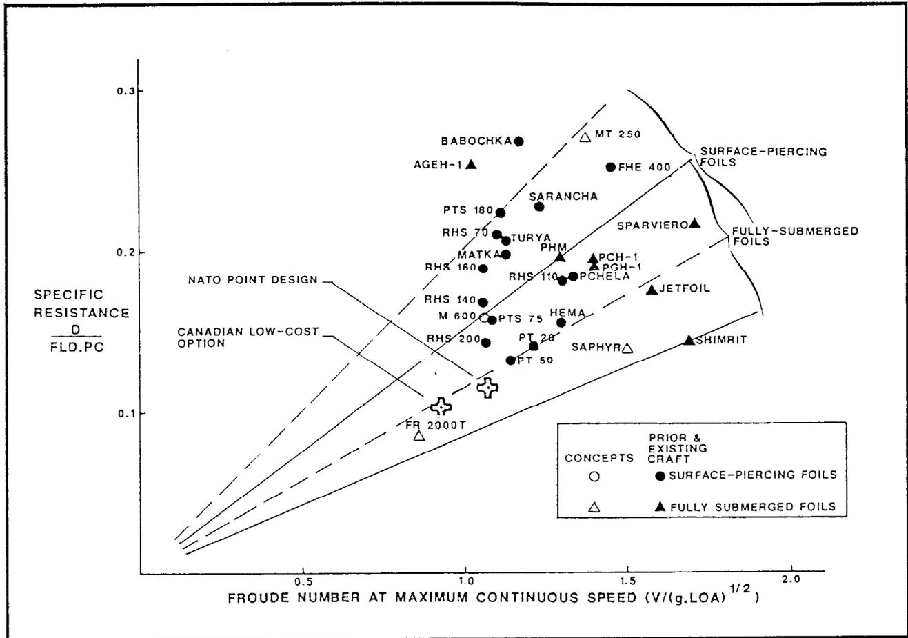
Figure 3.3.5-15. Specific Resistance of Hydrofoil Craft
