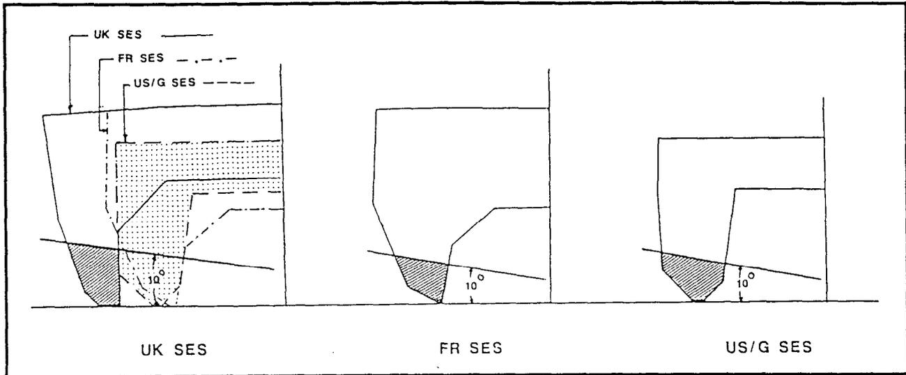
Figure 3.3.21-4. Comparison of Sidehull Cross-Sections
