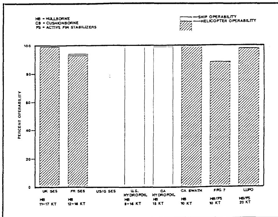
Figure 3.2.3-62. Comparison of Percentage Operabilities of ASW Ships at Low Speed in the Mediterranean in Winter
