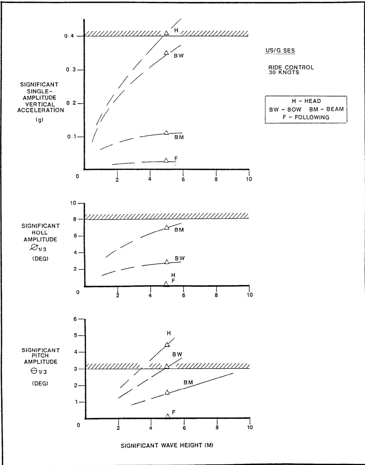
Figure 3.2.3-14. Predicted Variation of Motions and Accelerations With Significant Wave Height for US/G SES at 30 Knots
