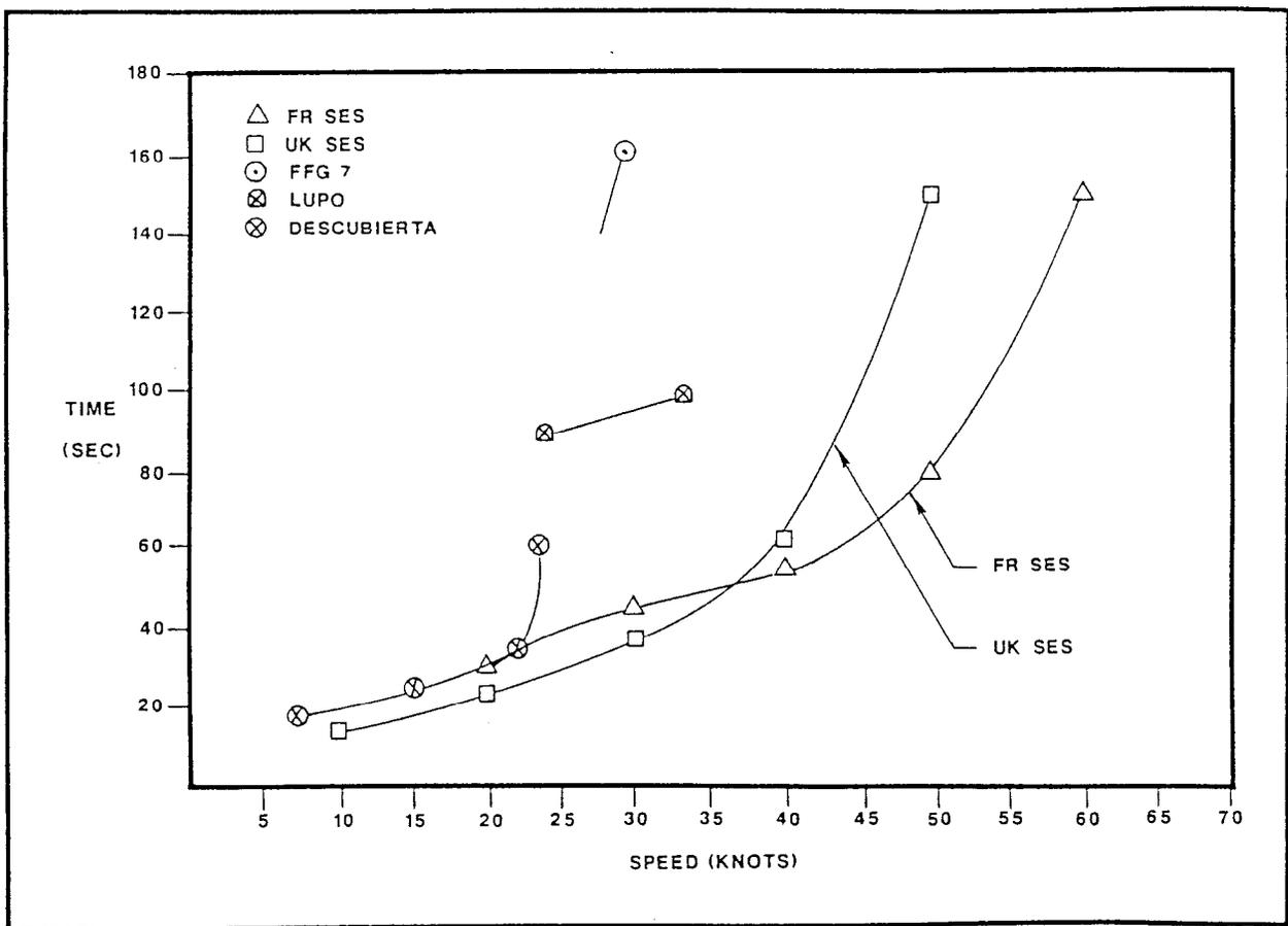
Figure 3.2.4-3. Comparison of Time of Acceleration to Speed
