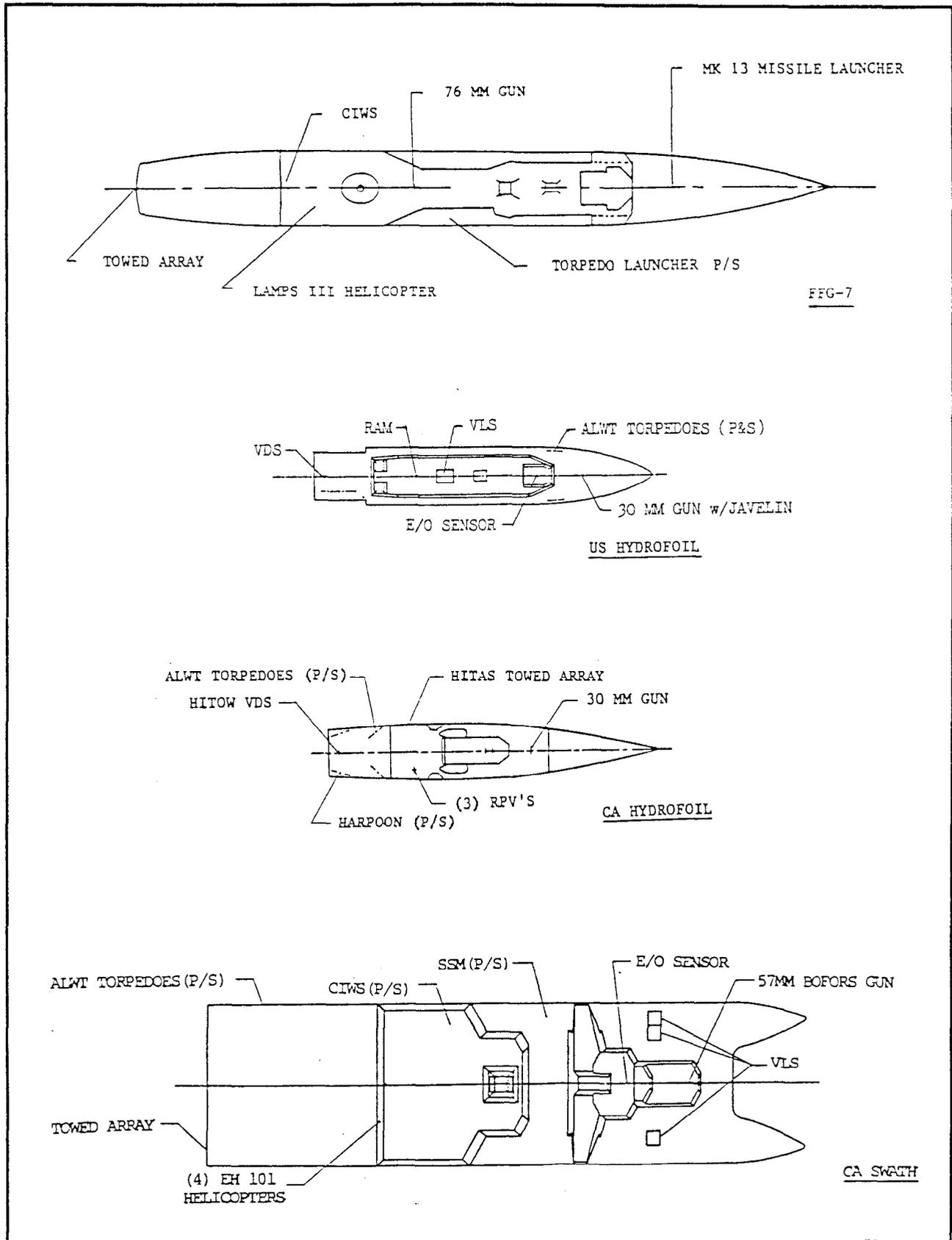
Figure 3.2.6-1. Combat Systems Arrangments Plan View (Sheet 2 of 2)
