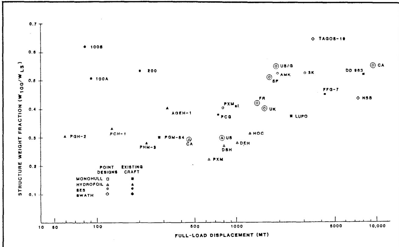
Figure 3.3.18-3. Structure Weight Fraction
