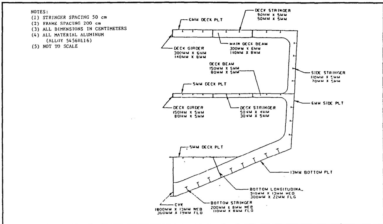
Figure 3.3.3-6. Hydrofoil Midship Section
