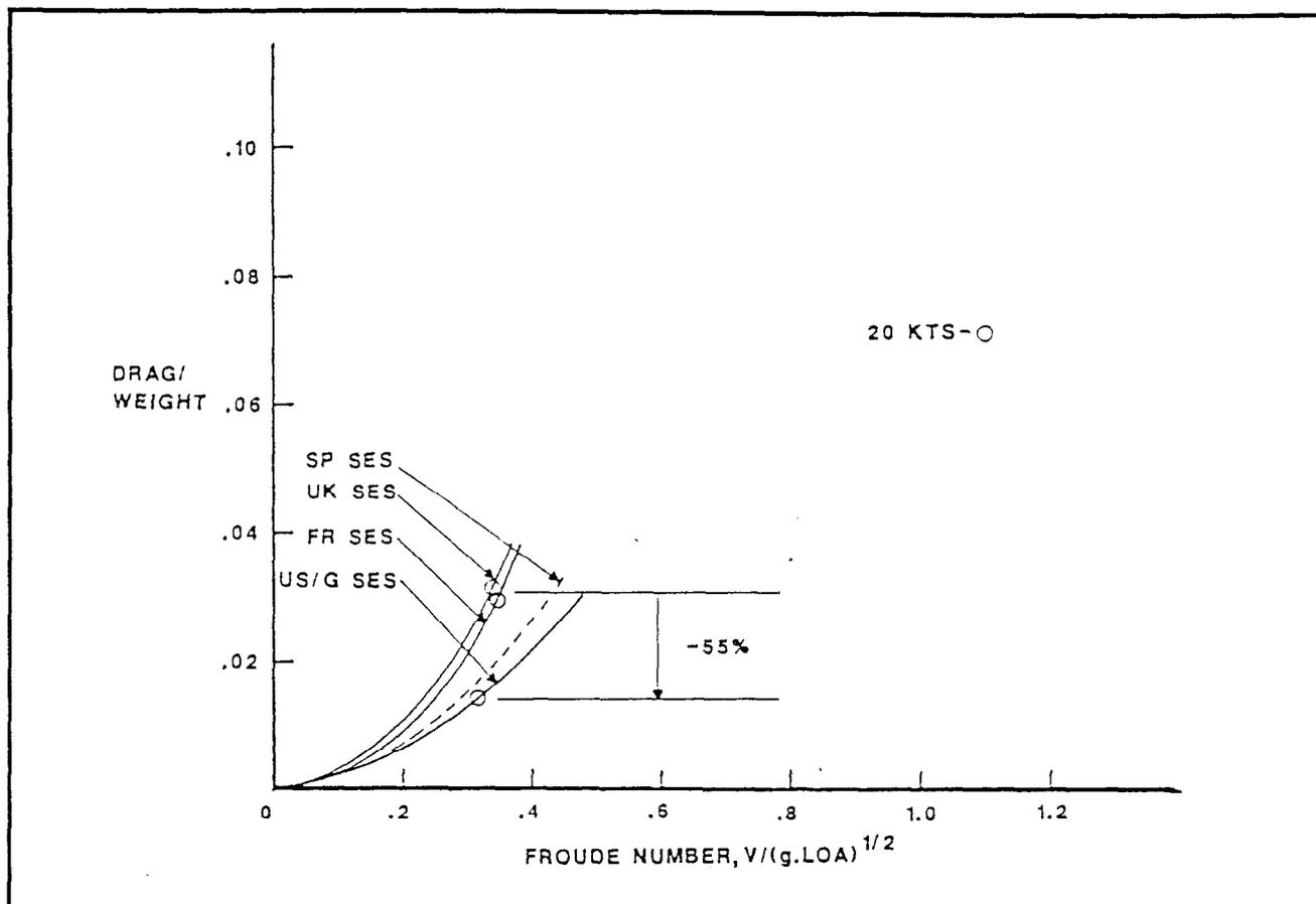
Figure 3.3.5-11. Comparison of SES Off-Cushion Drag in Sea-State 0.
