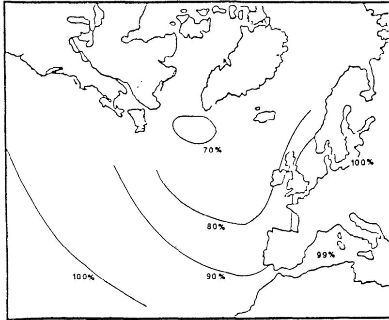
Figure 3.2.3-41. Operability Contour, Canadian Hydrofoil, 45 Knots, Ride-Control, Foilborne, Winter (Ship Operability)
