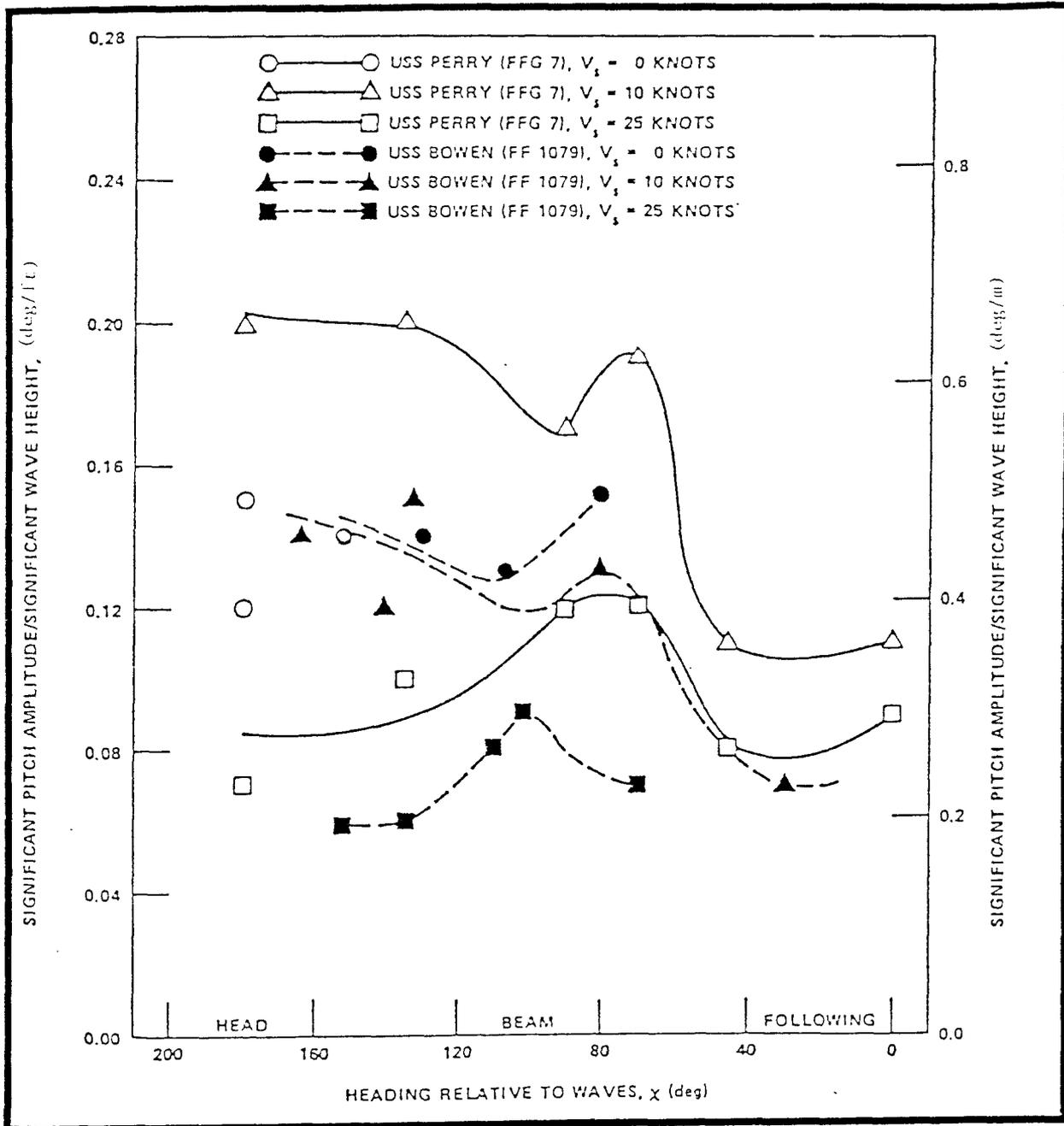
Figure 3.2.3-18. Significant Pitch Amplitude Per Unit Significant Wave Height Versus Heading Relative to Waves from the Trials Conducted on the USS PERRY (FFG-7) and the USS BOWEN (FF 1079) at Ship Speeds of 0, 10 and 25 Knots (Reference 17)
