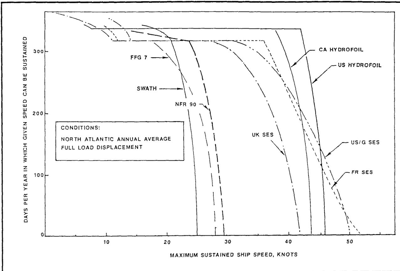
Figure 3.2.1-12. Days Per Year Versus Maximum Sustained Speed for NATO ANVs
