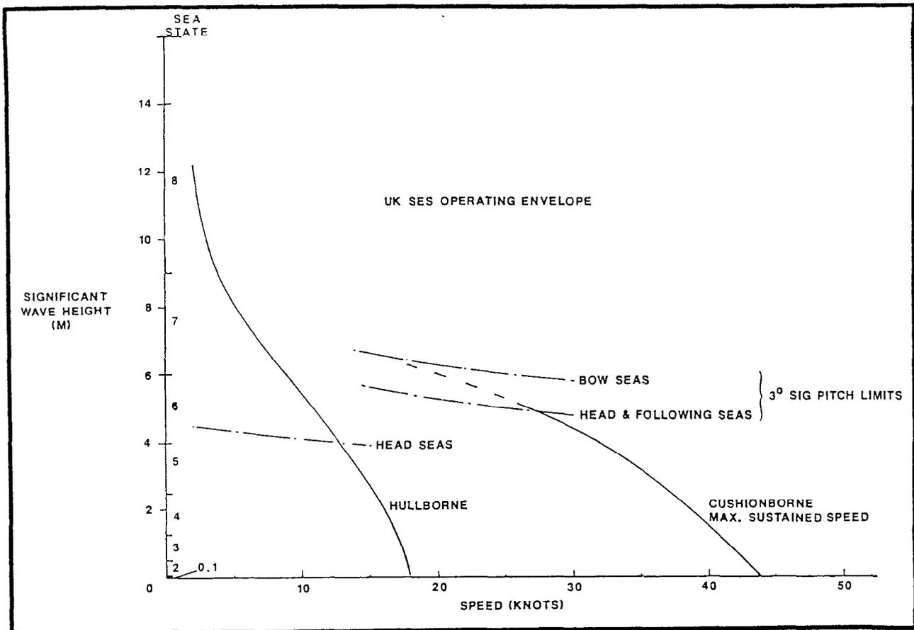
Figure 3.2.1-4. Maximum Sustained Speed Versus Sea State - UK SES
