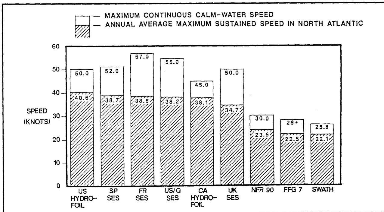
Figure 3.2.1-13. Comparison of Speed Capability
