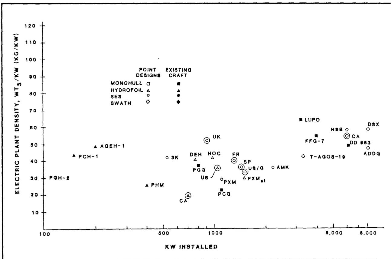
Figure 3.3.18-5. Electric Plant Weight Per KW
