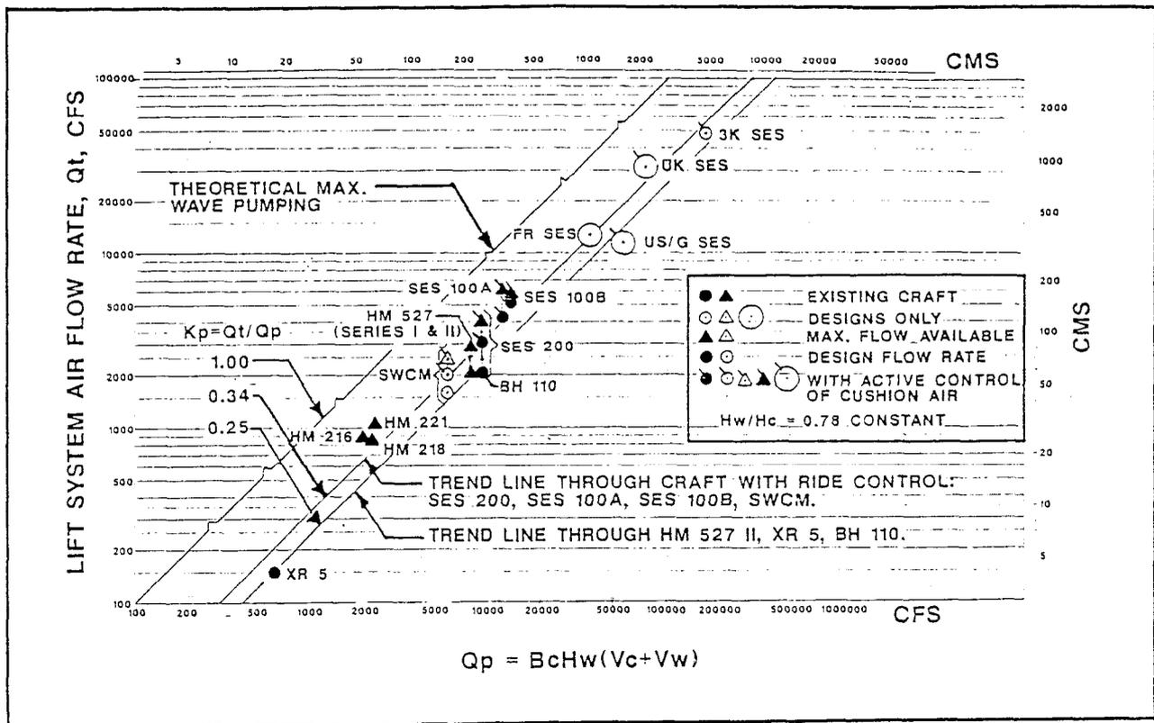
Figure 3.3.7-2. SES Cushion Air Flow Rate Trends Relative to Wave Height, Speed and Cushion Beam
