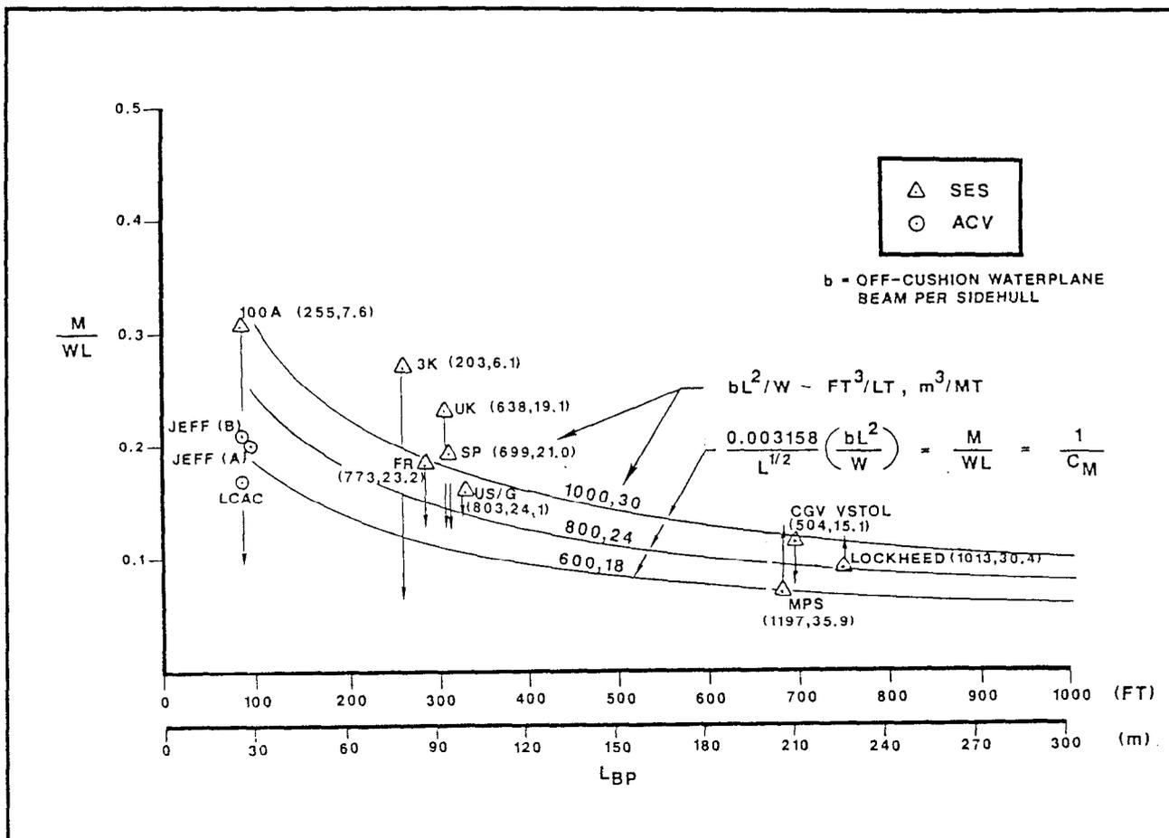
Figure 3.3.3-1. Comparison of Longitudinal Bending Moments Used in Prior SES/ACV Designs
