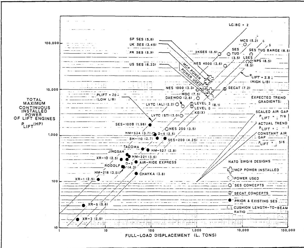
Figure 3.3.7-1. Variation of Installed Lift Power with Displacement for Prior, Existing and Conceptual SES With Non-Integrated Lift Systems.
