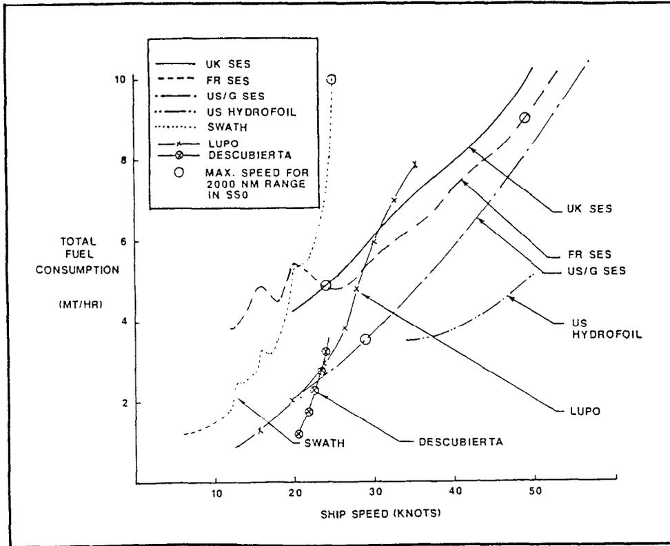
Figure 3.2.2-3. Fuel Consumption versus Ship Speed in the High-Speed, Cushion or Foilborne Mode in Sea State 0
