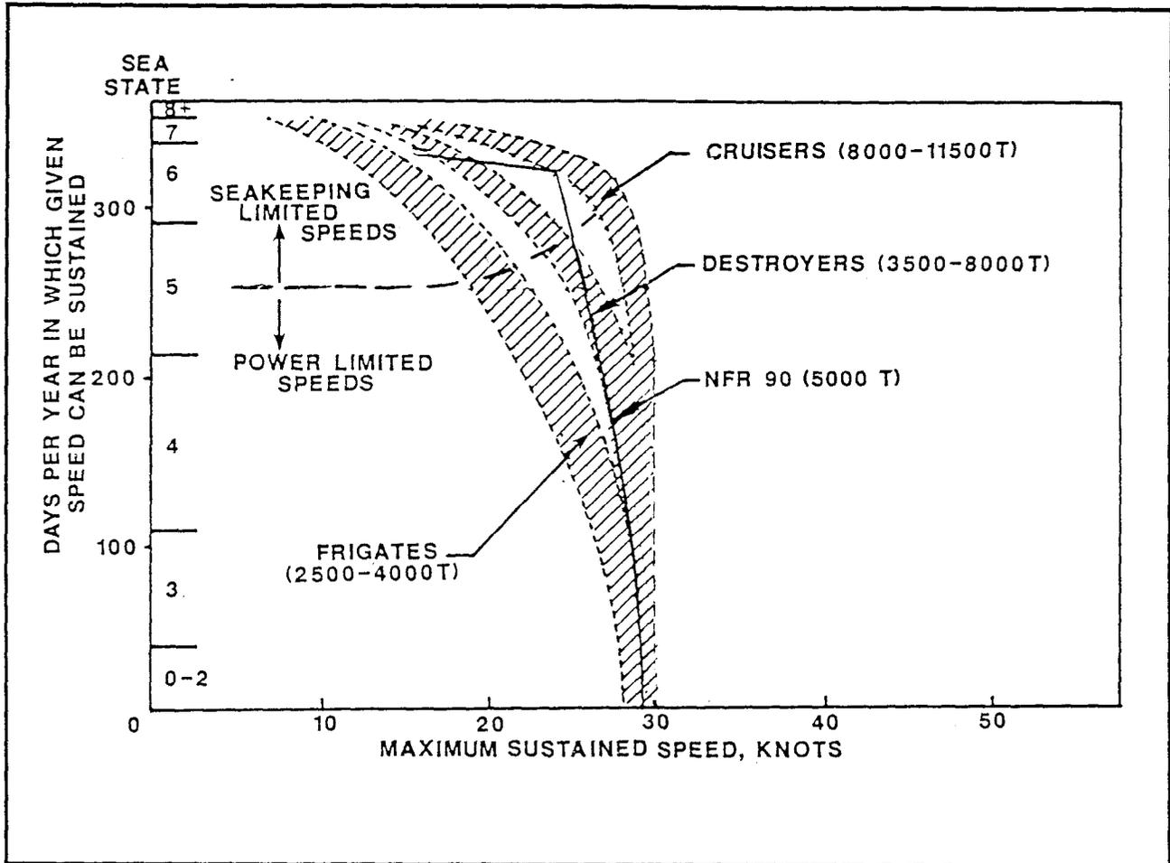
Figure 3.1.2-4. Sustained Speed Capability of Naval Ships (Reference 4)
