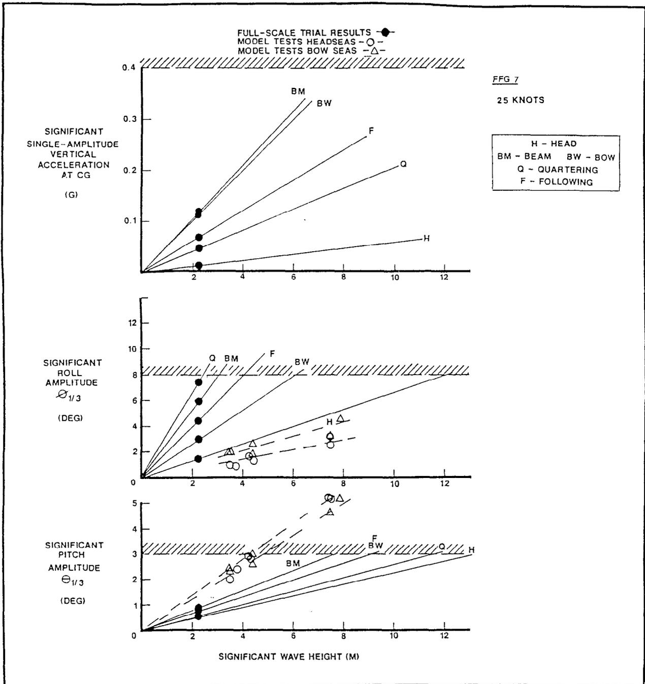
Figure 3.2.3-21. Predicted Variation of Motions and Accelerations With Significant Wave Height for FFG-7 at 25 Knots
