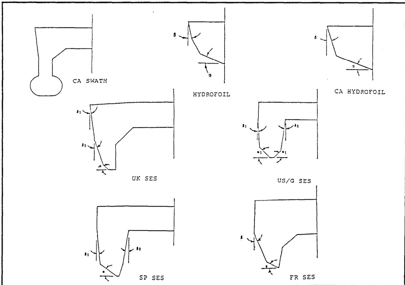
Figure 3.3.2-1. Hullforms
