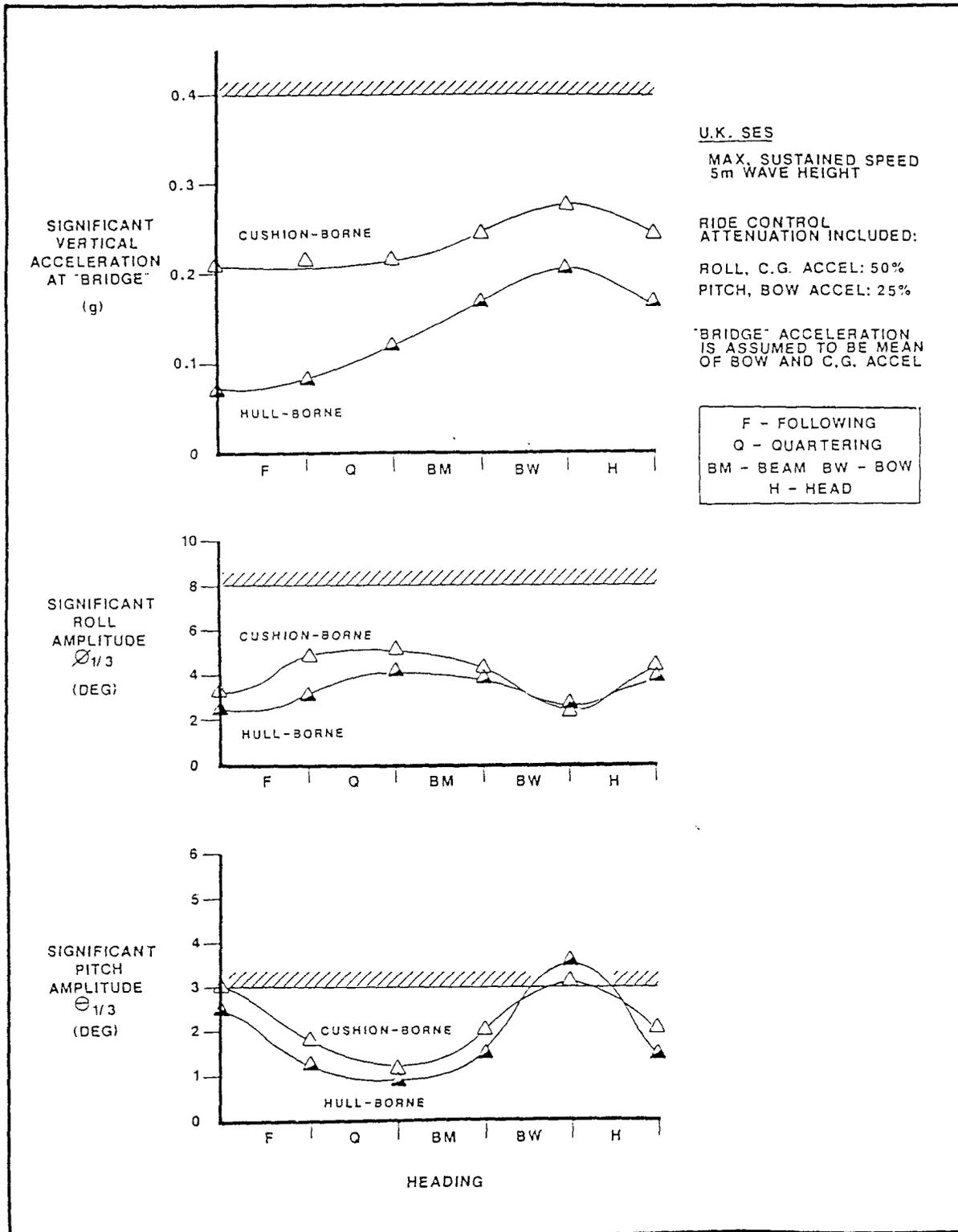
Figure 3.2.3-8. Predicted Variation in Motions and Accelerations With Heading Angle; UK SES at Maximum Sustained Speed in Waves With 5 Meter Significant Wave Height
