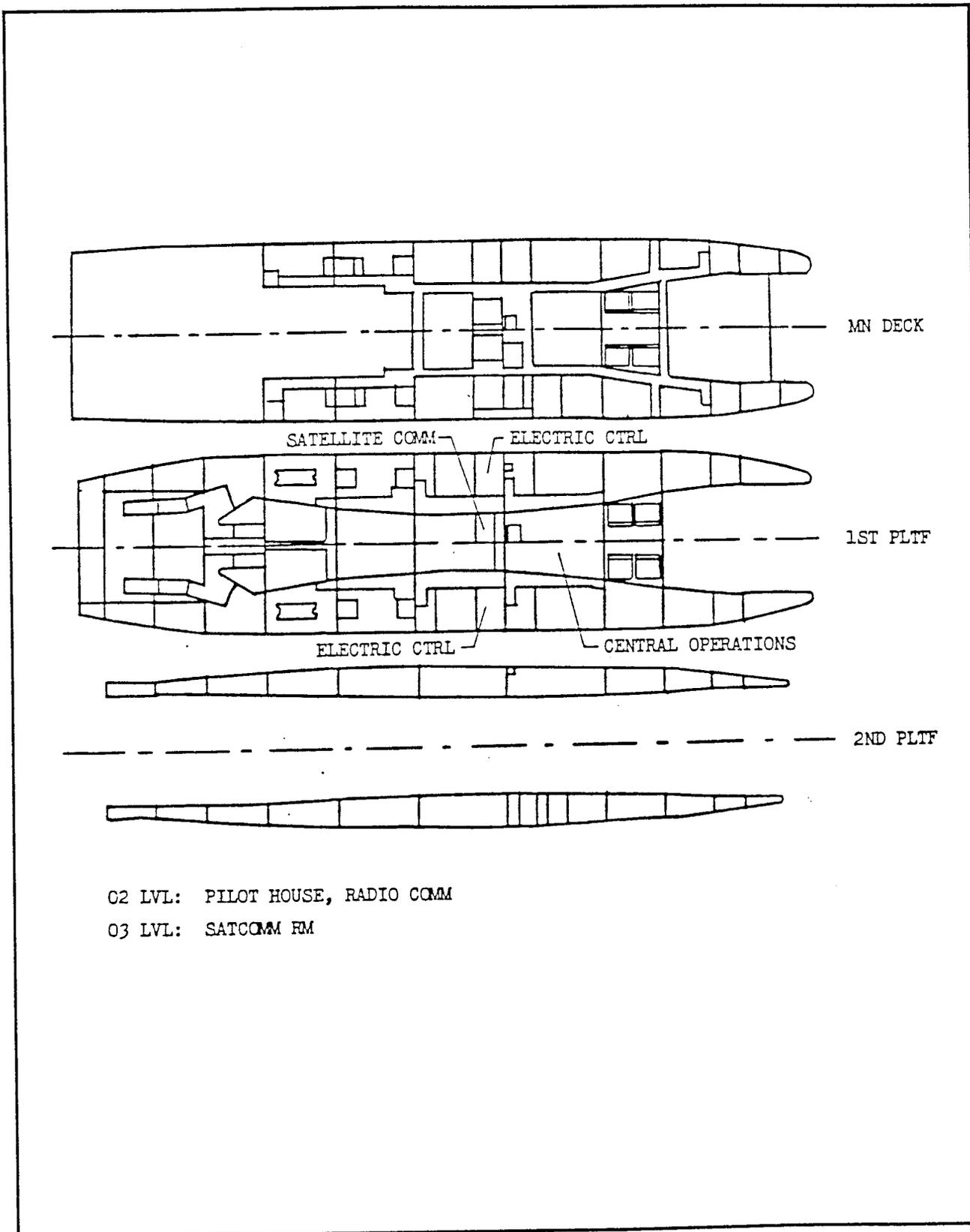
Figure 3.2.8.7-3. FR SES C<sup>3</sup>I Space Arrangement (Sheet 1 of 2)
