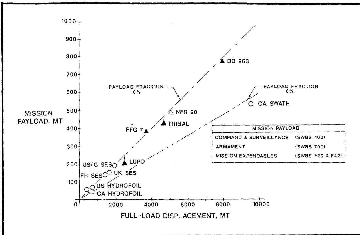
Figure 3.1.2-12. Comparison of Mission Payload
