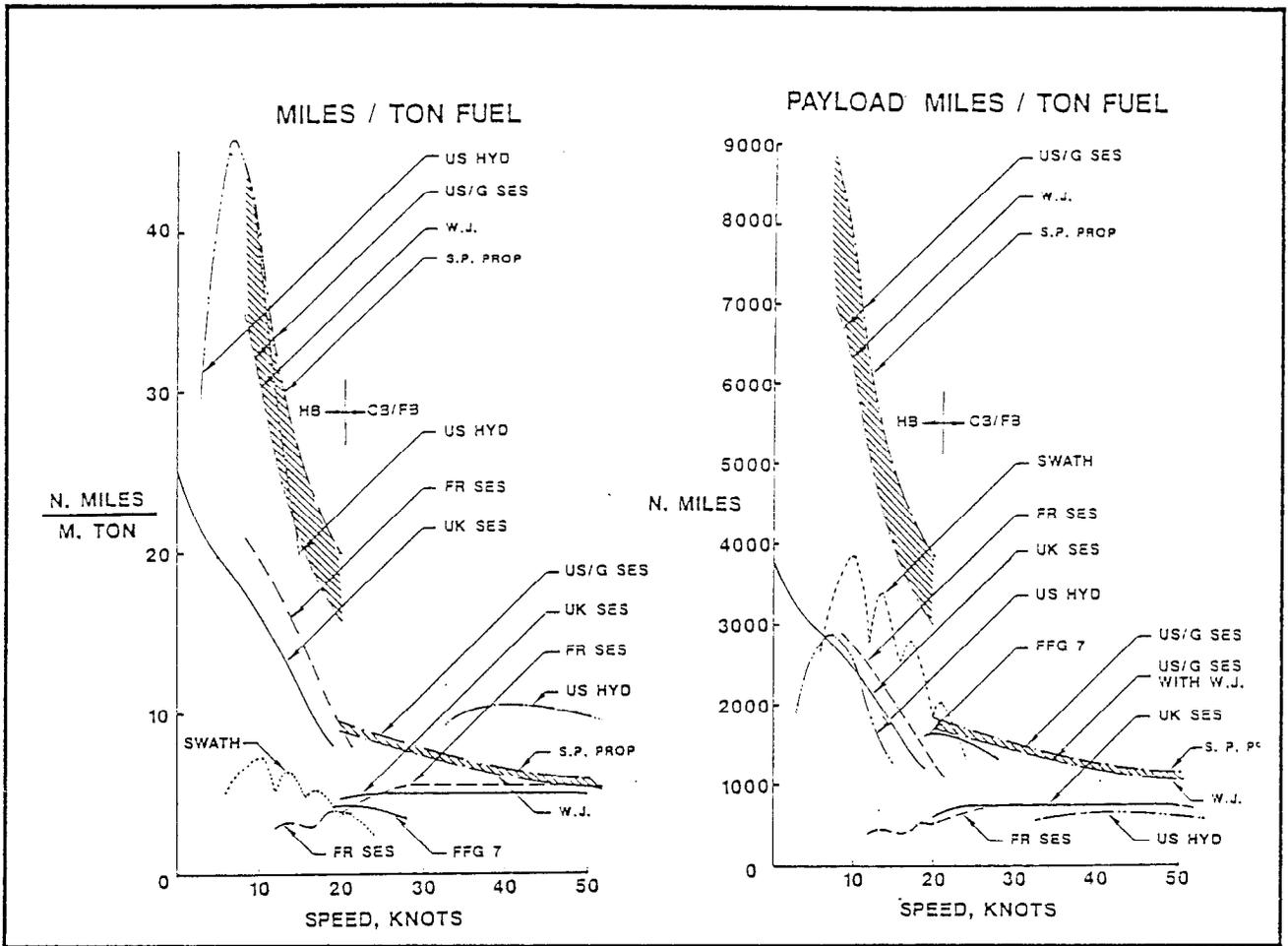
Figure 3.2.2-5. Comparison of Range Per Unit of Fuel
