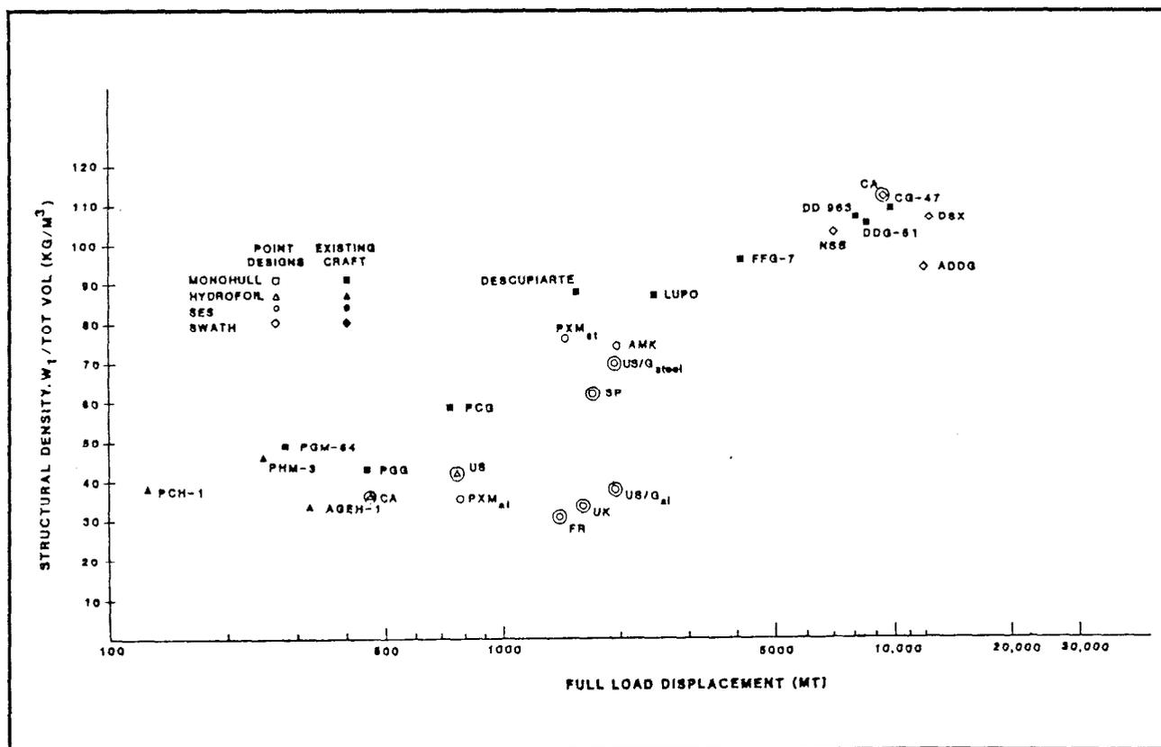
Figure 3.3.18-2. Structural Density
