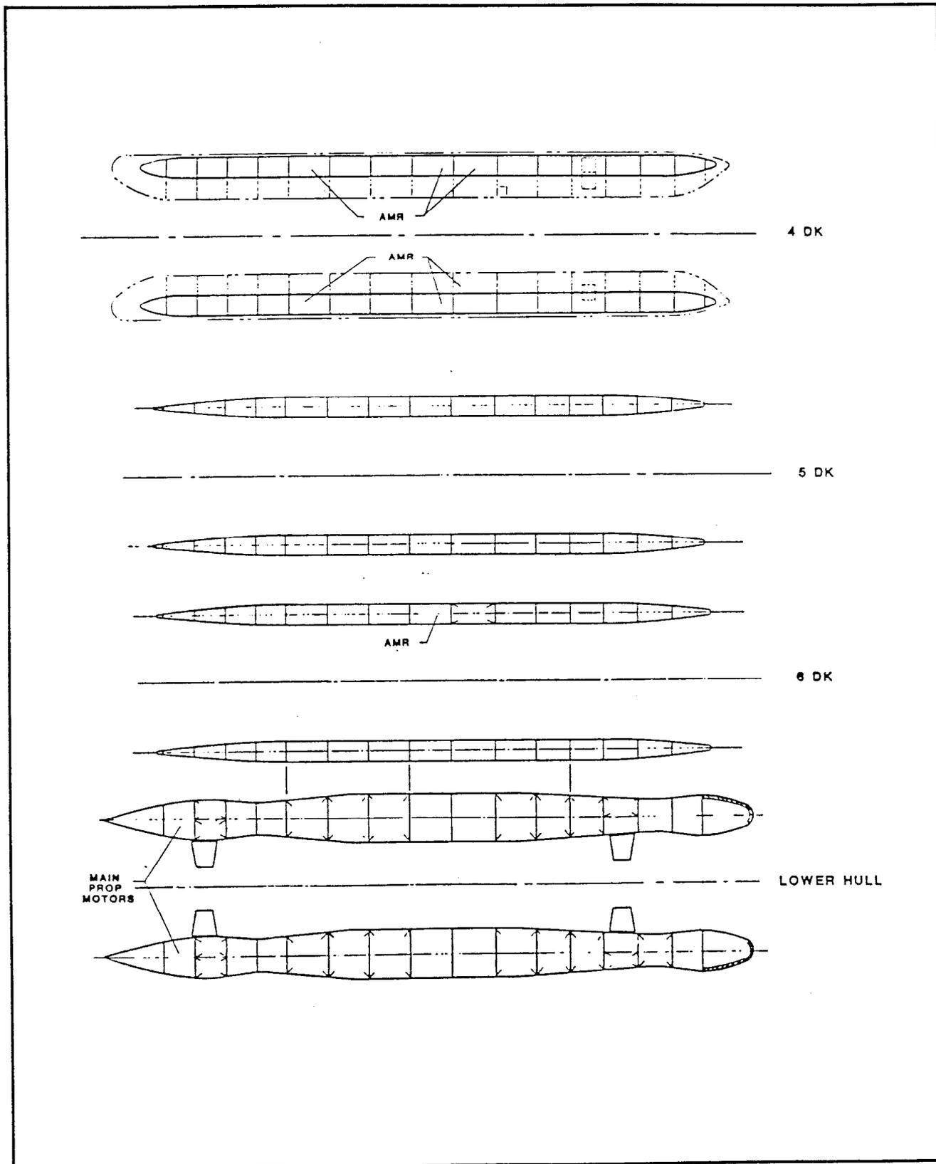
Figure 3.2.8.7-6. SWATH Machinery Arrangements (Sheet 4 of 4)
