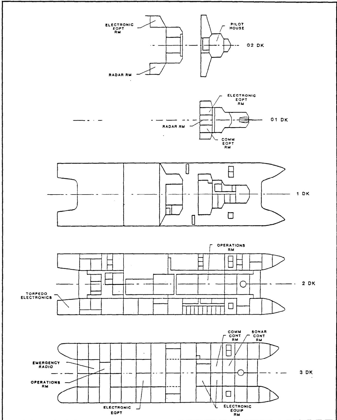
Figure 3.2.8.7-6. SWATH C<sup>3</sup>I Space Arrangement (Sheet 1 of 4)
