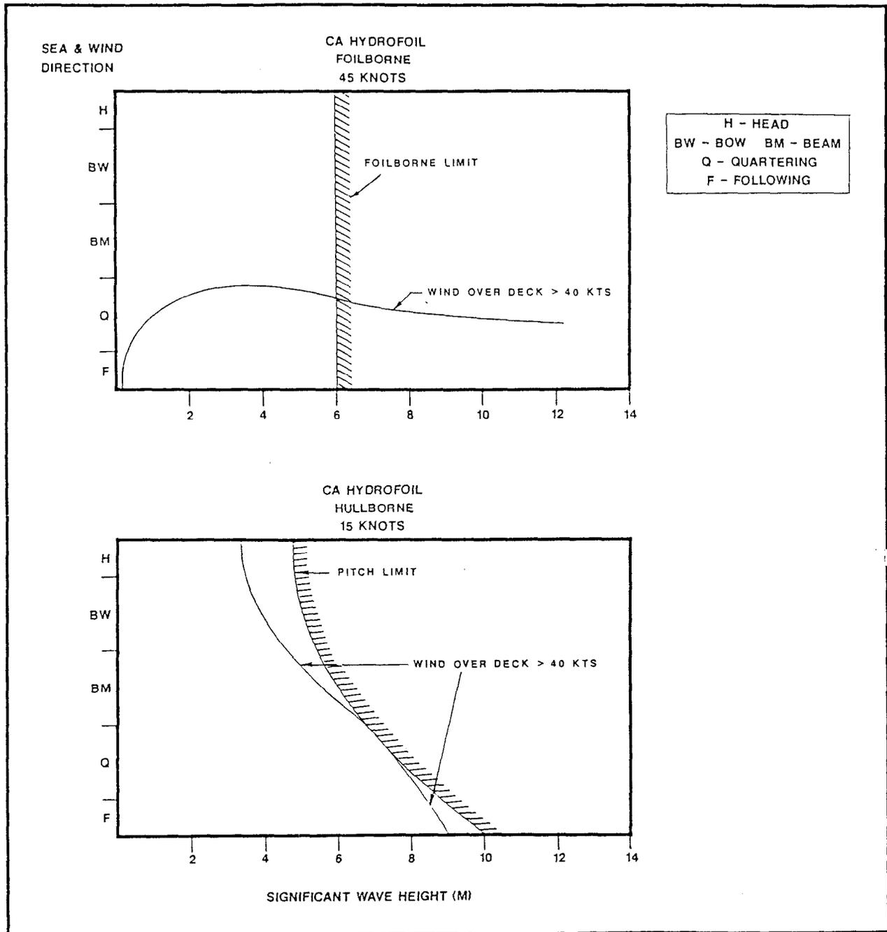
Figure 3.2.3-27. CA Hydrofoil Seakeeping Limits
