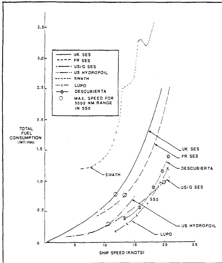
Figure 3.2.2-1. Fuel Consumption Versus Ship Speed - Low-Speed, Hullborne Mode in Sea State 0
