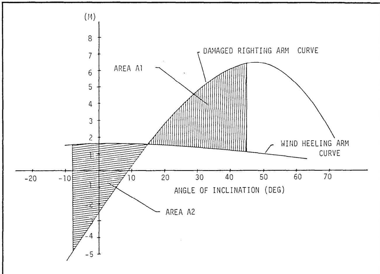
Figure 3.3.21-2. Damage Stability Curve
