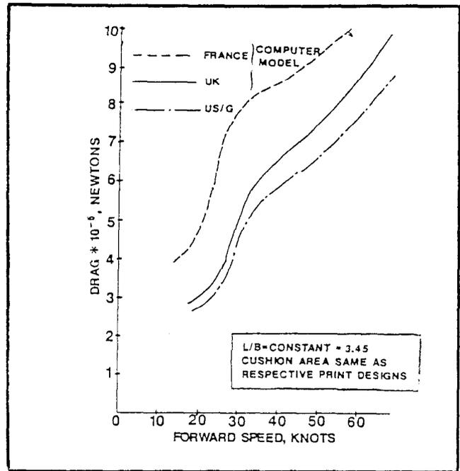
Figure 3.3.5-7. Comparison of Predicted Drag of Low L/B Version of SES Point Designs at Comparable Weights
