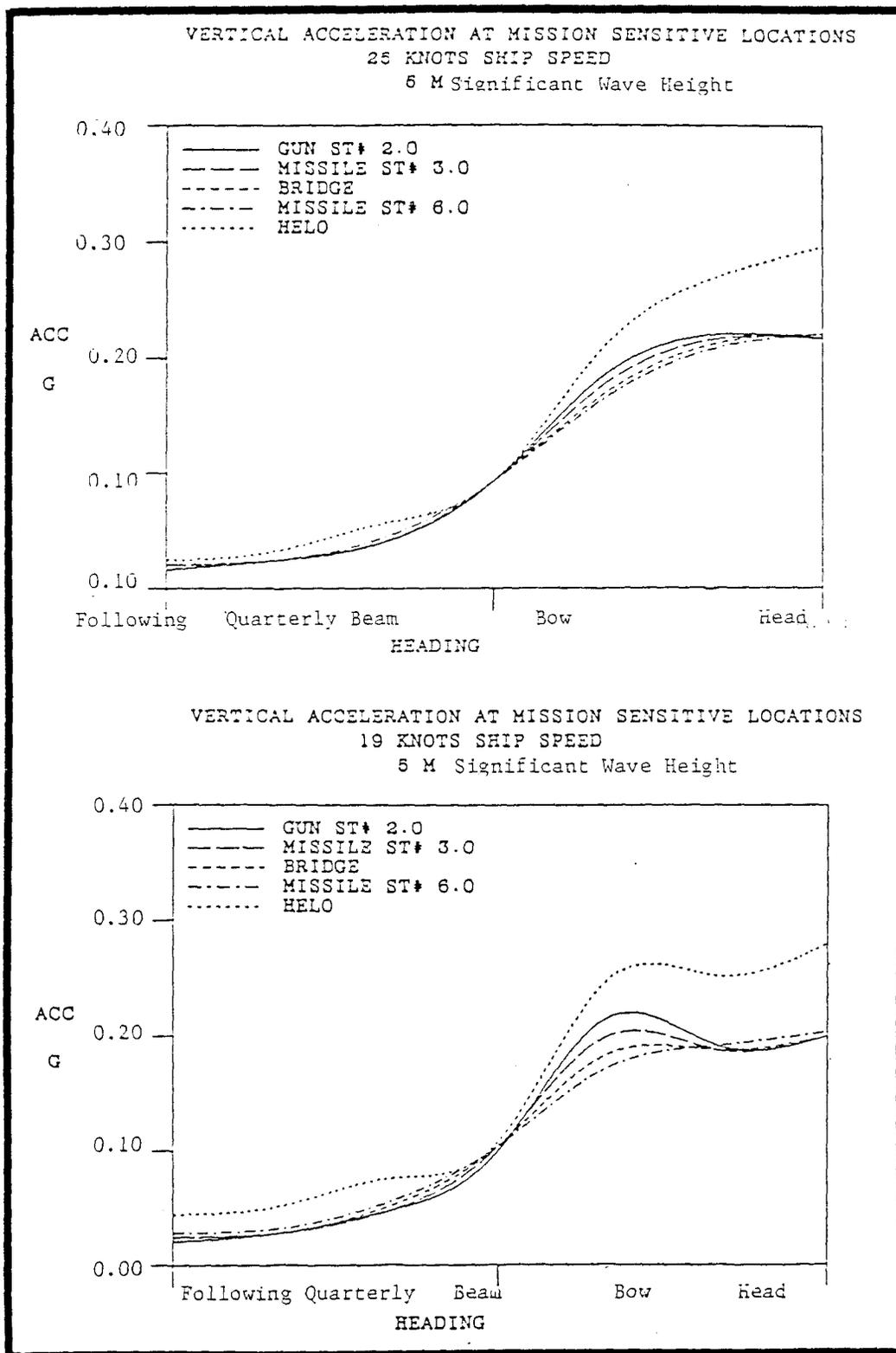
Figure 3.2.3-17. SWATH Vertical Acceleration at Worst Modal Period of Reference 15
