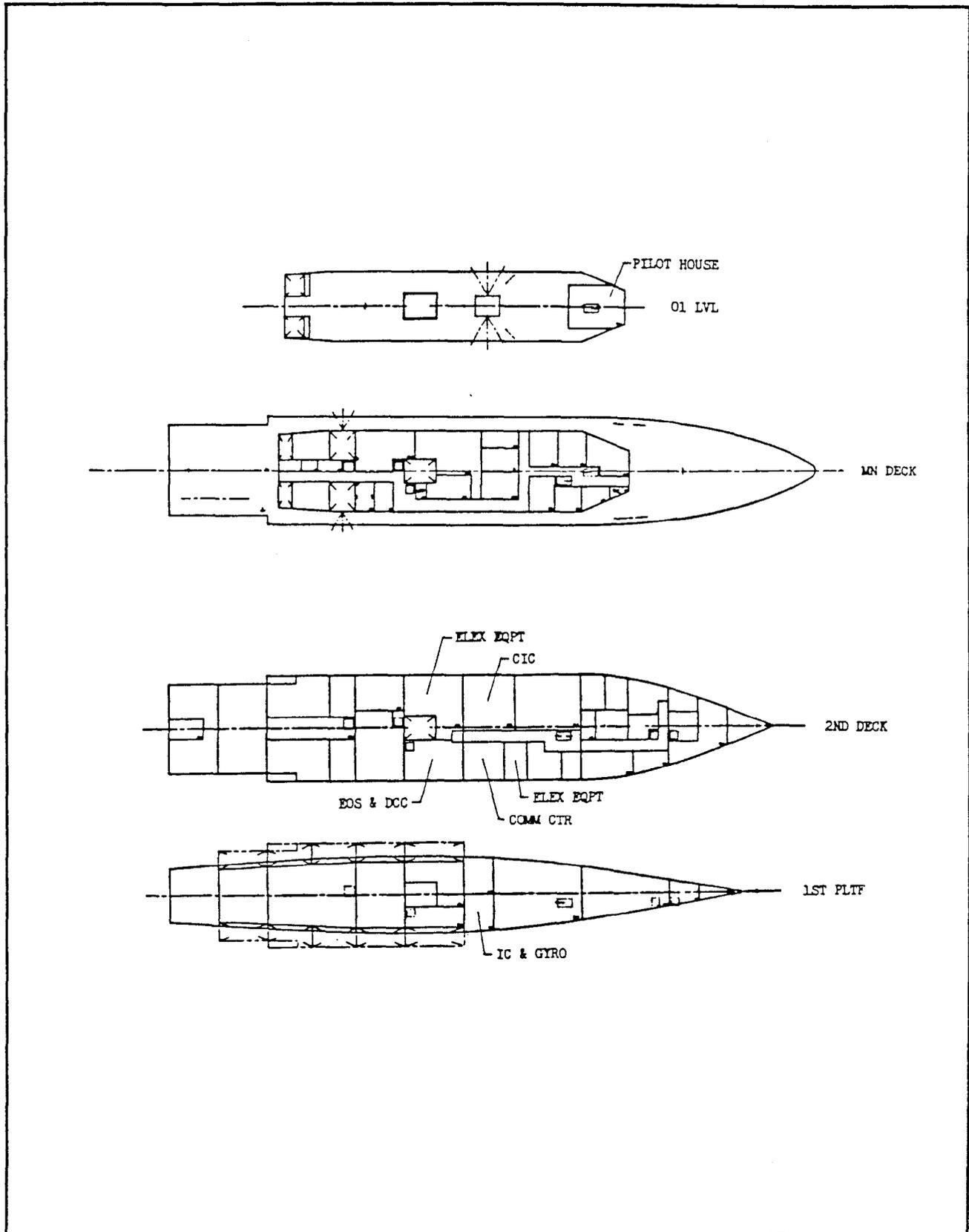
Figure 3.2.8.7-4. US Hydrofoil C<sup>3</sup>I Space Arrangement (Sheet 1 of 2)
