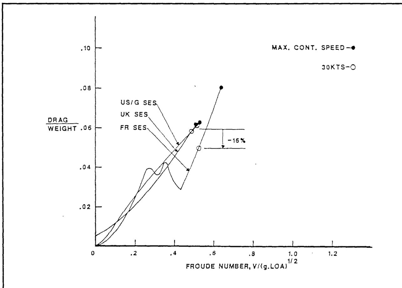
Figure 3.3.5-10. Comparison of SES On-Cushion Drag in Sea-State 6.
