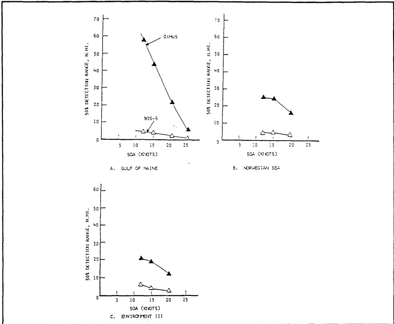
Figure 3.2.1-1. Effects of Changes in Speed on Detection Ranges. Results Relate to Two Different Sonars (DIMUS, BQS-6) for Three Different Acoustic Environments.
