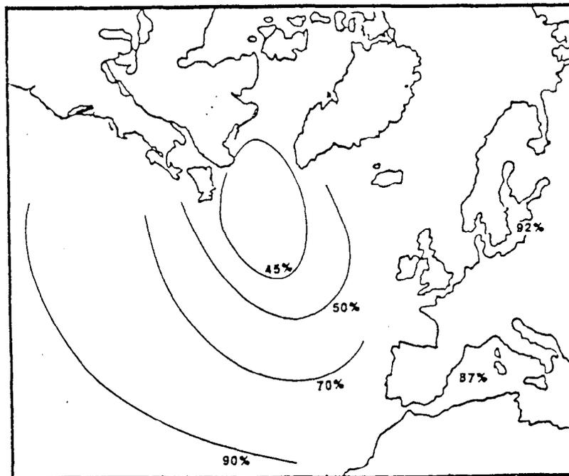
Figure 3.2.3-44. Operability Contour, FFG-7, 25 Knots, Active Fin Stabilizers, Winter (Ship Operability)
