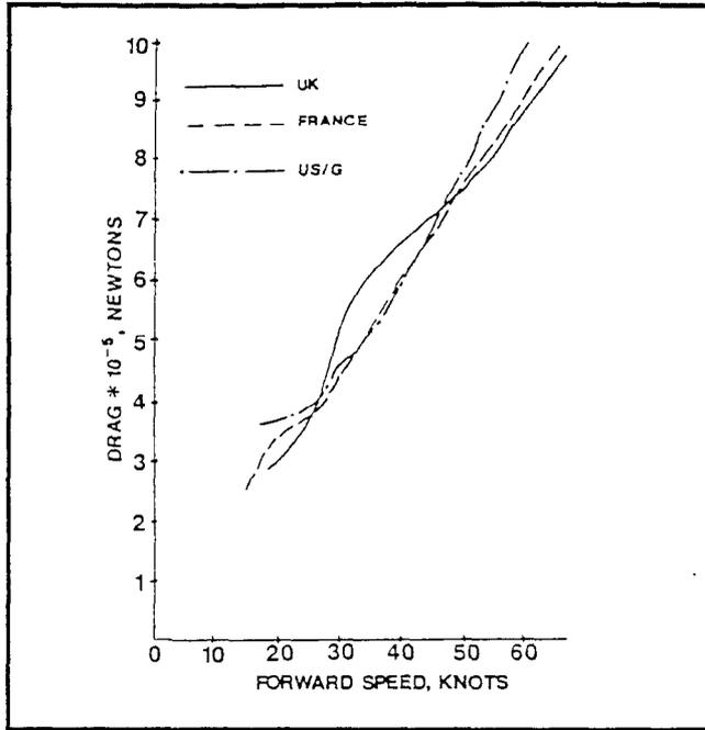
Figure 3.3.5-6. Comparison of Predicted Drag of SES Point Designs
