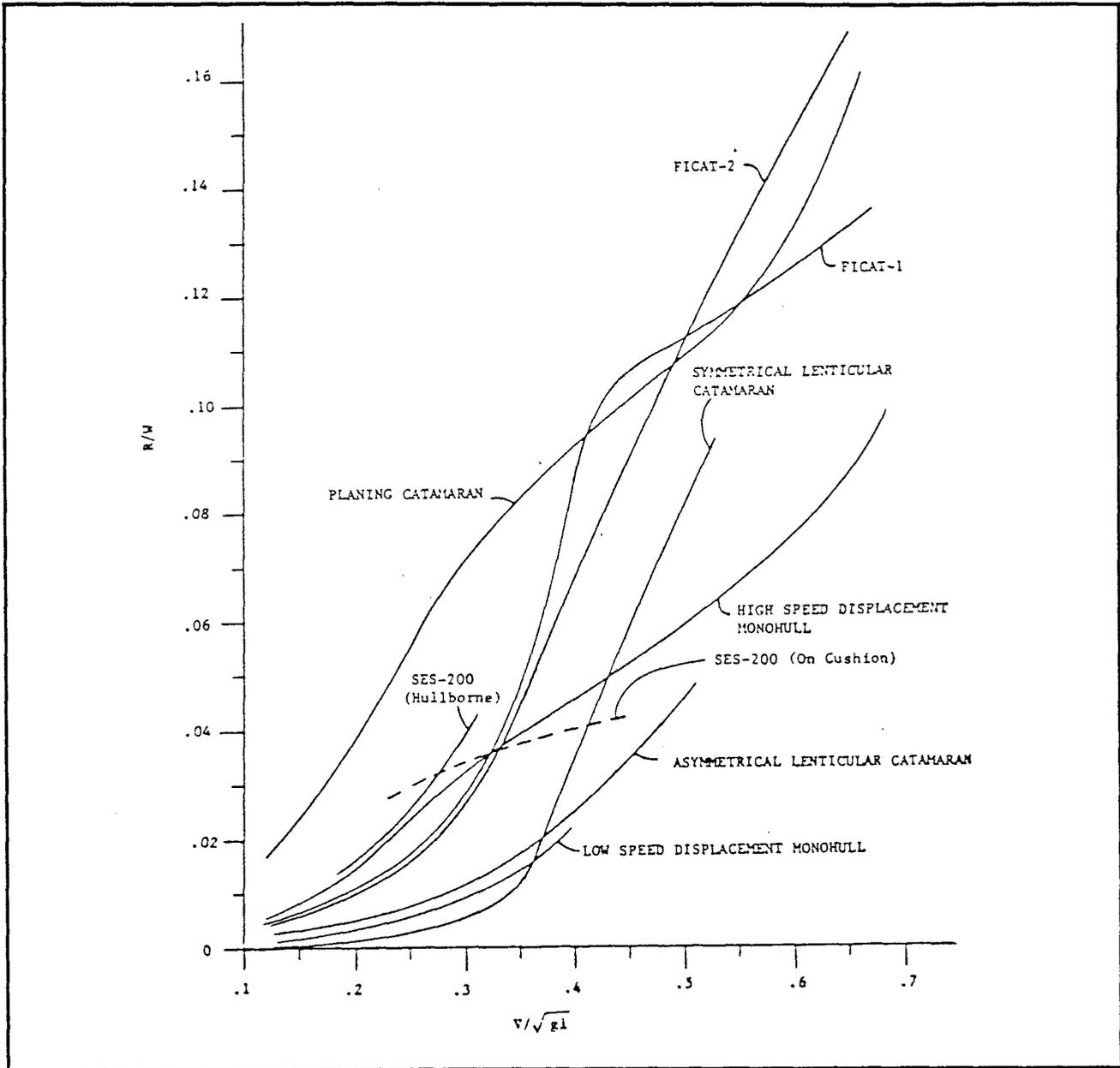
Figure 3.3.5-13. Specific Resistance of Comparative Hullforms in Calm Water
