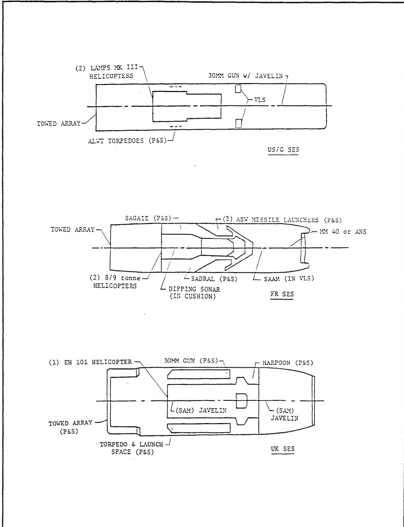
Figure 3.2.6-1. Combat Systems Arrangements Plan View (Sheet 1 of 2)
