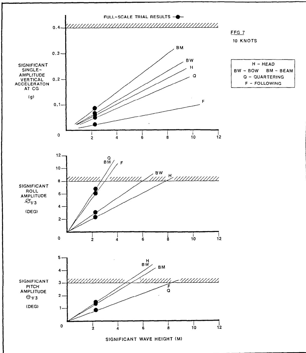
Figure 3.2.3-22. Predicted Variation of Motions and Accelerations With Significant Wave Height for FFG-7 at 10 Knots
