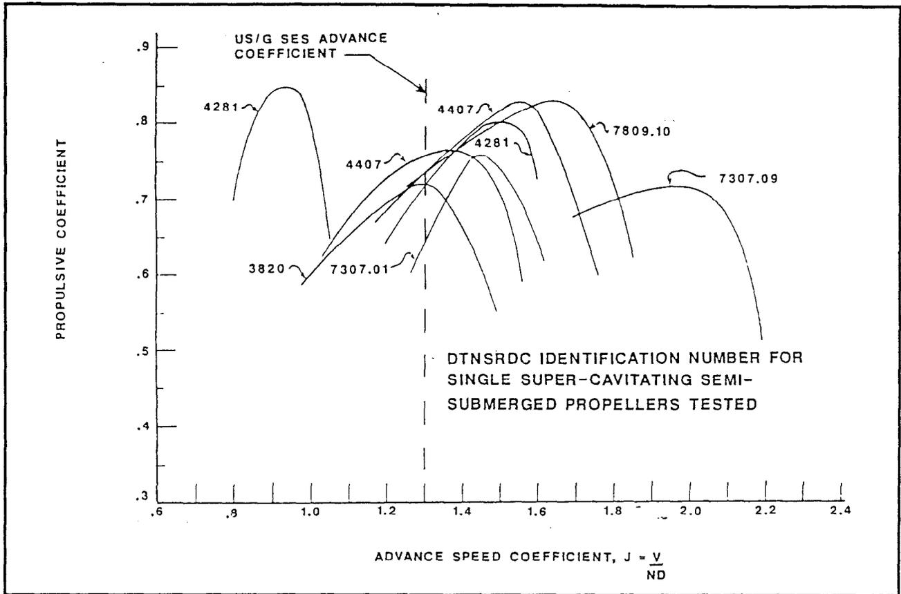
Figure 3.3.6.3-1. U.S. Surface Piercing Supercavitating Propeller Model Tests. (The above curves are representative of numerous DTNSRDC propeller tests run at various speed coefficients, depth of submergence, shaft inclination angle and propeller pitch.)
