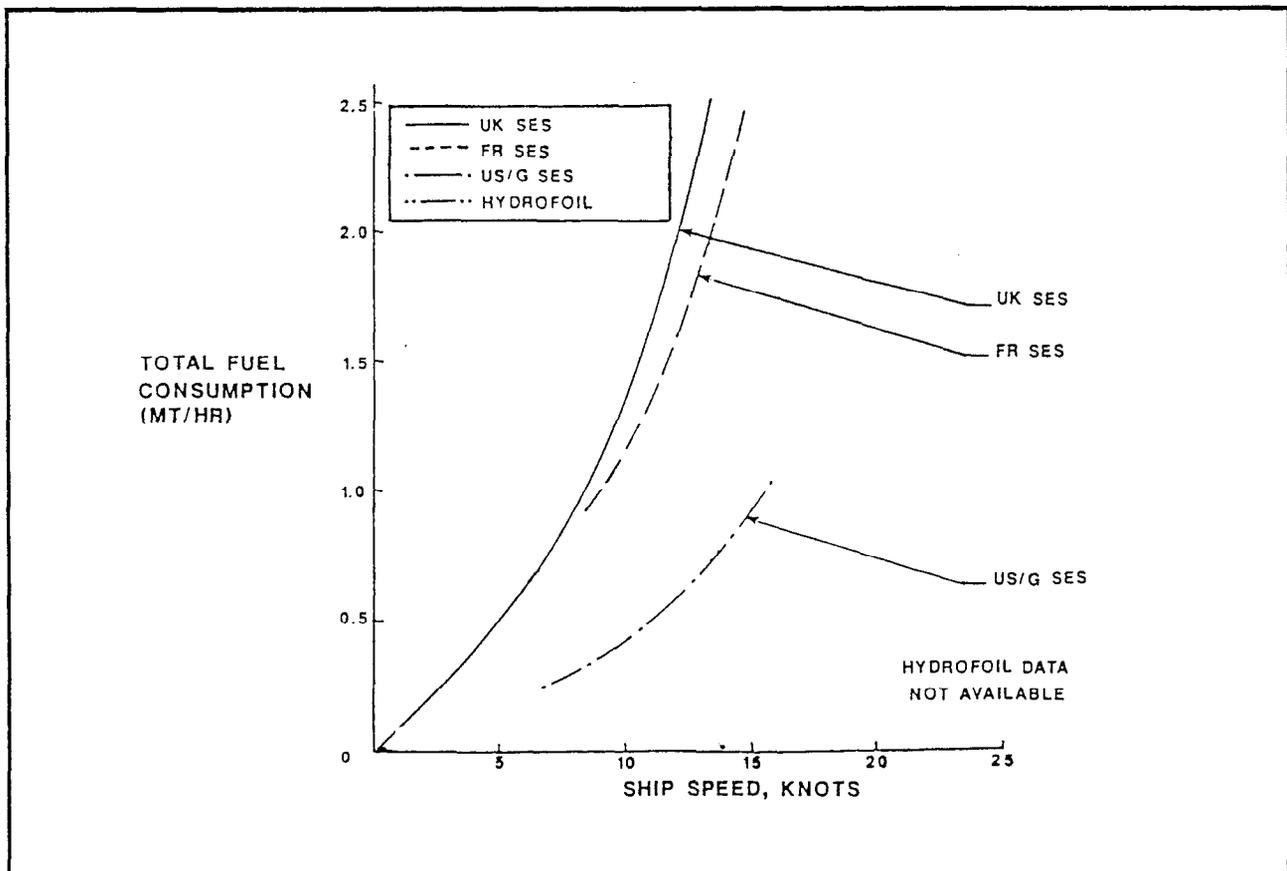
Figure 3.2.2-2. Fuel Consumption Versus Ship Speed - Low-Speed, Hullborne Mode in Sea State 6
