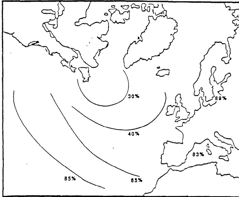
Figure 3.2.3-45. Operability Contour, FFG-7, 10 Knots, Winter (Ship Operability)
