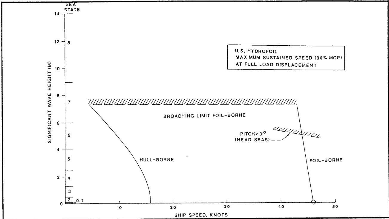
Figure 3.2.1-7. Maximum Sustained Speed Versus Sea State - U.S. Hydrofoil
