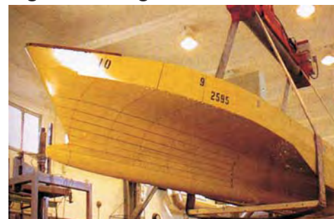
An extensive series of tank tests were carried out at Marintek and MARIN
