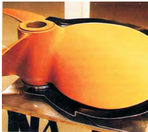
Propeller Blade During Encapsulation Process.
