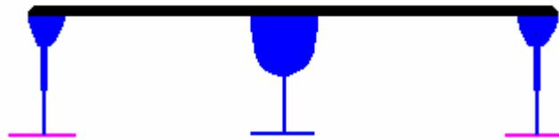
Submerged, variable angle foils
